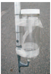
Sampling bottle attached to pole as found in the "Stormwater Sampling for the Vermont Multi - Sector General Permit: A Guide for Industrial Facilities"
