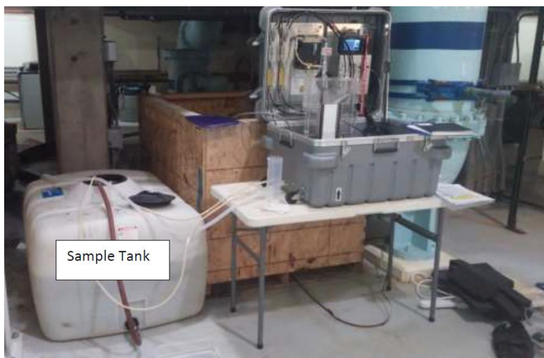
Figure 4.4 – Photo of Bench-Scale Ceramic Membrane Unit (Meiden)
