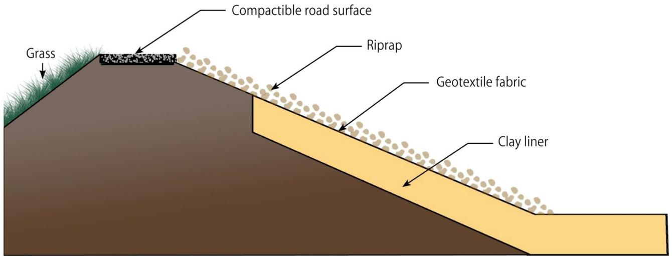
NOTE: See design criteria for specifications for riprap, clay and synthetic liner.
