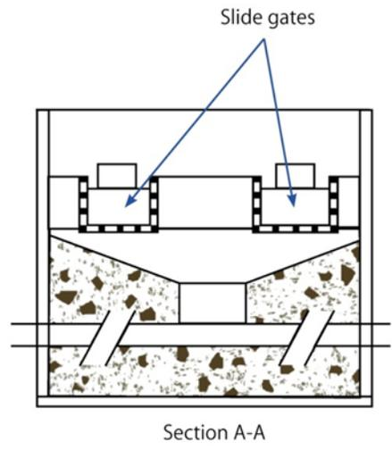
Figure 7A: **Telescoping valve**
