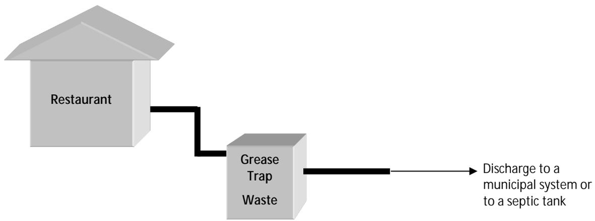
Figure 2. When there is no tank specifically dedicated to collection of greases, fats, and oils, the first septic tank that receives effluent from a restaurant is considered the grease trap.
