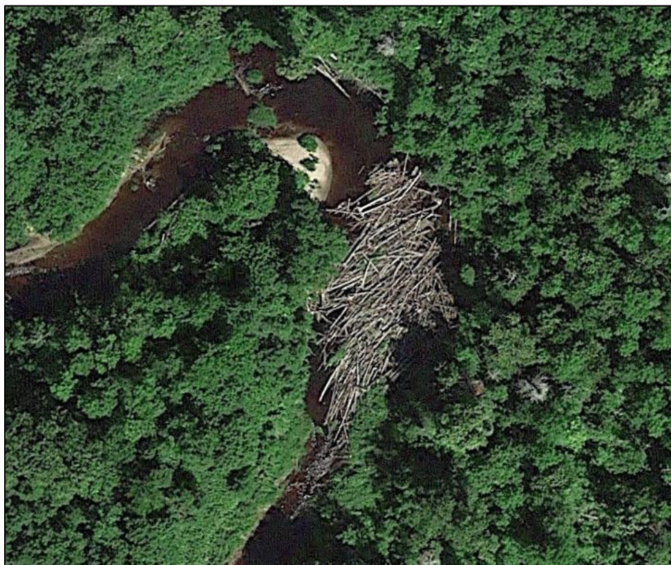
Figure 17. As a consequence of un-naturally fast erosion of stream banks of Caldwell Brook, trees along the channel are undermined and topple into the channel and form log jams. Many log jams were documented in Caldwell Brook. This aerial photo is from 7/18/2016. This logjam is still present in 2023 aerial photos.
