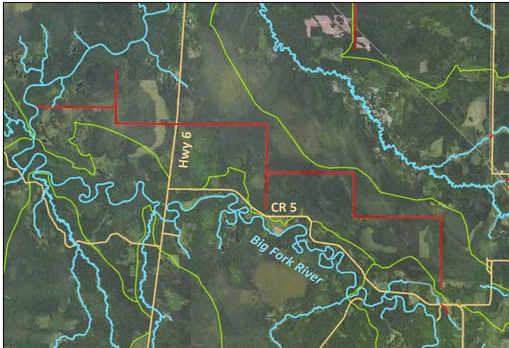
Figure 5. The peatland ditch system between the Big Fork River and Reilly Brook, which drains to the Big Fork River.
