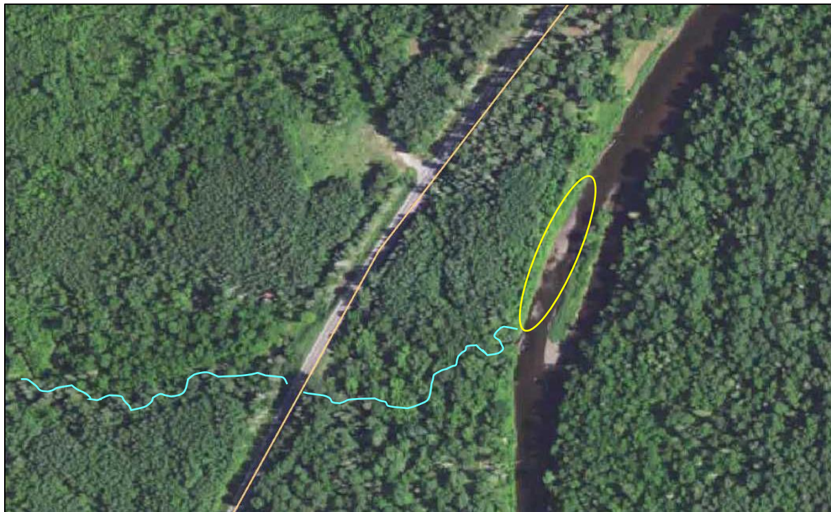
Figure 35. Deposited sediment (circled in yellow) can be seen in the Big Fork River immediately downstream of where the short tributary from Figure 23 enters the river.
