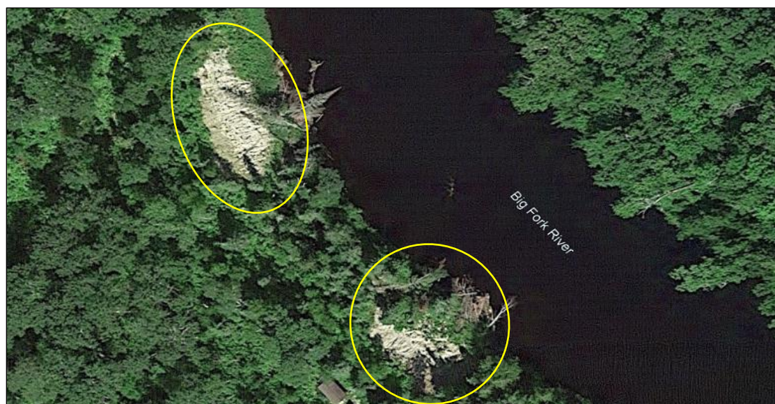
Figure 22. Two nearby bank erosion locations, about 3.6 miles downstream of Big Falls. Collapsed dead trees can be seen at the base of both bank slides.
