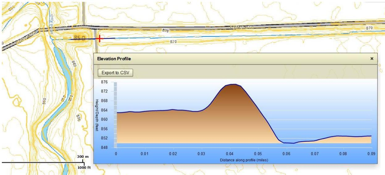
Figure 4.2.3. Elevation profile of the high gradient culvert on County Ditch 11 (IWI, 2017).
