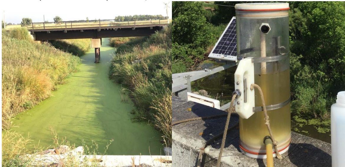
Figure 3. Images of eutrophication-related conditions, including excessive filamentous algae and duckweed at Site S003-274 (State Hwy 55 crossing) along Judicial Ditch 2 (AUID 09020101-559) on September 20, 2023 (left) and sestonic algae in the Van Dorn water sampler at Site S004-176 (490th St crossing) along the Rabbit River, South Fork (AUID 09020101-512) on June 10, 2021.
