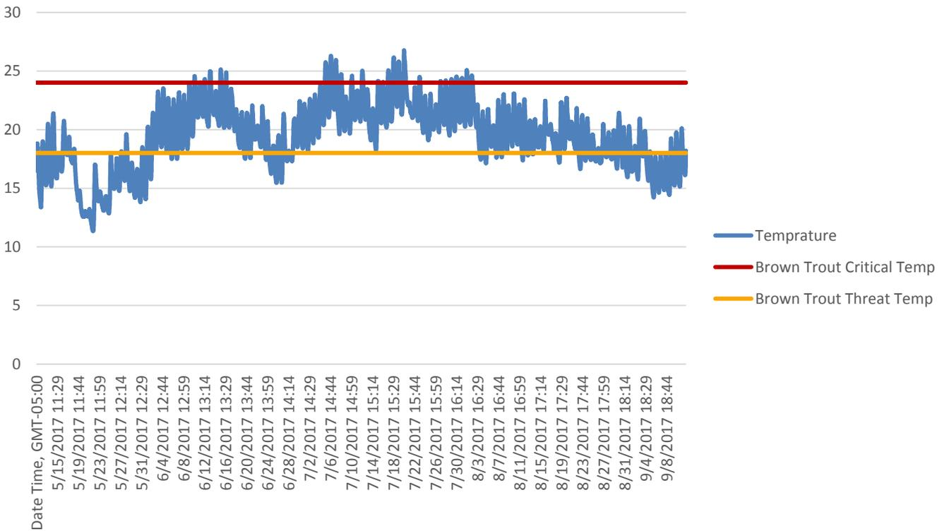
**Figure 18. Continuous temperature data collected longitudinally on the South Fork Crooked Creek in 2017. One station was located upstream of the R-3 reservoir, one just downstream of the R-3 reservoir discharge point, and one farther downstream at biological station 15LM033. This comparison was used to assess temperature changes and impacts from the reservoir and coldwater tributary springs just downstream of the R-3 outlet.**
