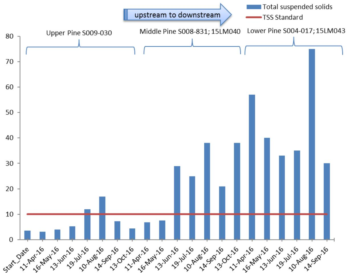
**Figure 10. TSS concentrations (mg/L) from 59 samples taken longitudinally (upstream-left to downstream right) at multiple Pine Creek sites in 2016 and 2017. Stations are organized upstream to downstream, which shows increases in TSS moving downstream in the impaired AUID (S009-031 and S004-017). The red dashed line (10 mg/L) indicates the TSS standard for coldwater streams. S005-076=15LM041, S009-031=15LM040, and S004-017=15LM043**
