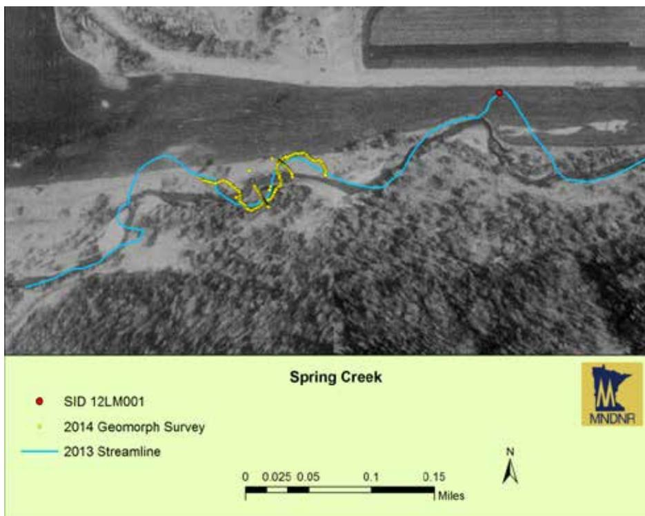
Figure 32. 2013 streamline and 2014 survey overlaying 1991 aerial photo.
