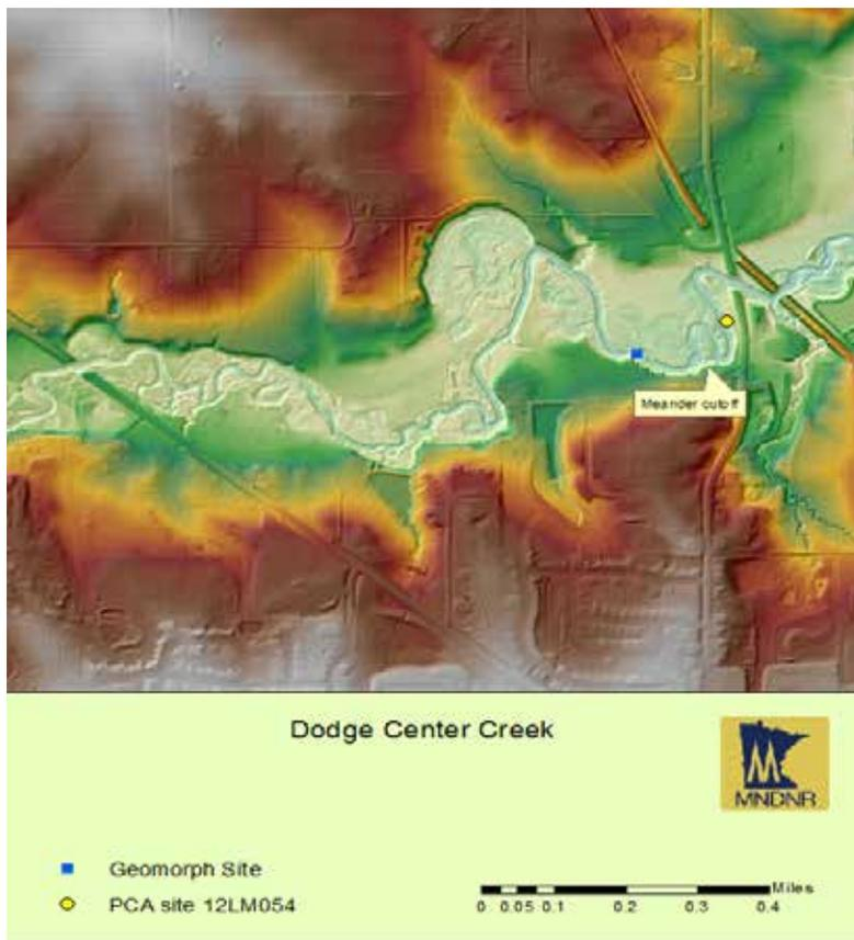
Figure 85. Survey locations and meander cutoff from MNDNR geomorphology survey.
