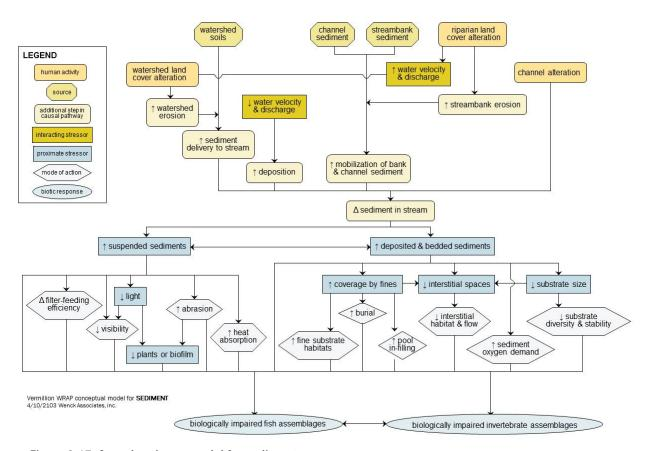
Figure 3-17. Causal pathway model for sediment.
