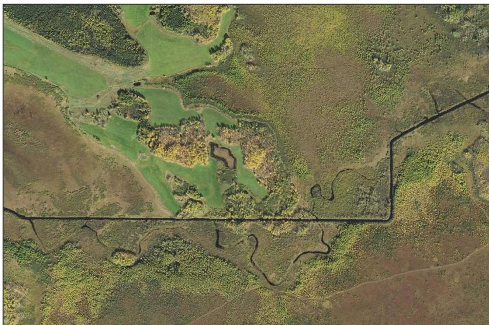
**Figure 12.** Example location where ditch filling could be accomplished to naturalize hydrology (improve storage). This peatland is just east of Kettle Lake, which can be seen at the far left. No stream channel existed in much of this wetland prior to ditching. The extent of the original, natural channels draining the wetland into Kettle Lake are circled in yellow.
