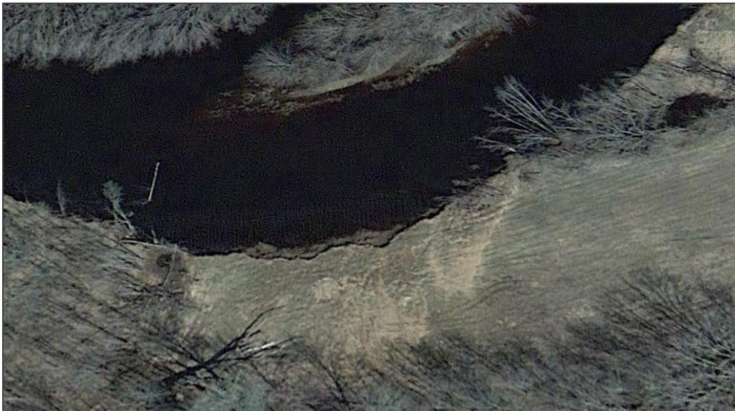
**Figure 43. Bank erosion all along the outside bend where trees have been cleared and replaced with grasses, which have far less capability of providing erosion resistance to the riverbank.**
