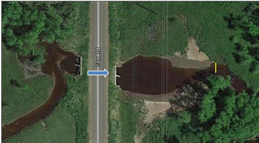
Figure 24. 1939 aerial photo of an eroded pool, still present in 2017. A road crossing existed at the head of the pool, which eliminated the floodplain there, and focused high flows, increasing the erosive force of the water. Arrows point to road, which is visible as a raised grade on recent LiDAR imagery.
