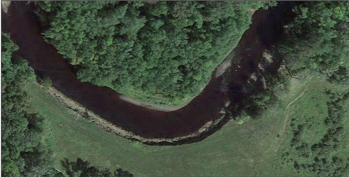
**Figure 42.** Local area of bank erosion where woody bank vegetation has been removed and replaced with grasses.
