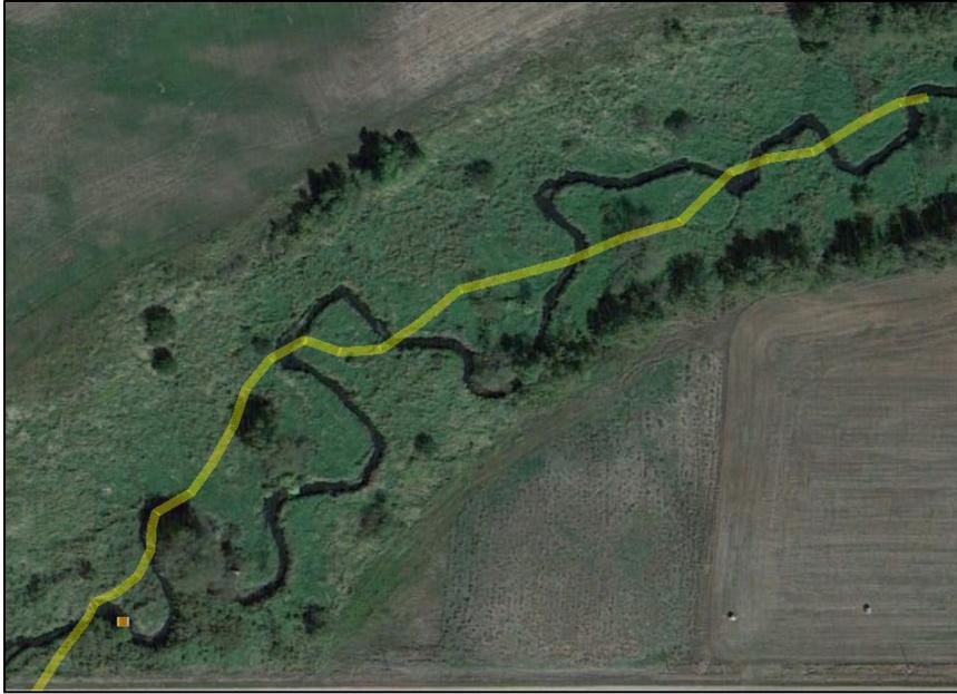
**Figure 8: Biological monitoring site GB-3 stream channel (yellow line – sinuosity of 1.05) superimposed on top of biological monitoring site GB-5 (sinuosity of 1.65).**
