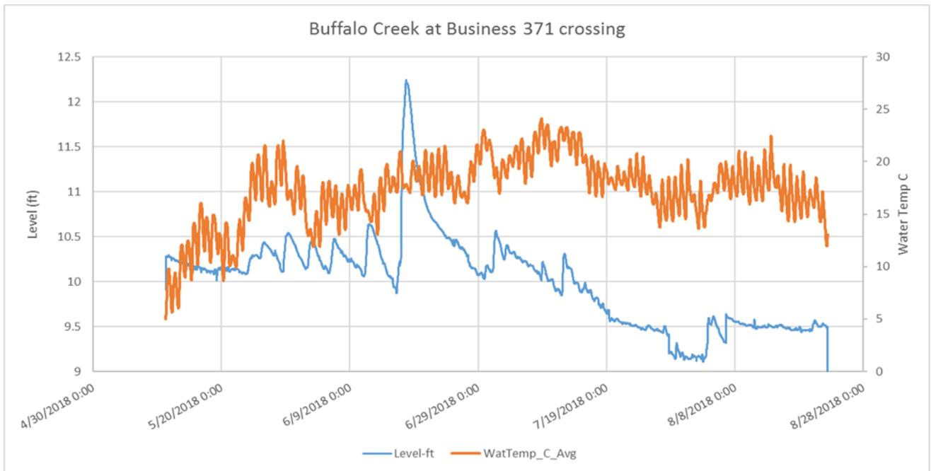
Probe was pulled out. Level is wrong after 8/2/2018. Water temp appears OK.
