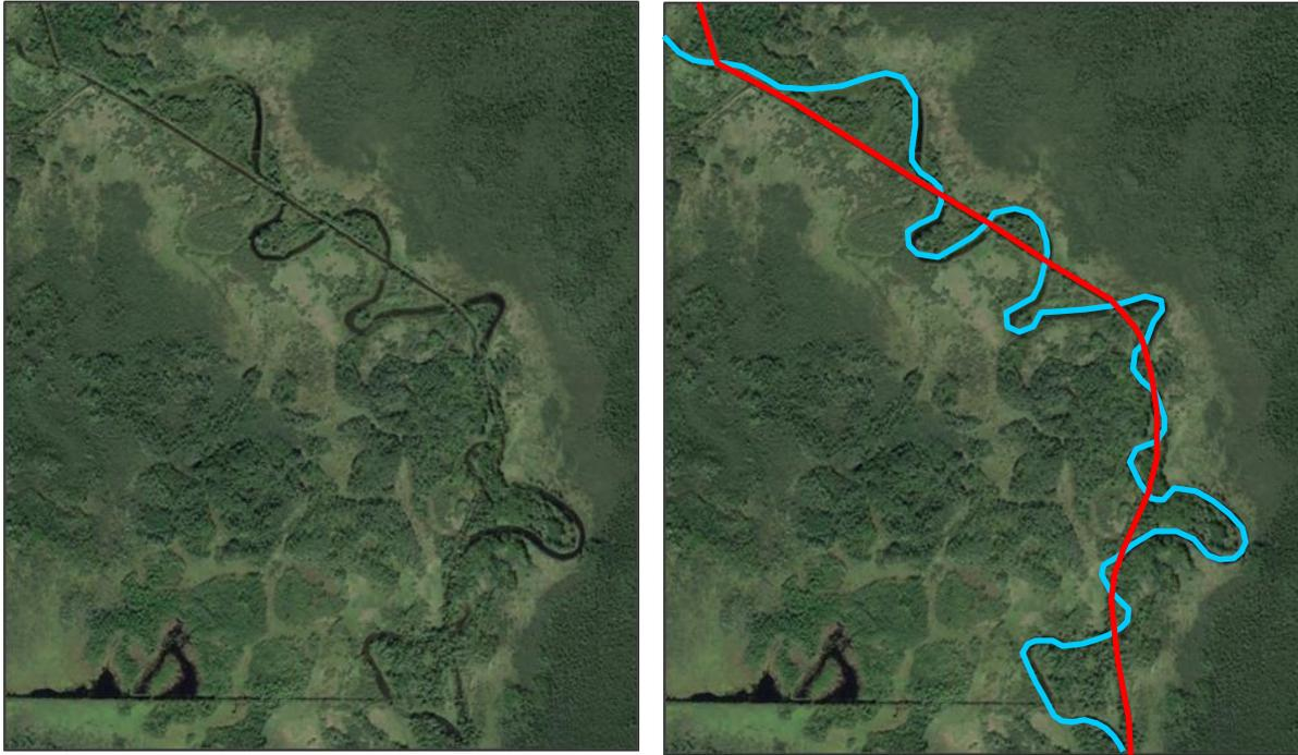
Figure 57. Tentative assessment of un-needed legacy ditches through peatlands. Portions of the MRGRW, which are not shown, have little of this ditching.
