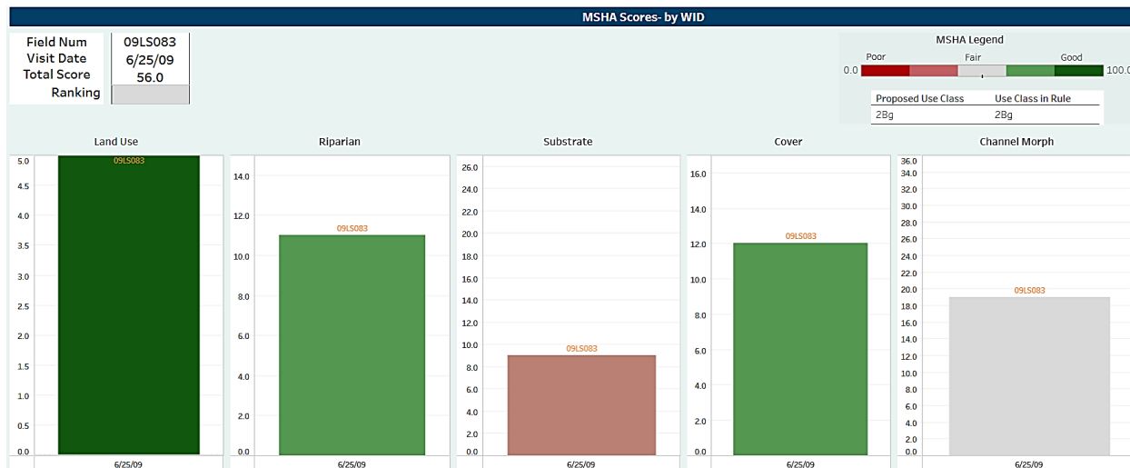
Figure 15: MSHA results for station 09LS083 on the impaired reach of Long Lake Creek. Metric scores ranked poorly for stream substrate quality and channel morphology
