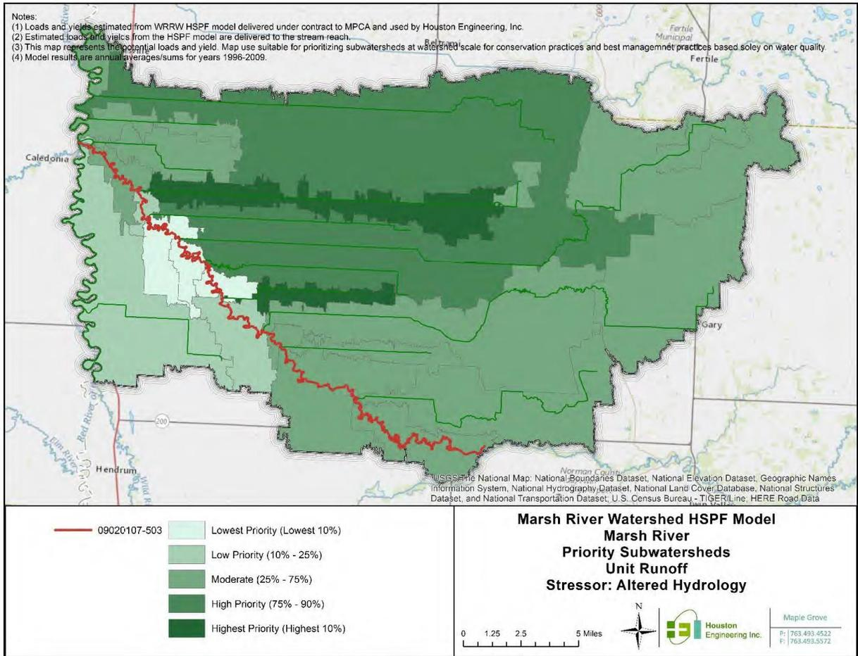
**Figure B-12: Map of prioritized subwatersheds for implementation to address excessive nutrients in the Marsh River Watershed, based on average (1996-2009) annual total phosphorus yields.**
