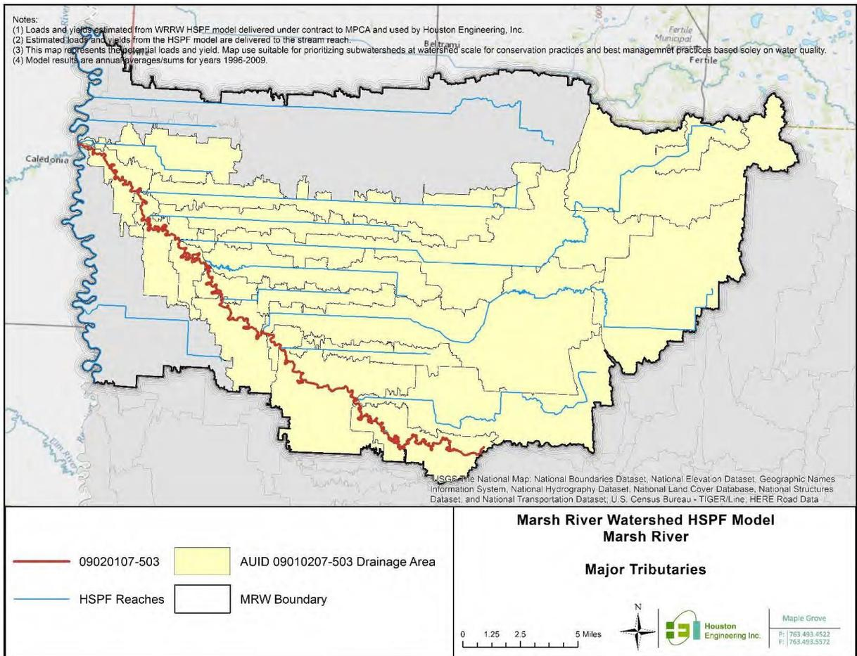
**Figure B-20: Map of prioritized subwatersheds for implementation to address altered hydrology in the Marsh River (AUID 09020107-503), based on average (1996-2009) annual runoff.**
