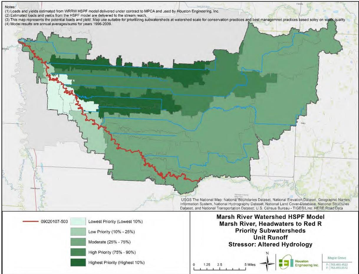
**Figure B-21: Map of prioritized subwatersheds for implementation to address excessive nutrients in the Marsh River (AUID 09020107-503), based on average (1996-2009) annual total phosphorus yields.**
