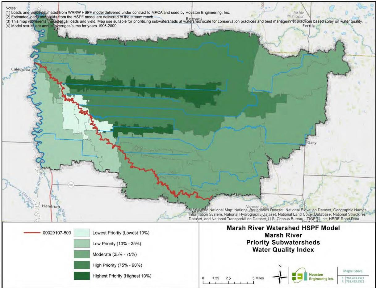
**Figure B-16: Map of prioritized subwatersheds for implementation of field and stream practices (Field Stream Index) to address excessive nutrients, based on average (1996-2009) annual total phosphorus load.**
