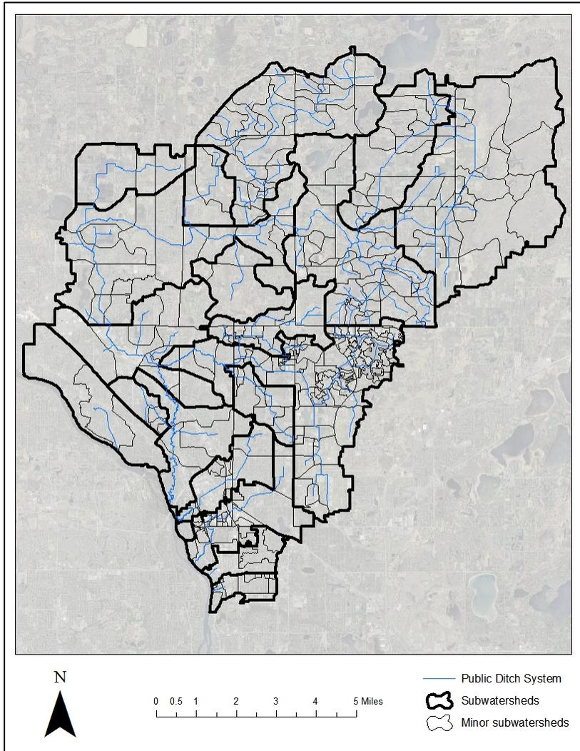
Figure 5. Subwatersheds and minor-subwatersheds delineated with LiDAR information.
