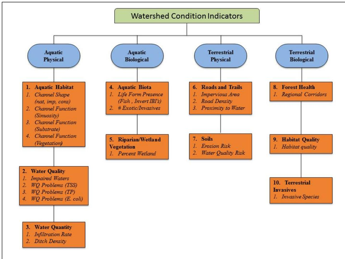
Figure 15 Conceptual model of Watershed Condition Classification assessment.
