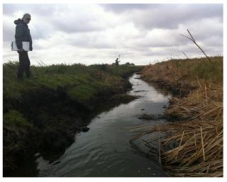
• Bankfull width is extraordinary wide due to ditch geomorphology, reach position within a wetland complex and Red River Valley flooding characteristics; thus the W/D ratio is also very high; this phenomenon is common throughout this study area
