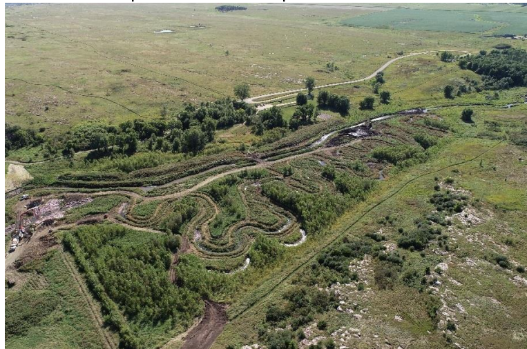
Figure 5. Stream restoration project in Mound Creek. Stream channel re-meandering, bank shaping, and grade control riffles restore natural features of the creek which improve conditions for aquatic life.
