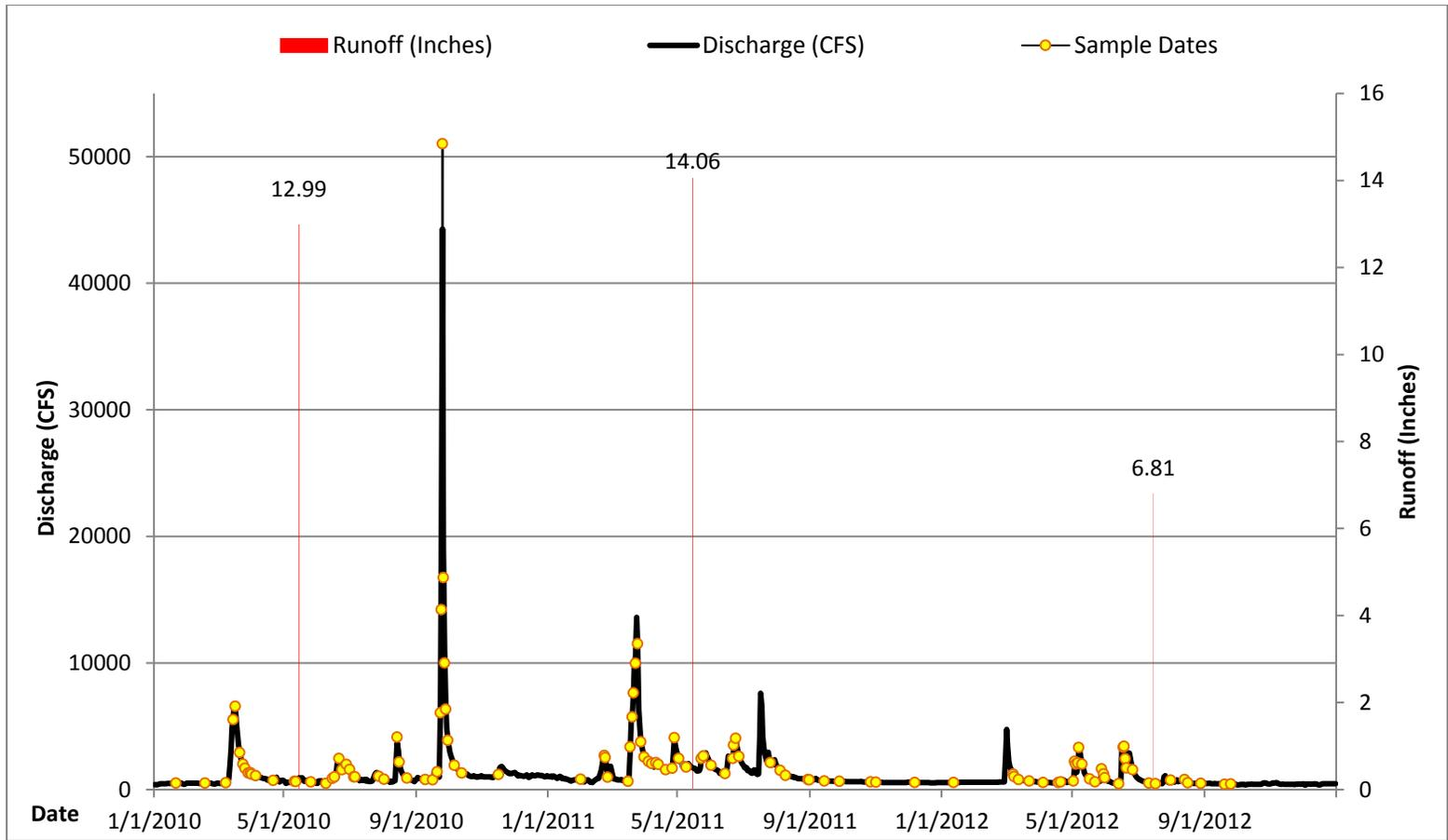
Figure 22. Hydrograph and annual runoff for the Zumbro River near Kellogg, Minnesota (2010-2012).
