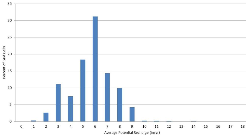
Figure 17. Average annual potential recharge rate percent of grid cells in the Mississippi River (Headwaters) Watershed (1996-2010).
