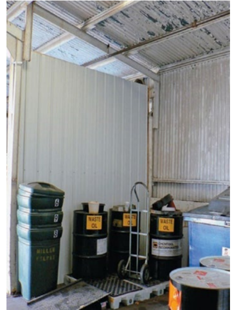
This facility avoids exposing pollutants to stormwater by collecting and storing waste fluids indoors with secondary containment.
