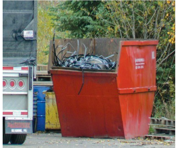
Uncovered scrap bins do not meet the No Exposure requirements.
