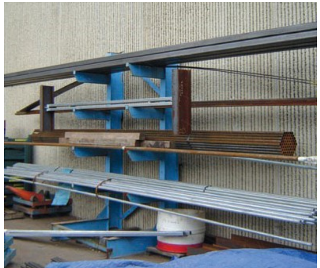
Materials such as raw steel, or steel coated with oil, need to be sheltered to qualify for the No Exposure Exclusion.
