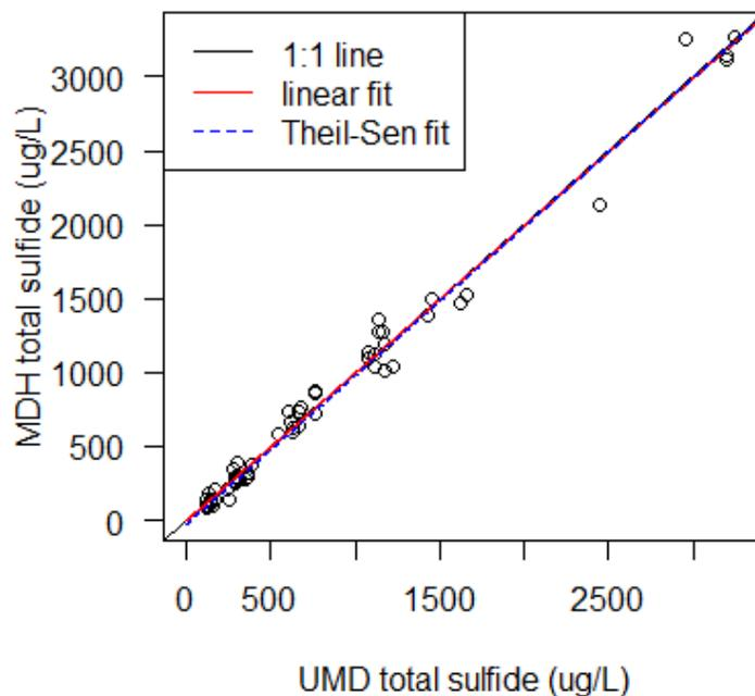
Figure 1. Comparison of sulfide data produced by the UMD lab and the MDH lab from the fourth vessel of each treatment in the hydroponic seedling experiments.  $r^2 = 0.99$ ,  $n = 59$ ; the linear regression equation is:  $\text{MDH} = 0.997 \text{ UMD} - 2.2$ . The Theil-Sen fit refers to a non-parametric regression method, which confirms the similarity of the sulfide analyses performed by the two laboratories.
