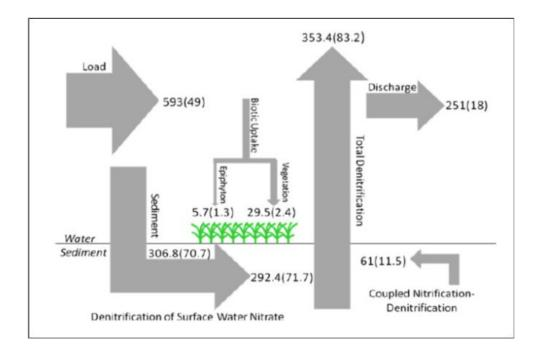
Figure 26. Net NO<sub>3</sub>-N budget (mean (1 SE), (mg m-2 h-1) for Third Lake, Navigation Pool 5 during June and July 2005. n = 3 for discharge and load, n = 8 for coupled nitrification–denitrification and total denitrification, n = 16 for biotic uptake and denitrification of surface water nitrate. Reprinted from Kreiling et al. (2010).
