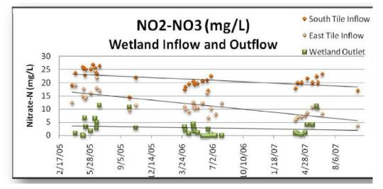
Figure 33. Inlet and outlet NO<sub>x</sub>-N concentration for County Ditch 58 constructed wetland, located in Seven Mile Creek watershed in Minnesota, from 2005 to 2007. East tile inflow was treated by another upstream constructed wetland prior to the County Ditch wetland. Reprinted from Kuehner (2009).
