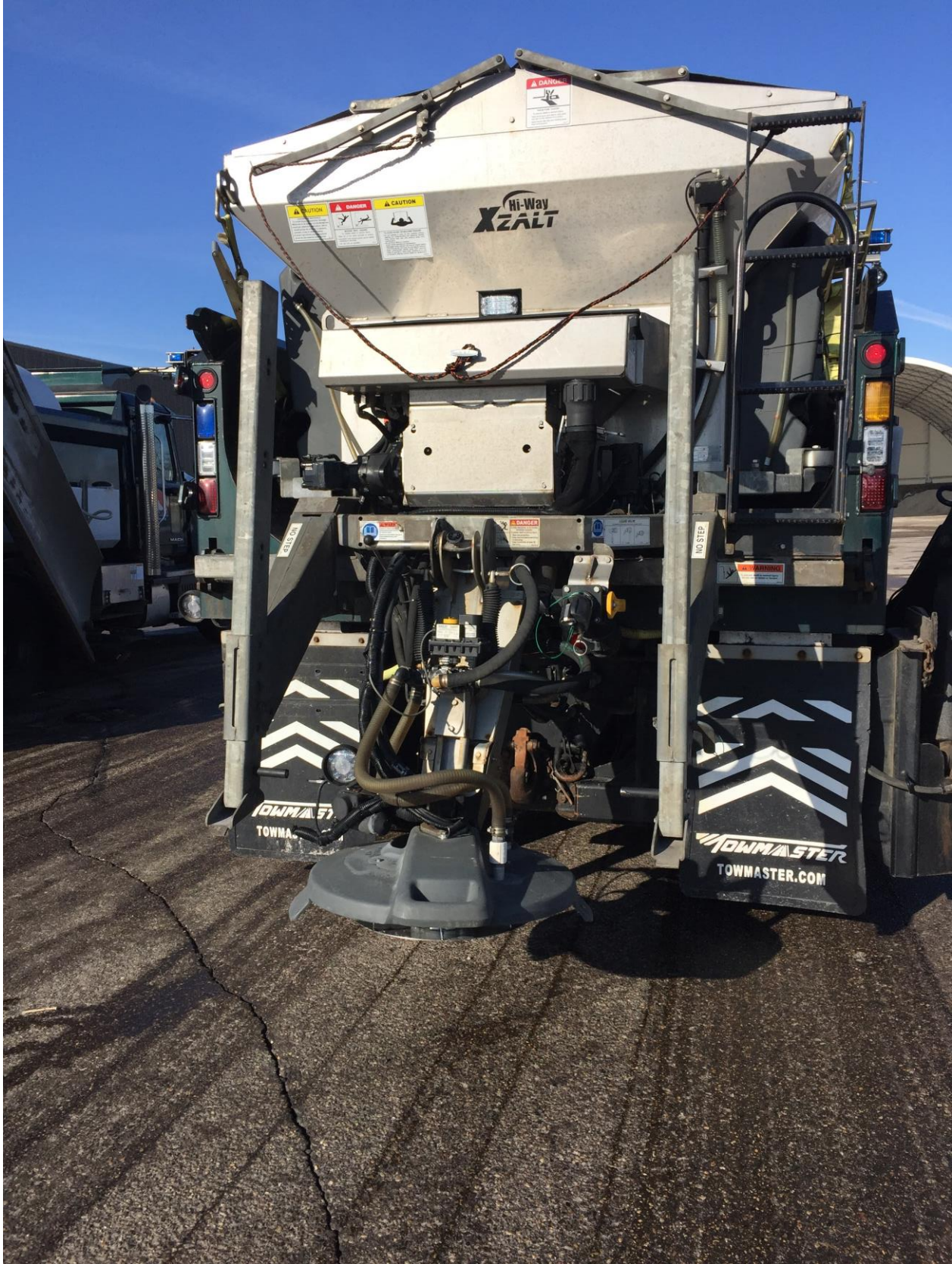
Figure 74: City of Waconia Truck capable of dry/liquid material mix application.
