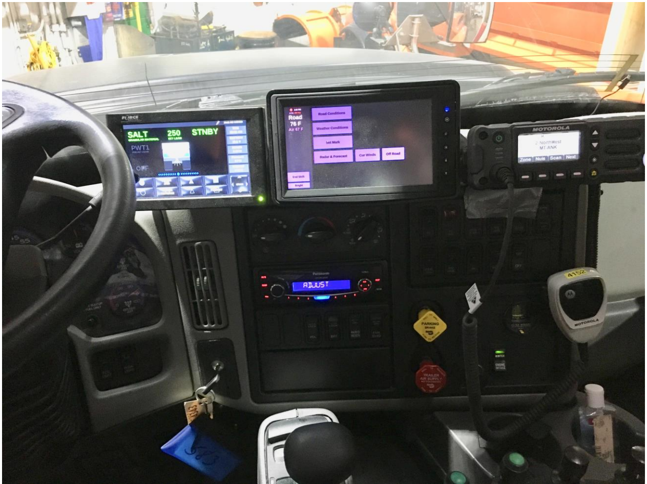
Figure 76: Inside look at MDS/MDSS of a MndOT Plow Truck
