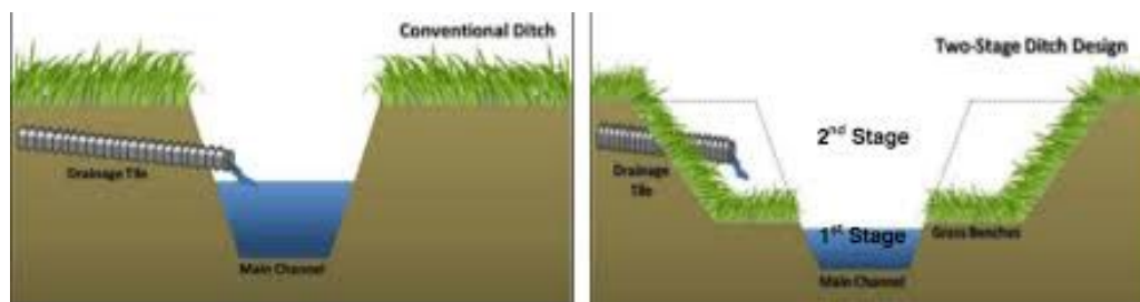
Figure 23. Two-stage ditch design diagrams. (Board of Water and Soil Resources 2020).
