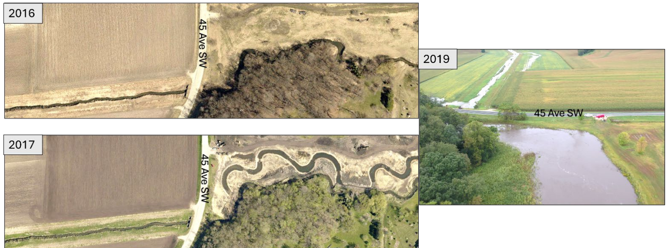
Figure 31. Aerial photos of Cascade Creek, Rochester, Minnesota, before (upper left) and after (lower left) restoration at 45 th Ave. The after-restoration aerial photo was taken shortly after the floodplain was reconnected to the channel. The drone image (right) was captured during a flood event when the newly constructed floodplain was activated and can be compared to the upstream incised stream channel, also at 45 th Ave.
