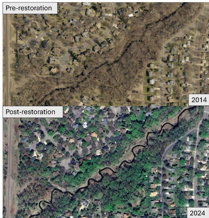
Figure 30. Before (upper) and after (lower) construction of a restoration based on Natural Channel Design Principles. Channel dimension, pattern and profile were informed by a reference reach. Sand Creek, Coon Rapids, Minnesota. (photo Minnesota Department of Natural Resources).
