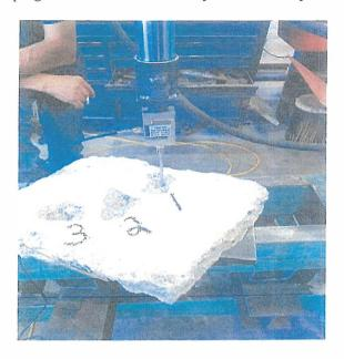
Below is a picture of the load cell that was used to measure the dislodging force
