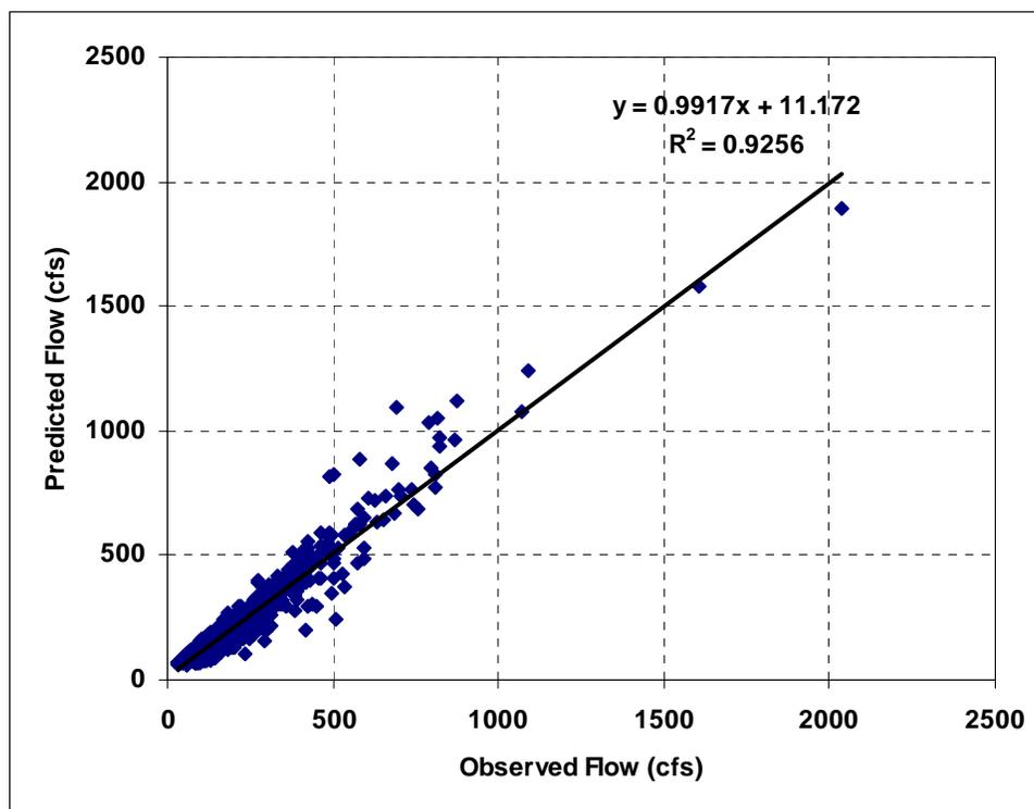
**Figure 4-7. Comparison of observed and predicted flows at the MCES gage at Hastings 1995—2002.**
