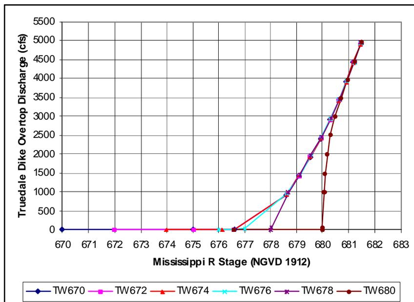
Figure 4-17. Truedale Slough dike overtop discharge at various tailwater elevations.
