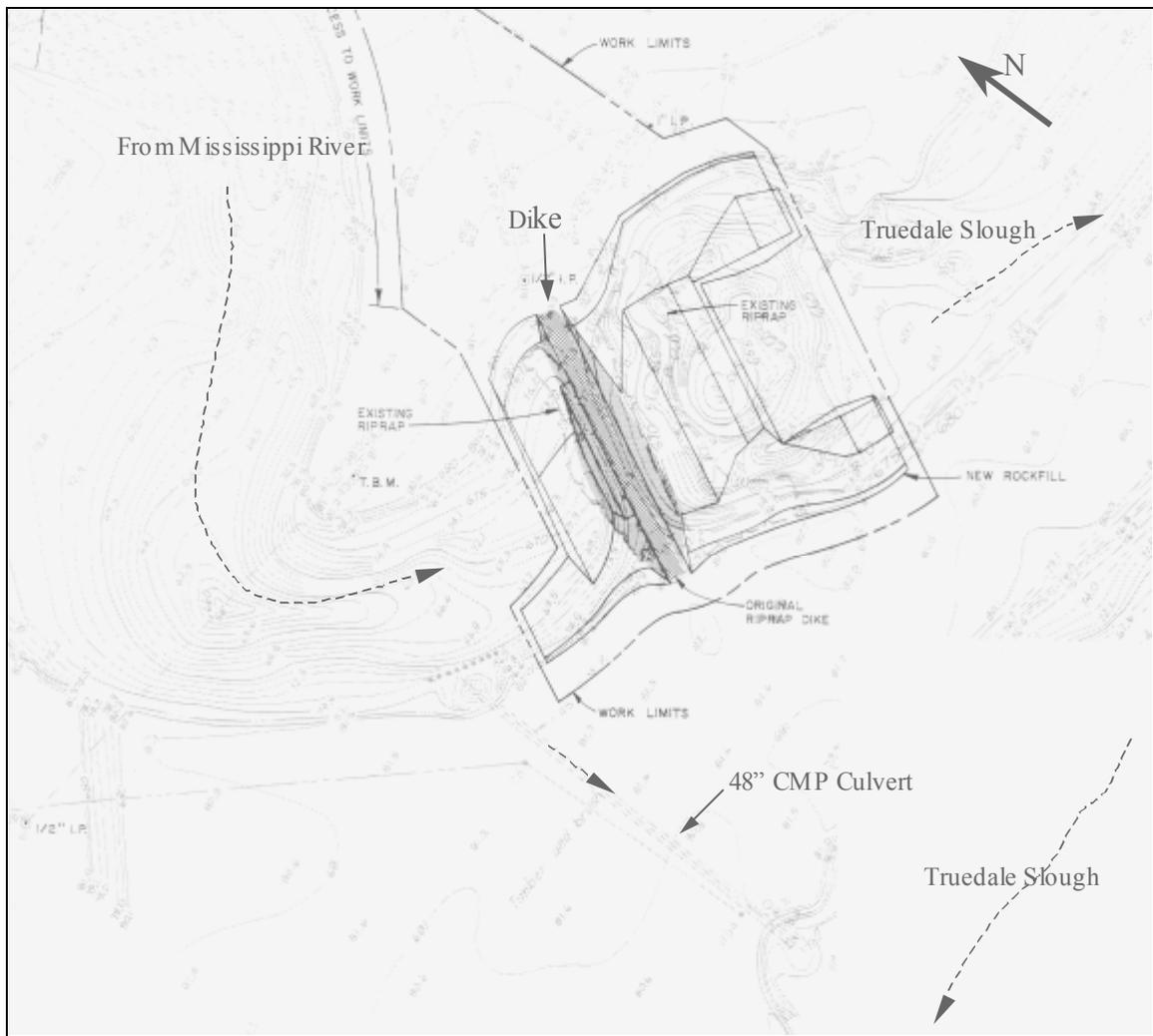
**Figure 4-13. Plan View of Truedale Slough Dike and Culvert**
