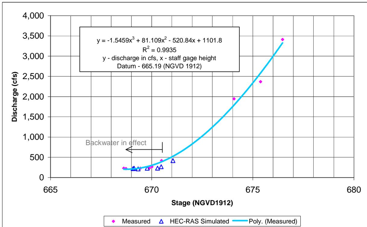
**Figure 4-28. Stage-discharge relationship at Etter Bridge.**
