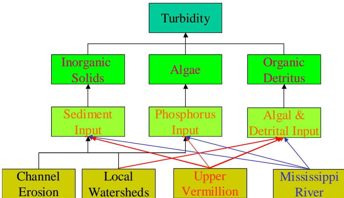
Figure 3-1. General conceptual model of turbidity in the LVR.
