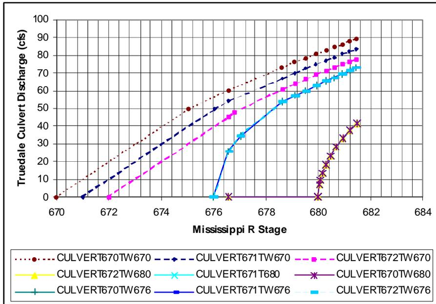
Figure 4-16. Truedale Slough culvert discharge sensitivity to invert elevation.
