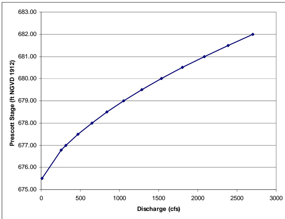
**Figure 4-11. Preliminary stage-discharge relationship for the Vermillion Slough (modular flow into the slough).**
