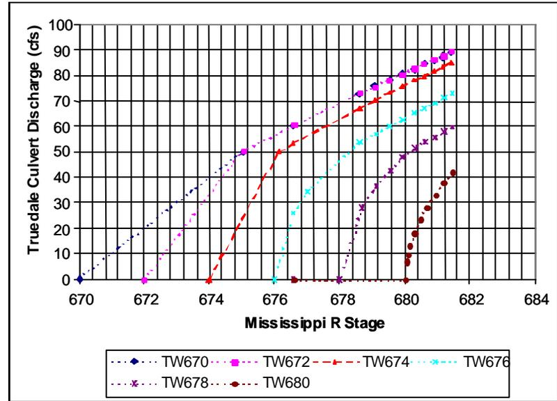
Figure 4-15. Truedale Slough culvert discharge as a function of Mississippi River Pool 3 stage.
