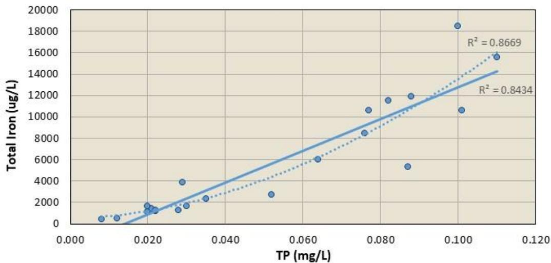
Figure 3-14. Musselshell Creek (S009-505) TP vs total iron. The very high correlation of these concentrations suggests their source being peatland soils. The dotted line is a 3<sup>rd</sup> order polynomial regression line, with a slightly better R<sup>2</sup> value than the linear model.
