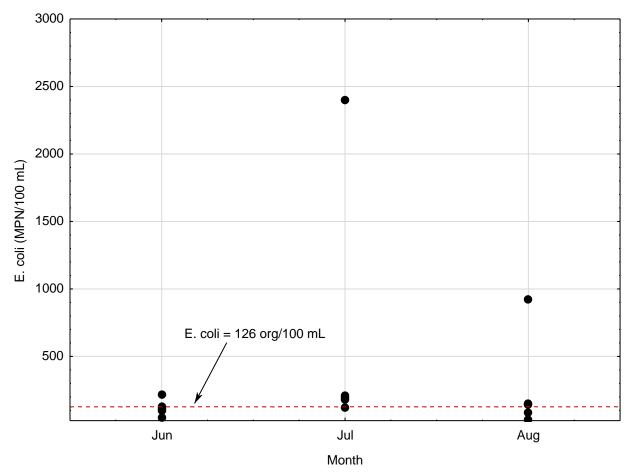
Figure 3-6. *E. coli* (MPN/100ml) by month in Hasty Brook (07010103-603) at monitoring station S005-777, 2007-2016. The dashed line represents the stream water quality standard (126 org/100ml).
