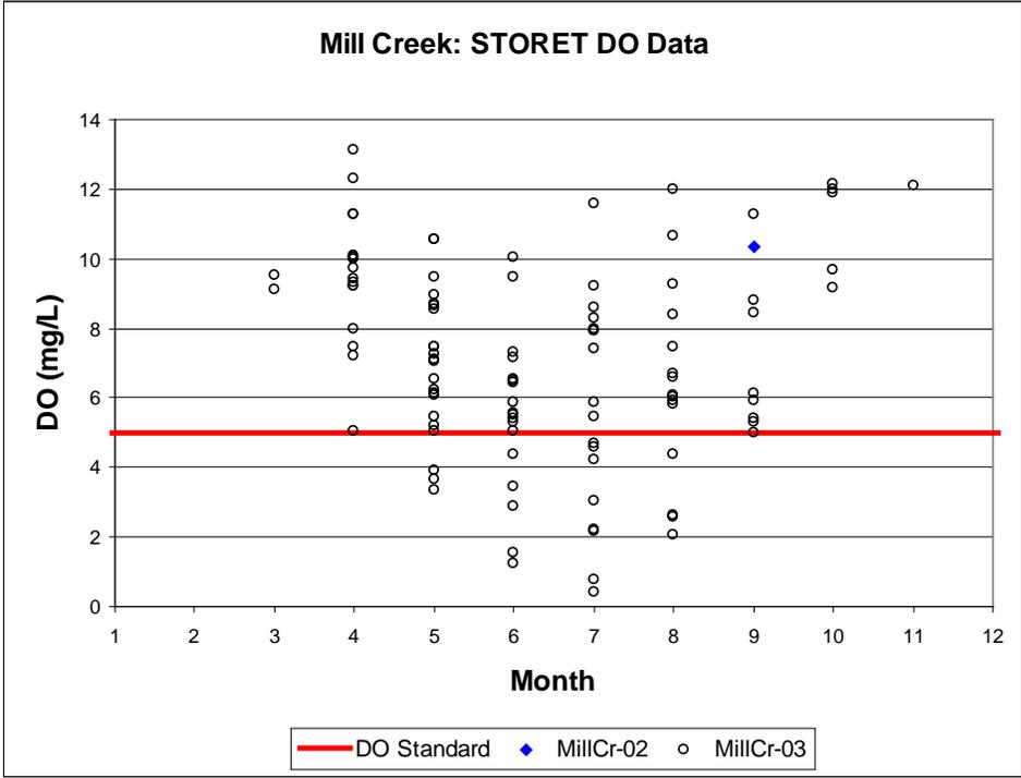
**Figure 2.2** Dissolved oxygen data from STORET for all Mill Creek stations by month, regardless of year.
