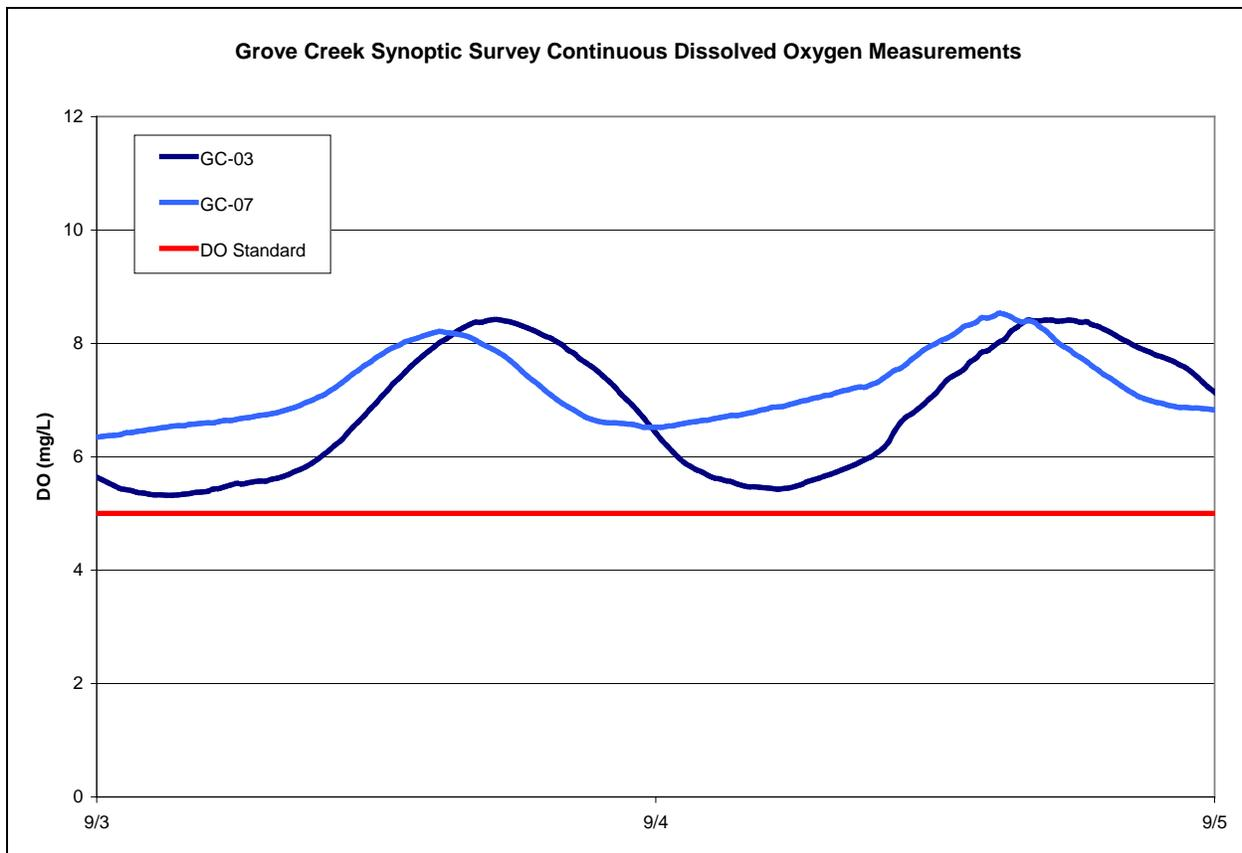
Figure 4.9 Synoptic survey continuous dissolved oxygen concentrations.
