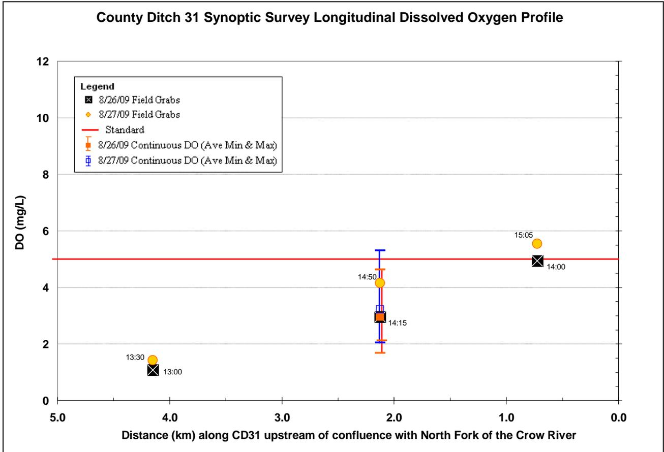
Figure 4.10 Dissolved oxygen observations during the August 2009 synoptic survey.
