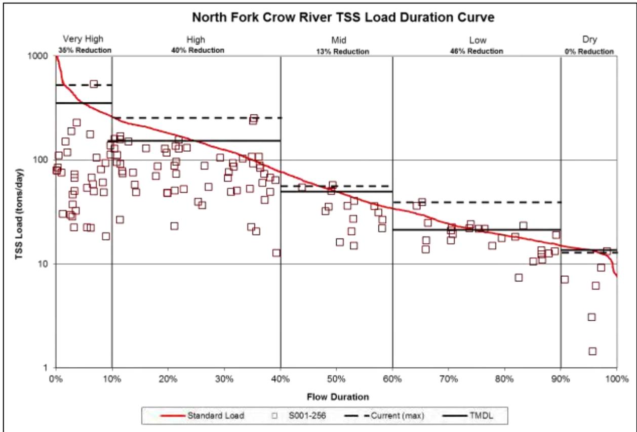
Figure 3.4. North Fork Crow River Impaired Reach (07010204-503) TSS Load Duration Curve and necessary TSS reductions to meet TMDL.
