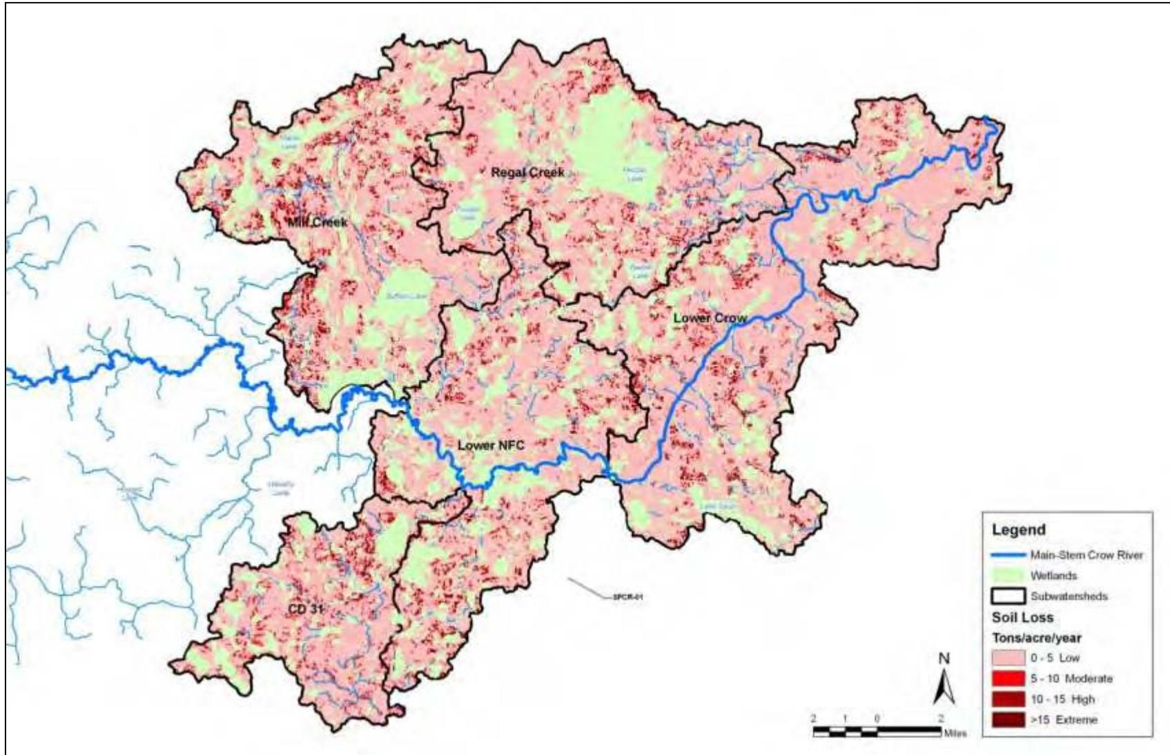
Figure 3.8. Average annual soil loss per acre for the North Fork Crow and Lower Crow River impaired reach study areas calculated using the USLE.
