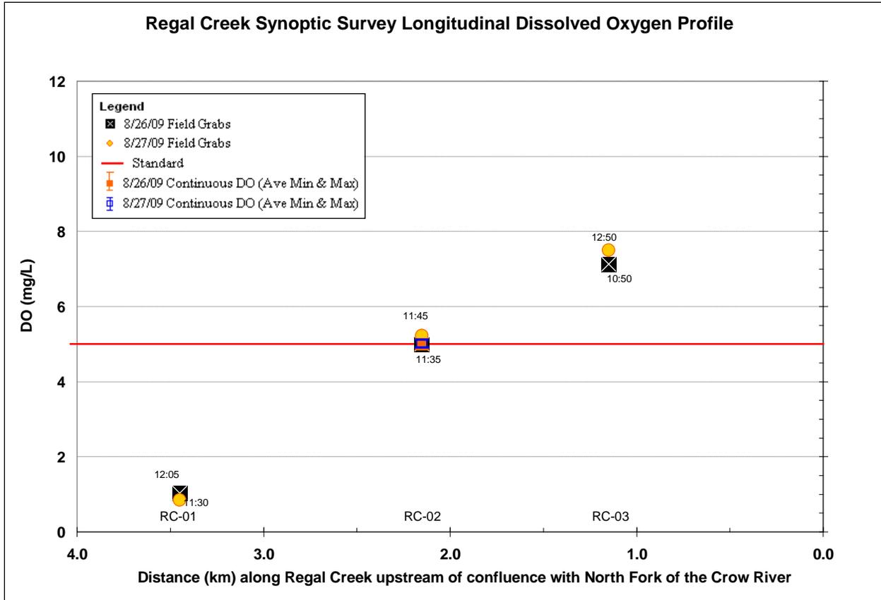
Figure 4.8 Dissolved oxygen observations during the August 2009 synoptic survey.
