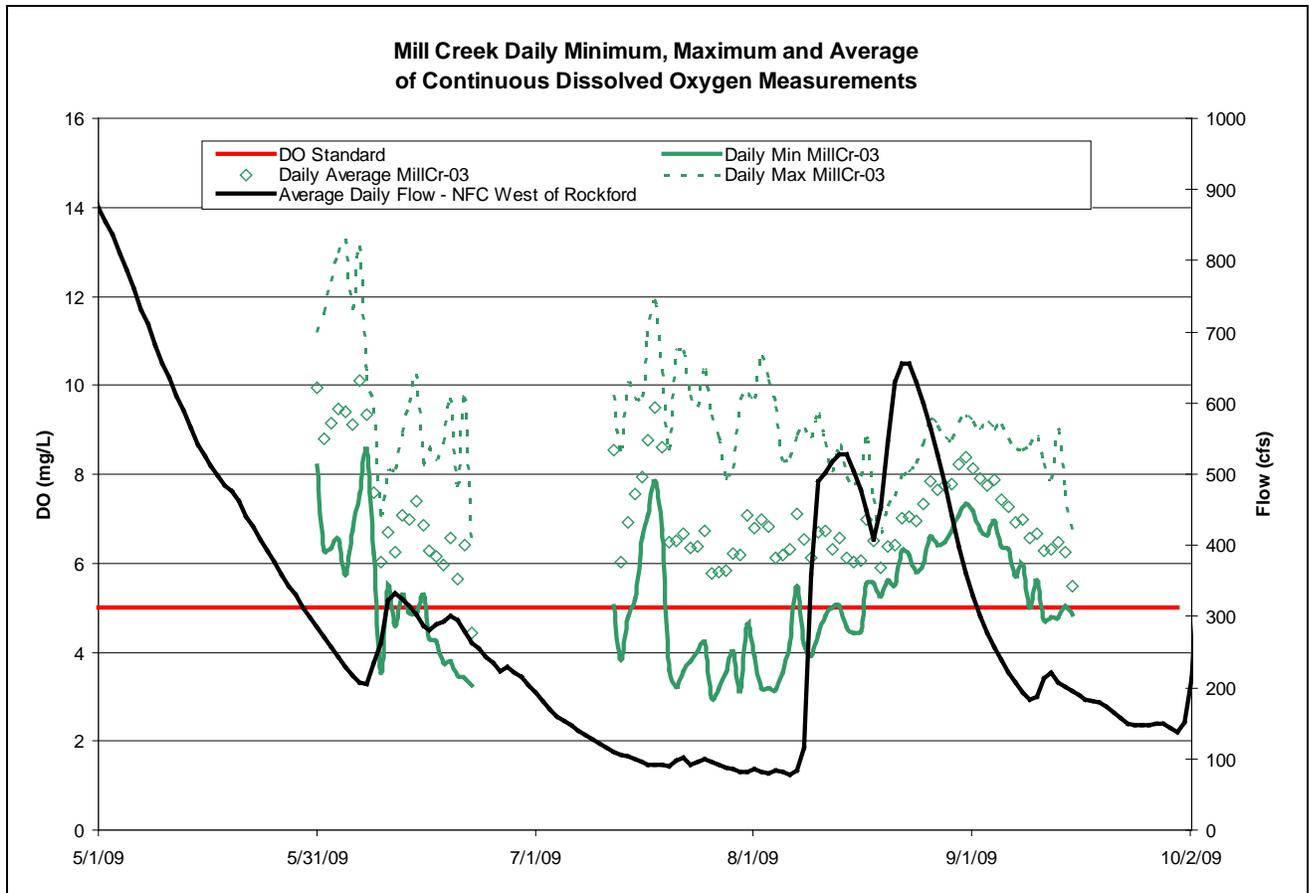
Figure 2.4 Statistics of continuous dissolved oxygen data collected in 2009.
