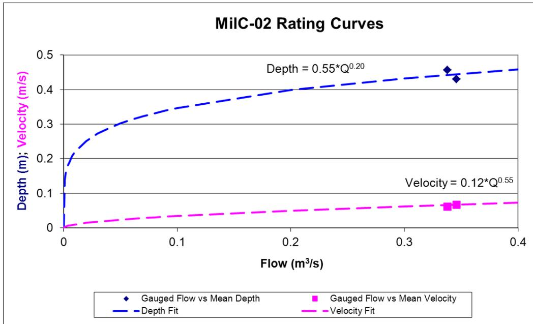
Figure 3.1 Hydraulic rating curve plot for gauging station MilC-02.
