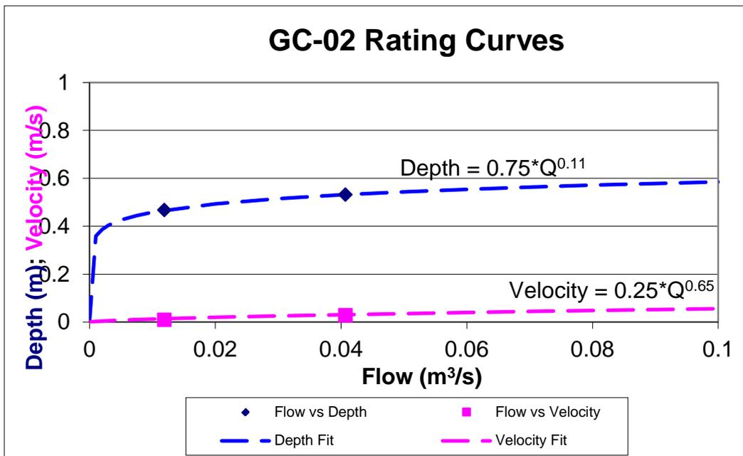
Figure 3.1 Hydraulic rating curve plot for gauging stations GC-02.
