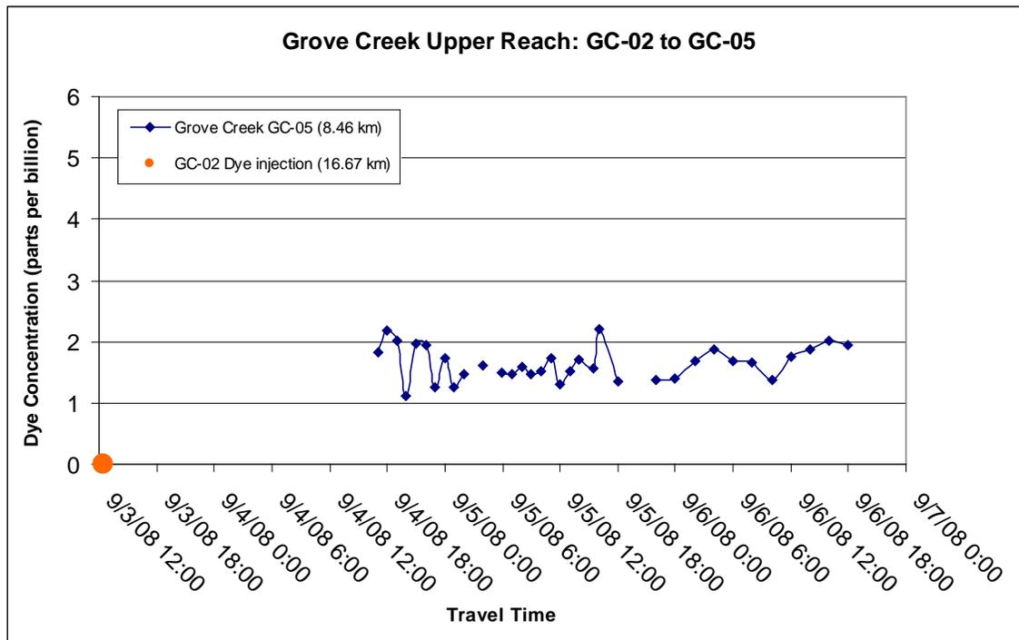
**Figure 4.1:** Dye concentration measurements from station GC-05.
