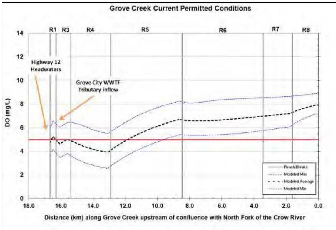
Figure 4.9. Grove Creek current permitted conditions QUAL2K model run.
