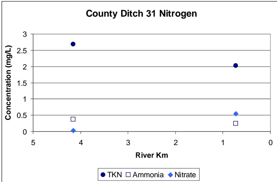
Figure 4.4 August 26, 2009 synoptic survey grab lab results for CD31.
