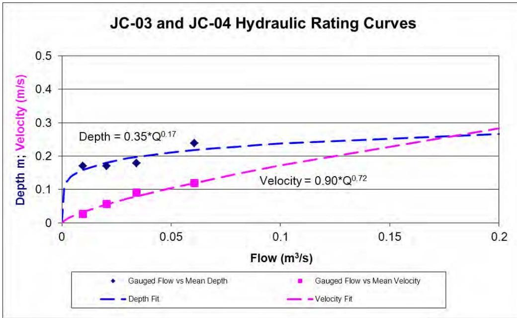
Figure 3.1 Hydraulic rating curve plot for gauging stations JC-03 and JC-04.
