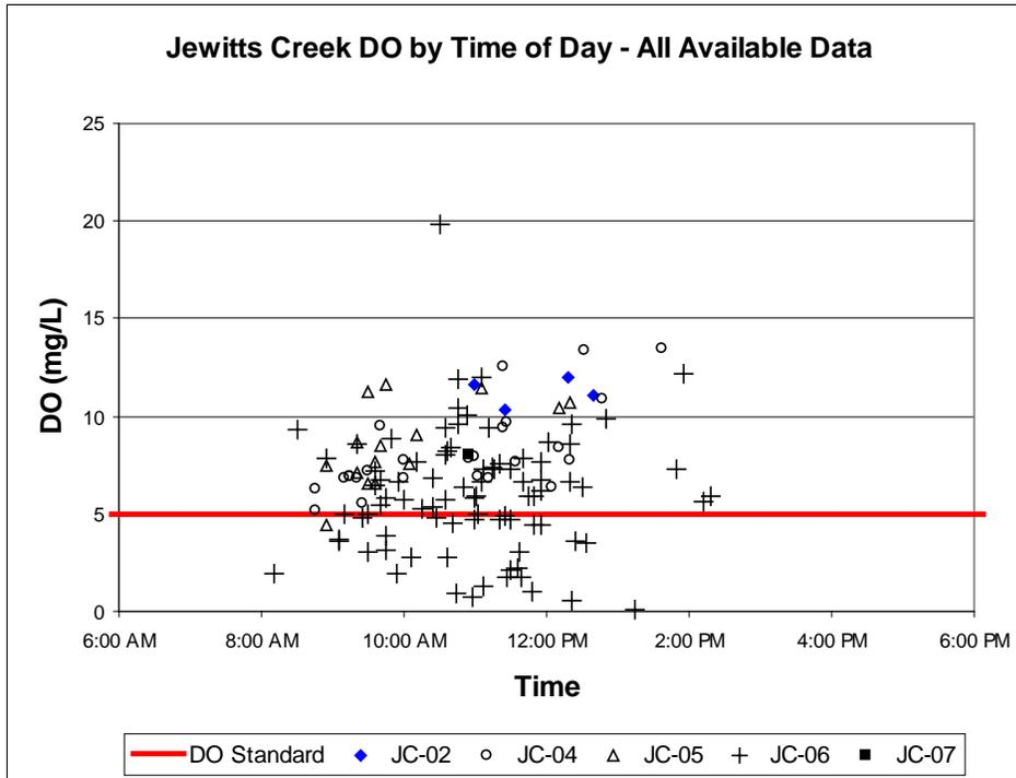
**Figure 2.3** Dissolved oxygen data from STORET for all Jewitts Creek stations by time of day, regardless of year and month. No data has been collected prior to 8:00 am or later than 4:00 pm.
