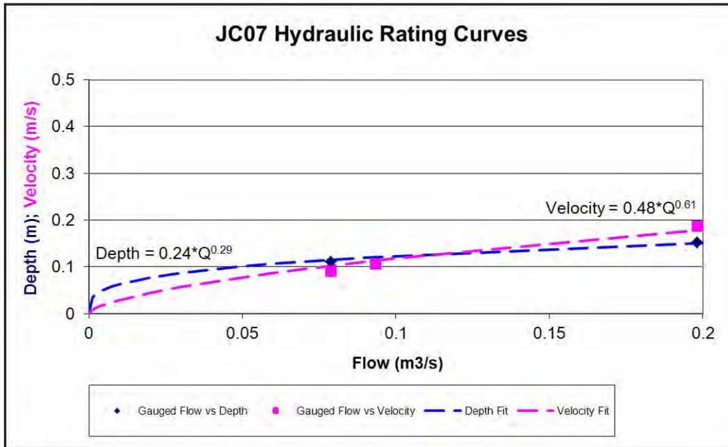
Figure 3.3 Hydraulic rating curve plot for gauging stations JC-07
