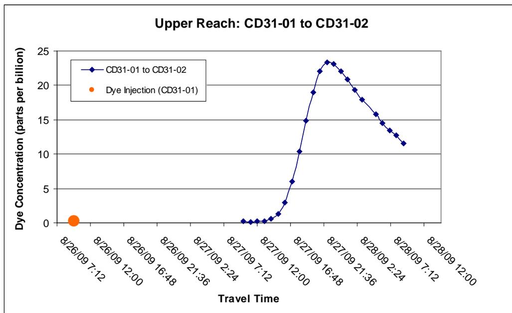
**Figure 4.1** Dye concentration measurements from station CD31-02.
