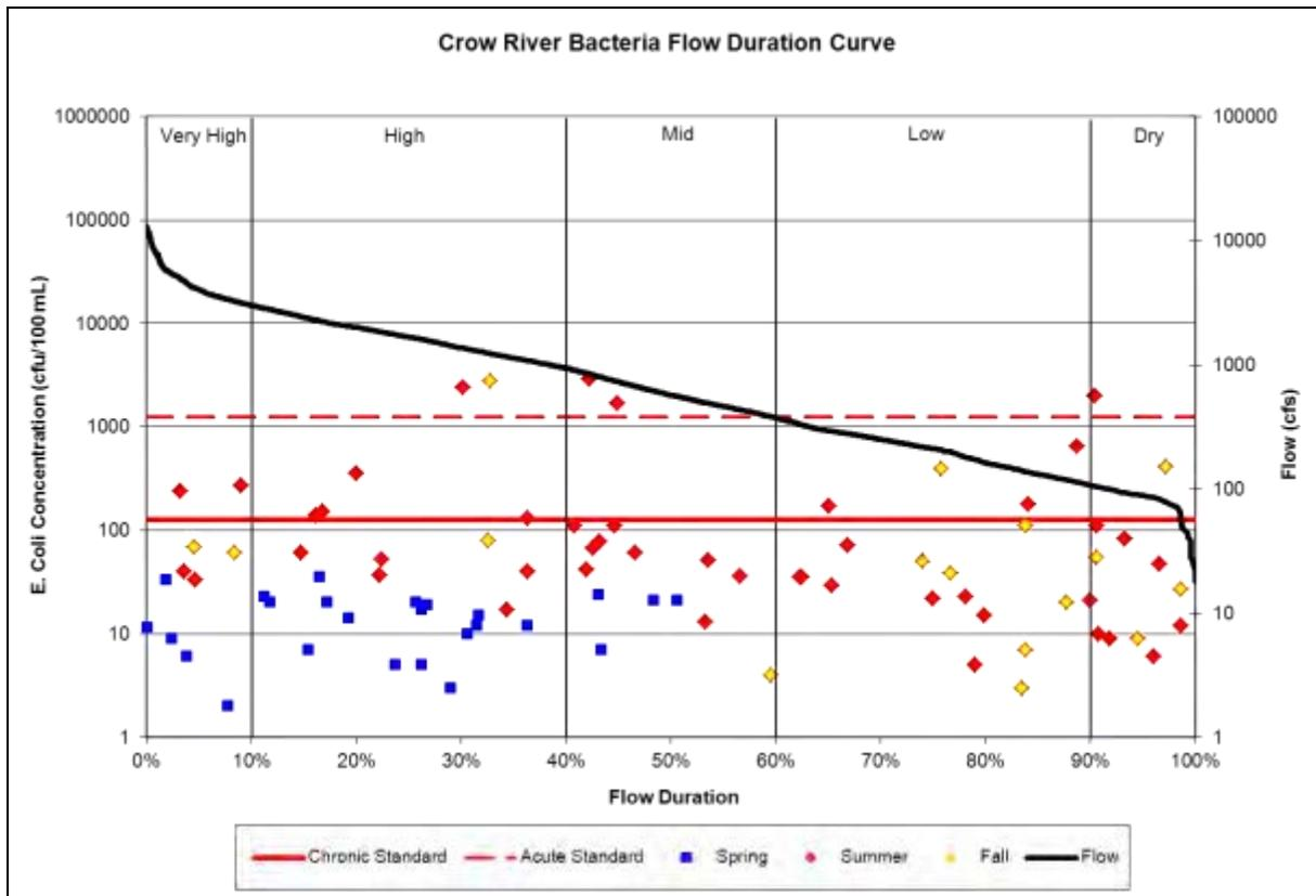
Figure 2.5. Individual *E. coli* measurements in the Lower Crow River impaired reach plotted by season and flow regime.
