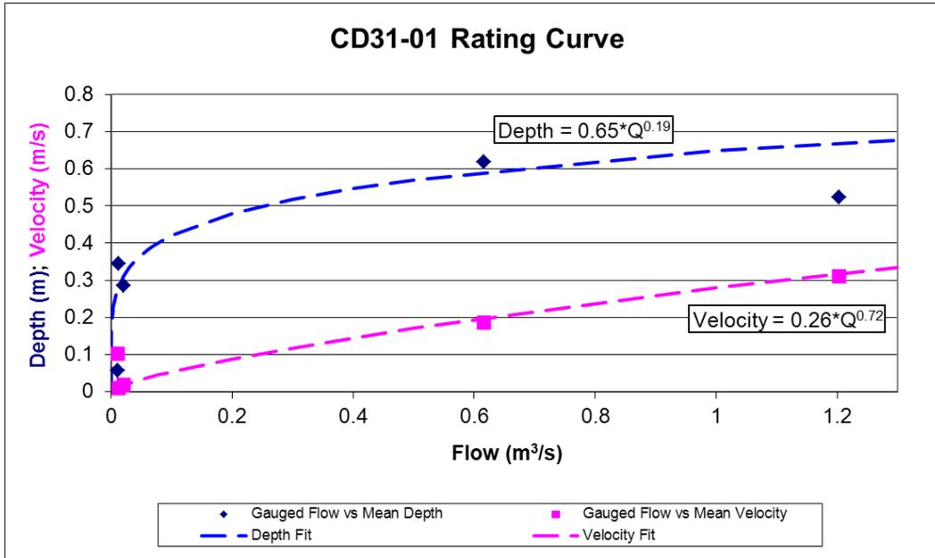
**Figure 3.1** Hydraulic rating curve plot for gauging station CD31-01.
