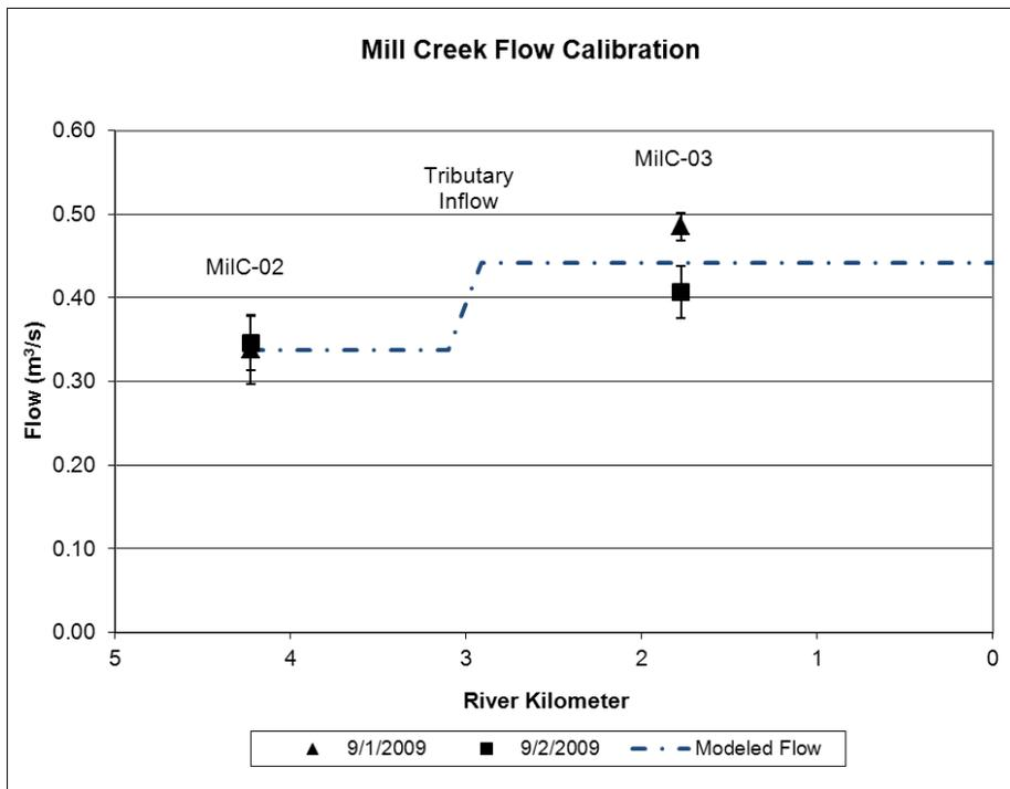
**Figure 3.3** Final Mill Creek flow calibration with tributary inflow.
