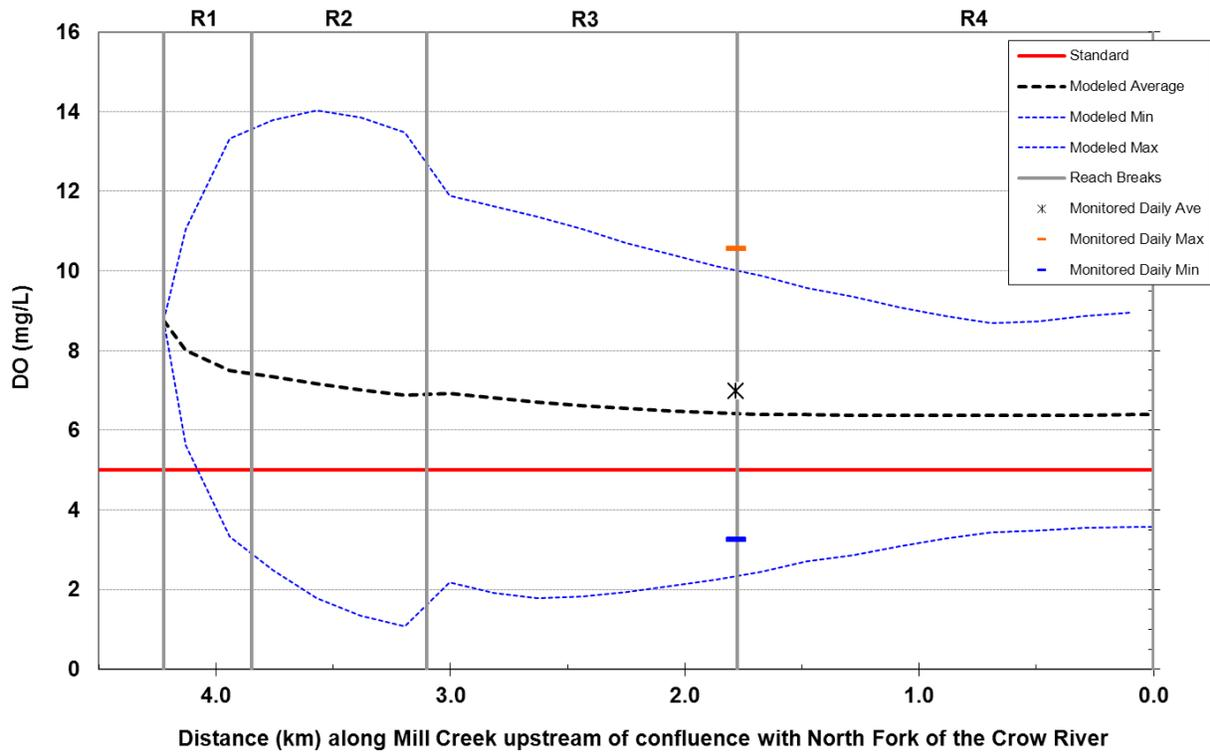
Figure 6.1 Mill Creek August 3<sup>rd</sup> low-flow model simulation dissolved oxygen longitudinal profile.
