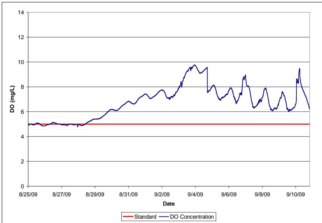
**Figure 2.5** Continuous DO measurements at Station S002-030 from 8/25/09 to 9/11/2009 (preliminary data supplied by the MPCA).
