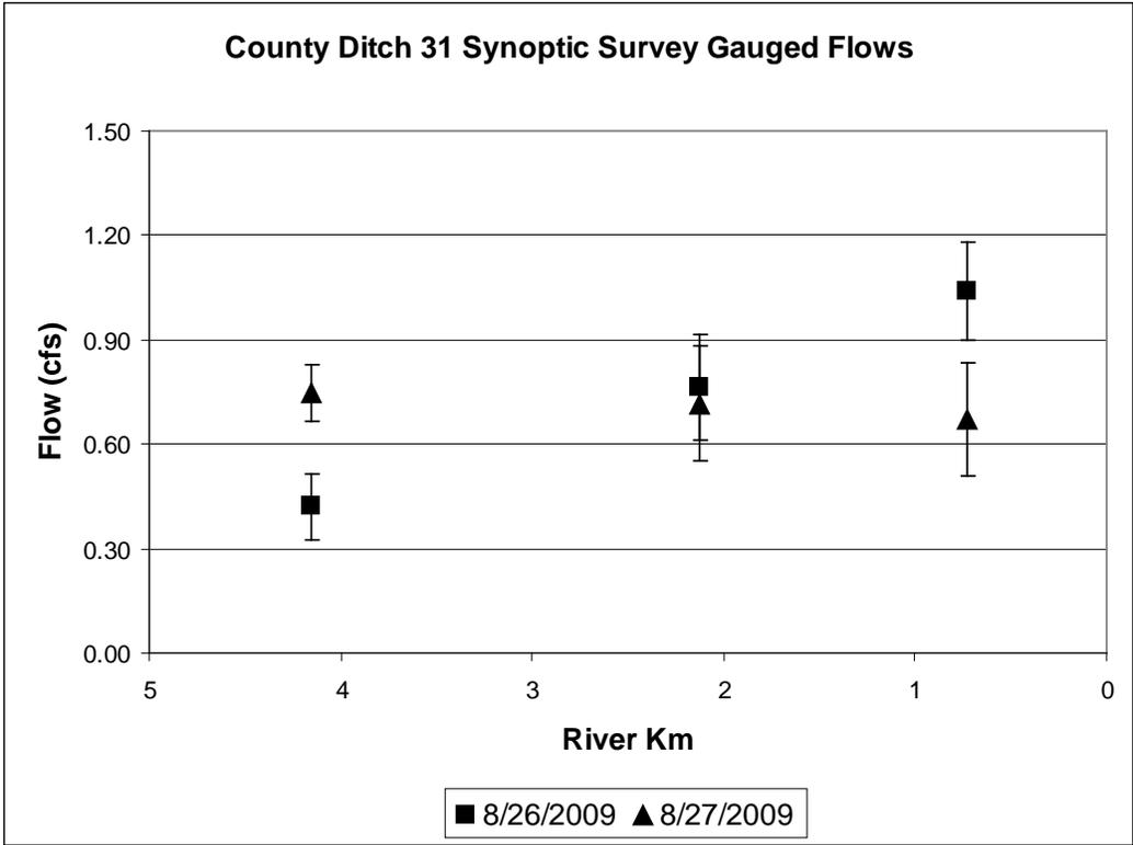
**Figures 4.3** Gauged flows by river kilometer for the CD31 synoptic survey. Error bars represent estimated uncertainty of the Flow-Tracker field measurement.
