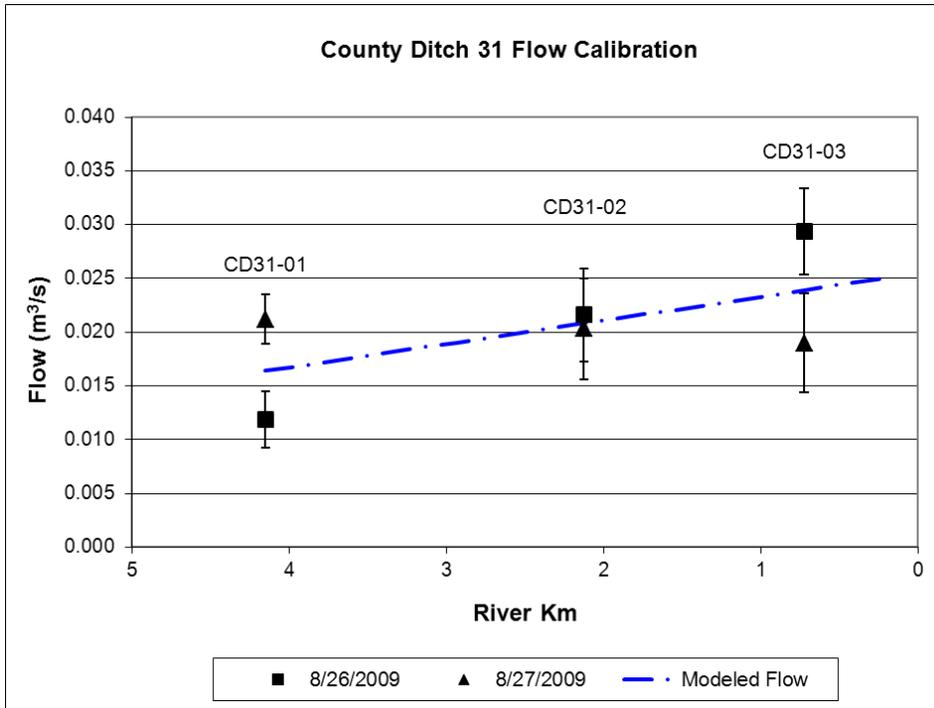
**Figure 3.4** Final County Ditch 31 Flow calibration with diffuse and point source inflows.
