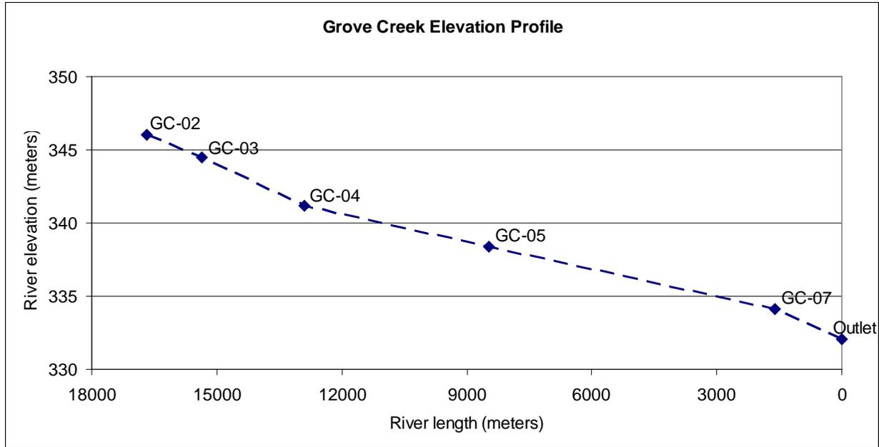
**Figure 2.1** Survey elevations used to estimate reach slopes for Grove Creek.
