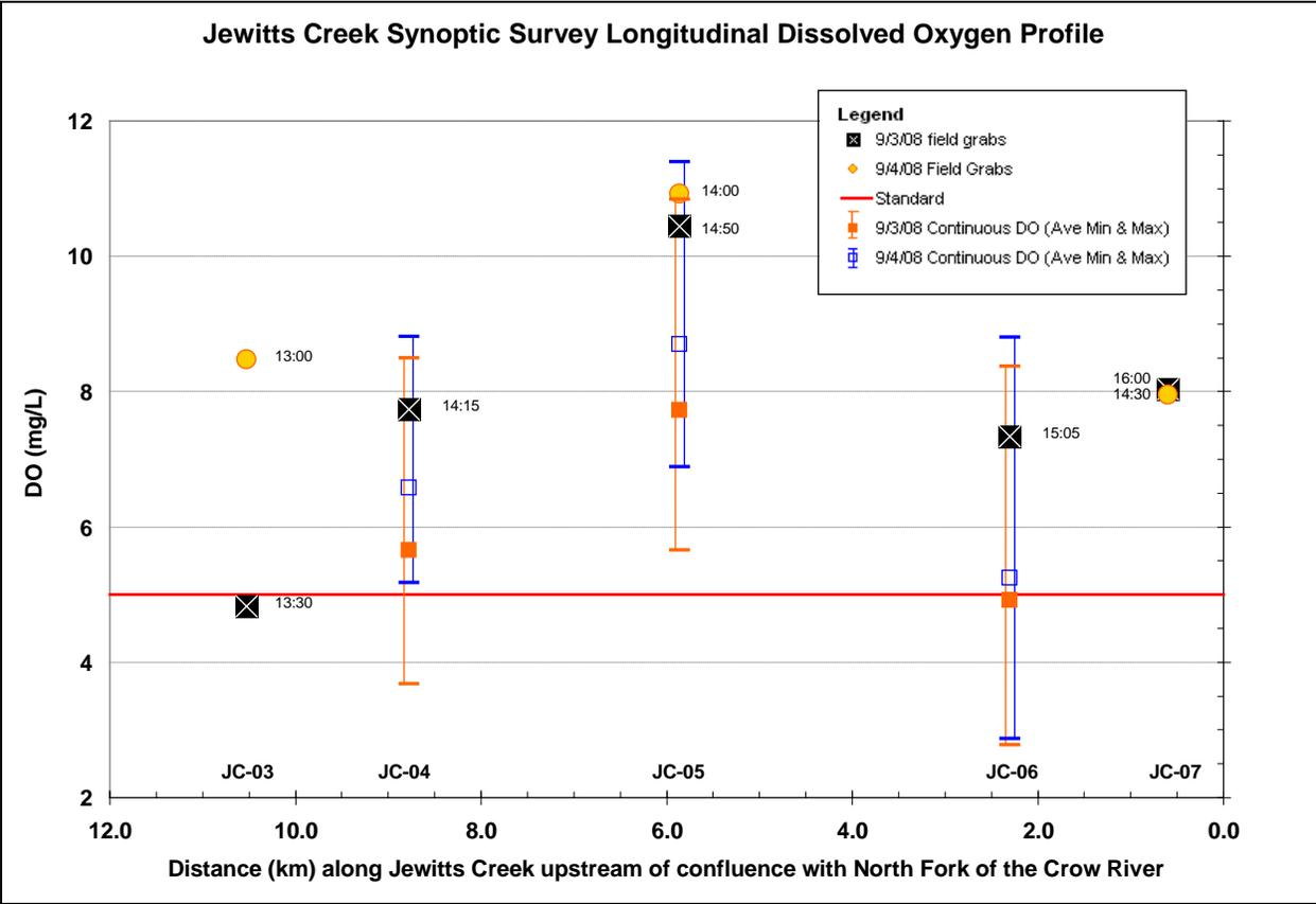
Figure 4.10 Dissolved oxygen observations during the September 2008 synoptic survey.
