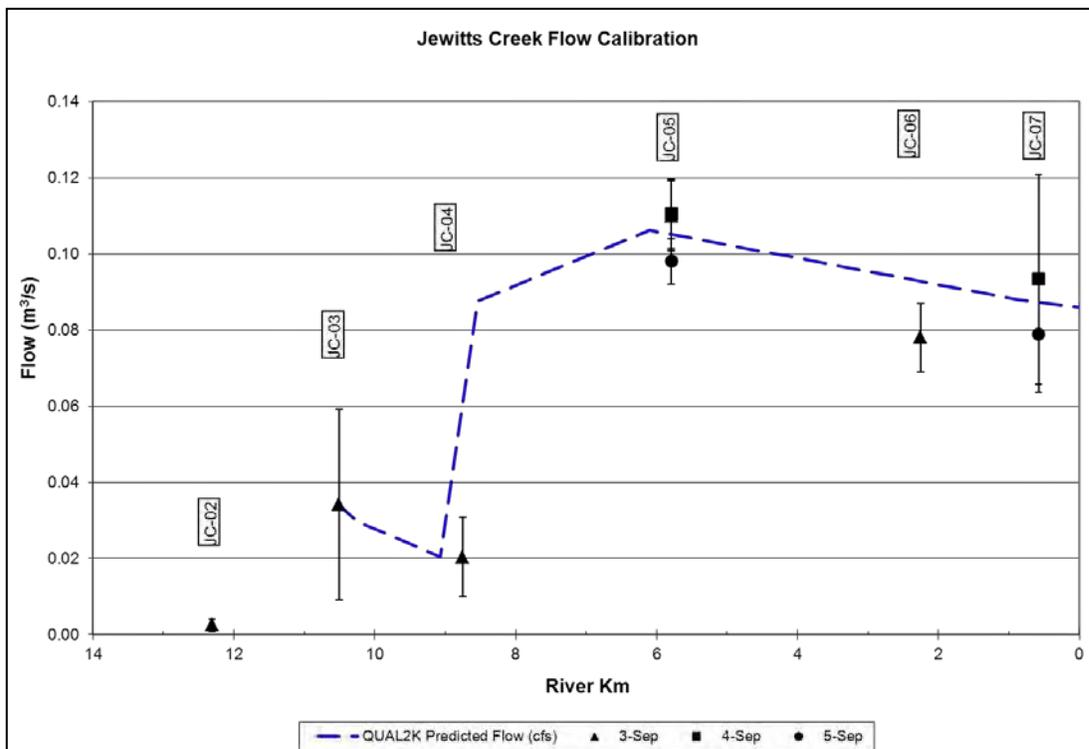
**Figure 3.4** Final Jewitts Creek Flow calibration with diffuse and point source inflows.
