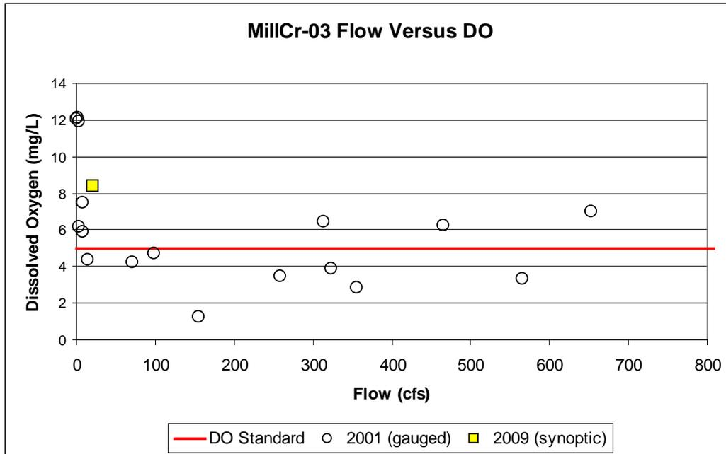
Figure 2.5 MillCr-03 dissolved oxygen compared to gauged and continuous flow measurement.
