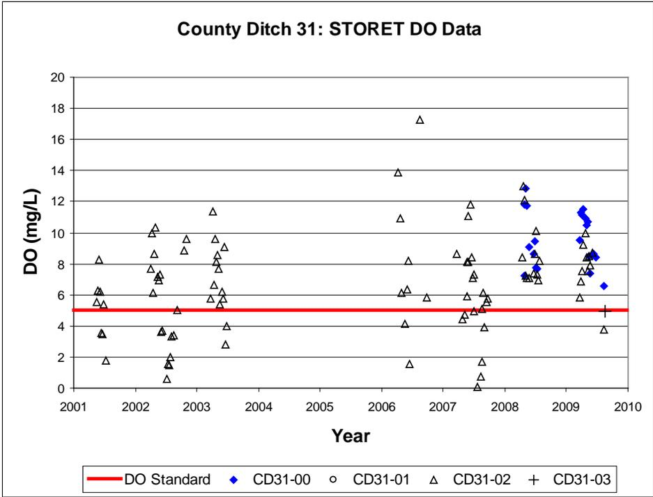
Figure 2.1 Dissolved oxygen data from STORET for all CD31 Stations.
