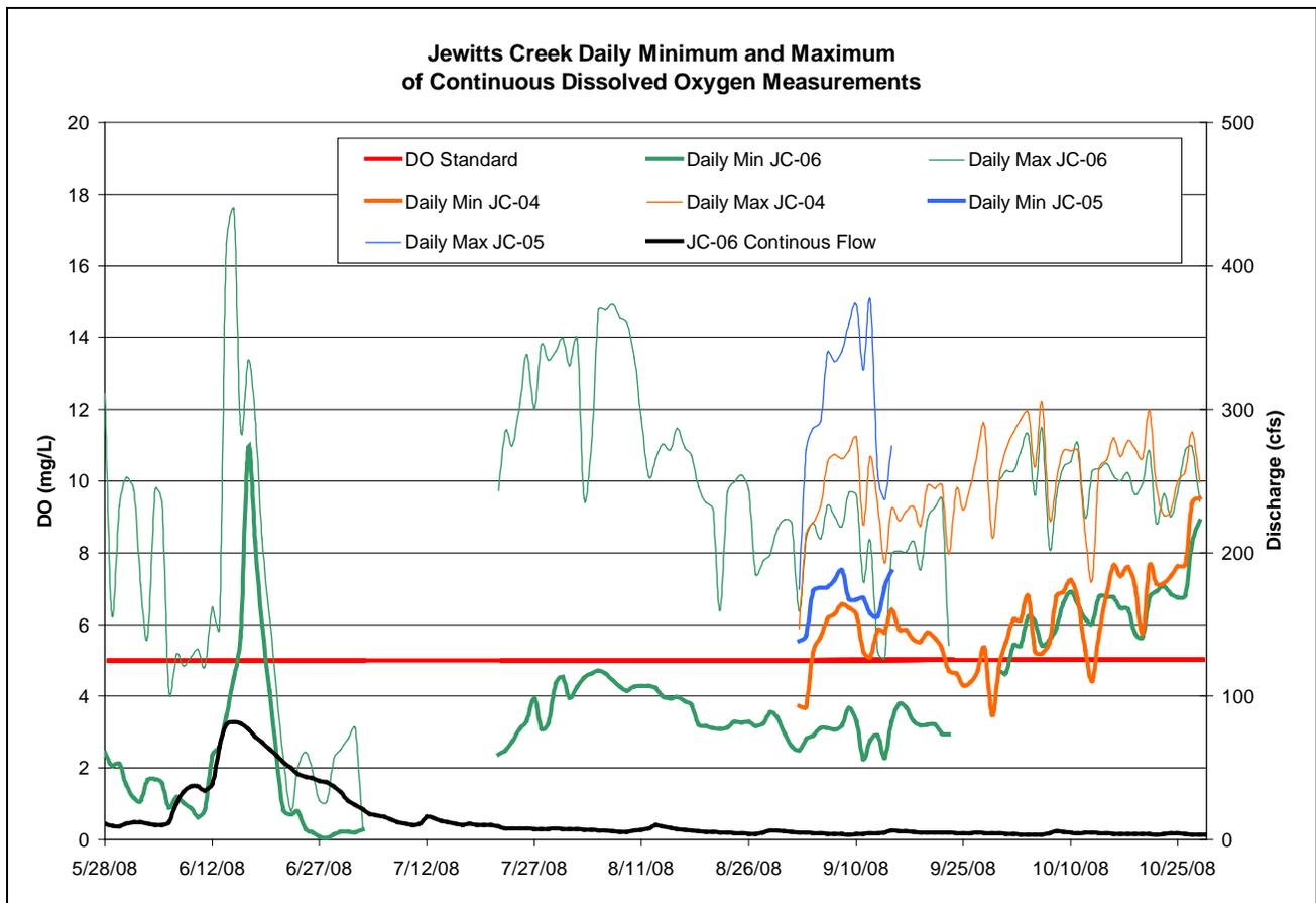
**Figure 2.4** Daily statistics of continuous dissolved oxygen and flow data collected in 2008.
