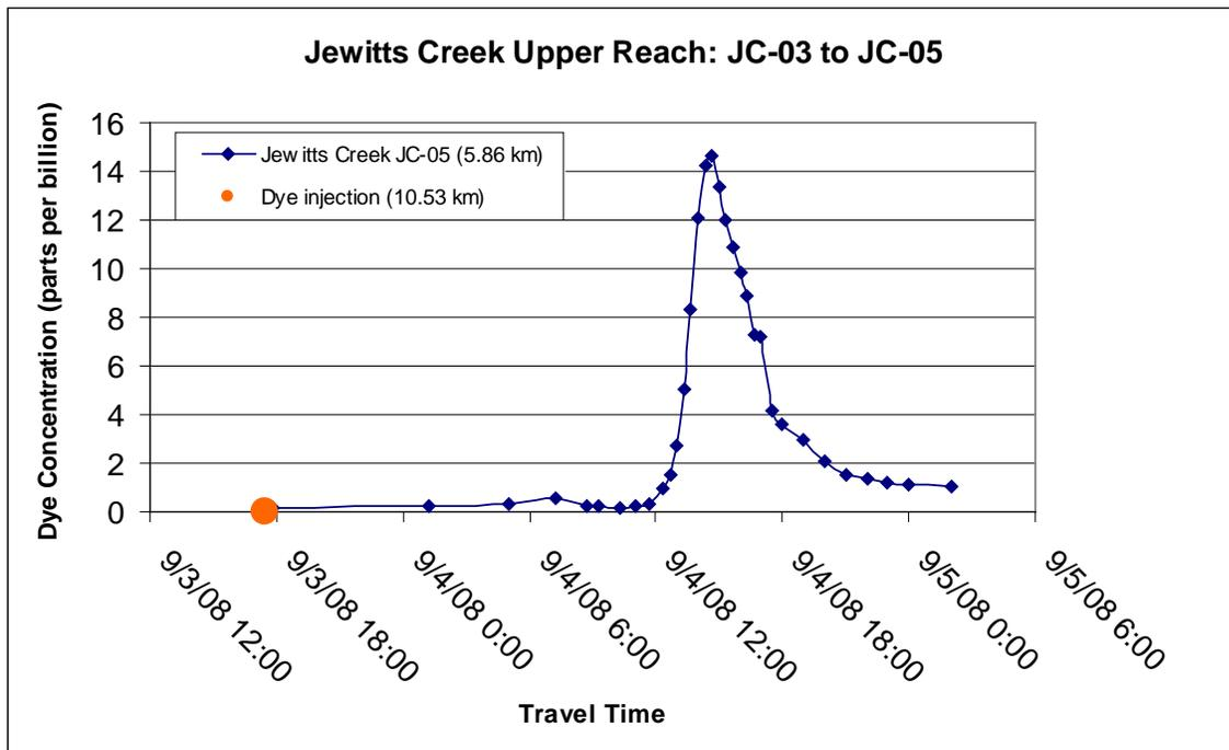
**Figure 4.1** Dye concentration measurements for station JC-05.
