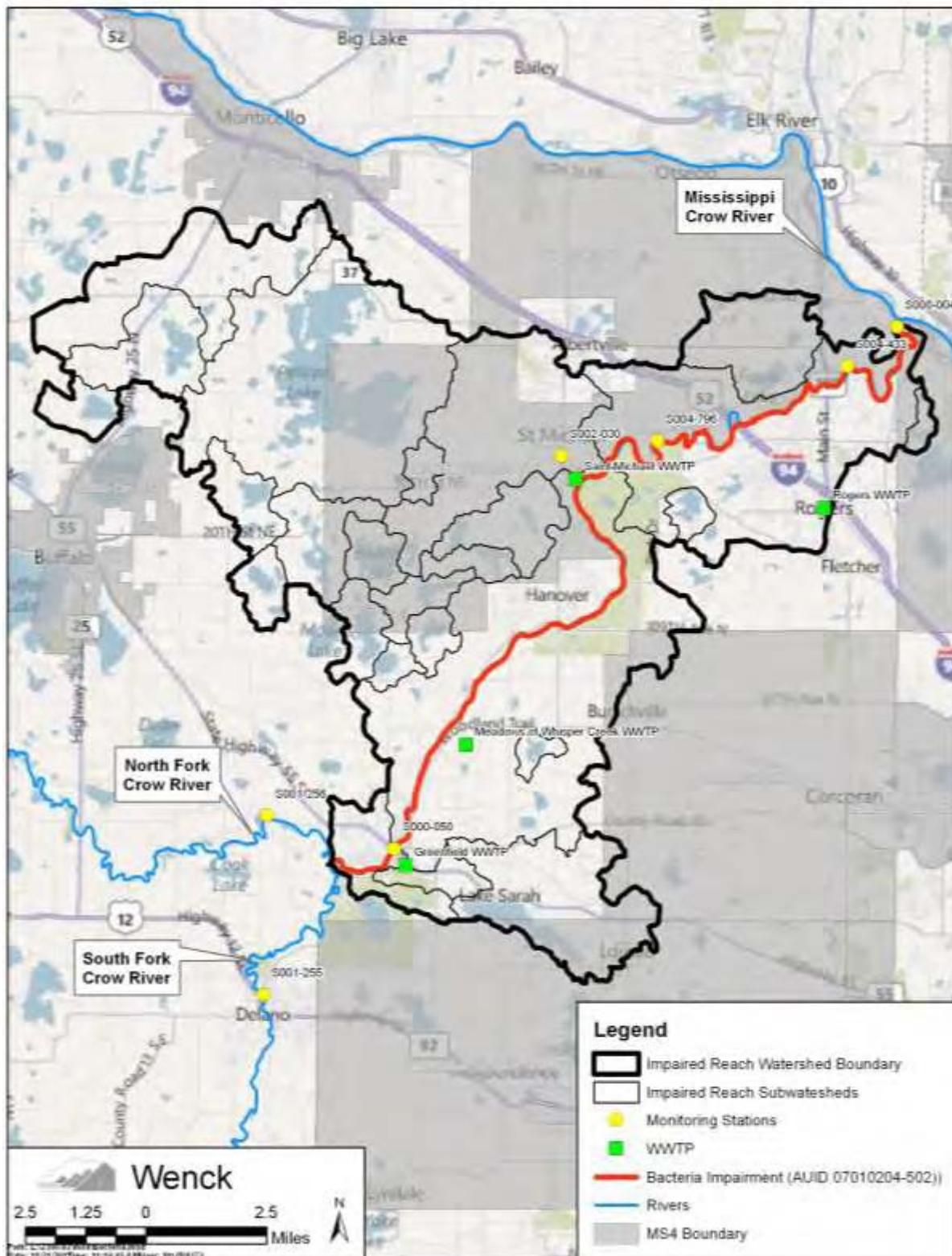
Figure 2.1. Lower Crow River *E. coli* impaired reach watershed, sampling locations and wastewater treatment facilities.
