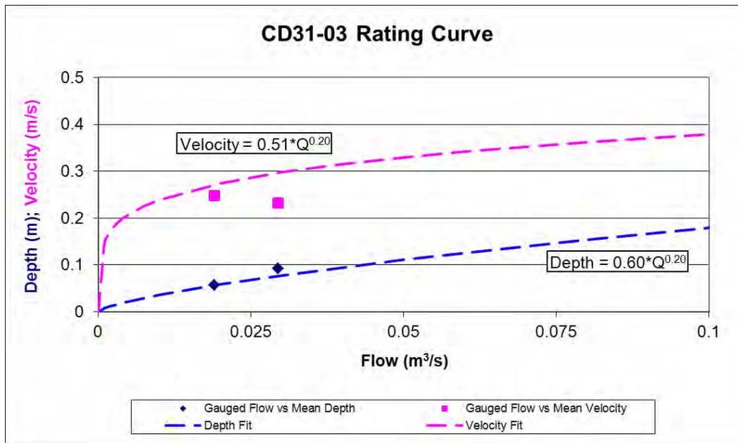
Figure 3.3 Hydraulic rating curve plot for gauging station CD31-03.
