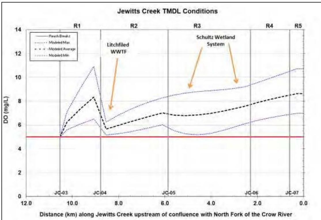
Figure 4.12. Jewitts Creek TMDL scenario QUAL2K model run.
