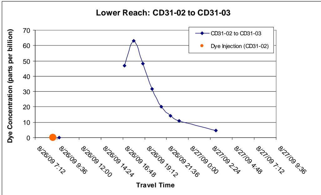
Figure 4.2 Dye concentration measurements from station CD31-03.
