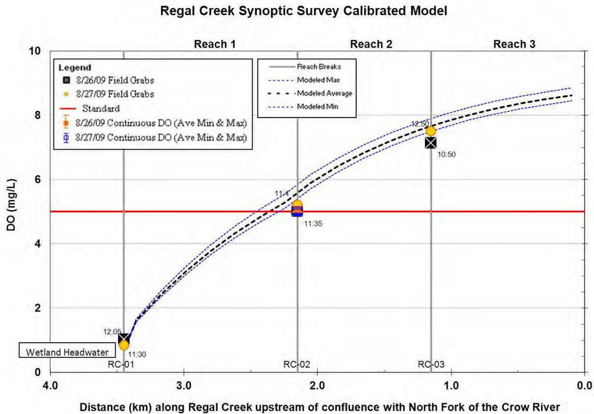
Figure 5.1 Regal Creek calibrated dissolved oxygen longitudinal profile.
