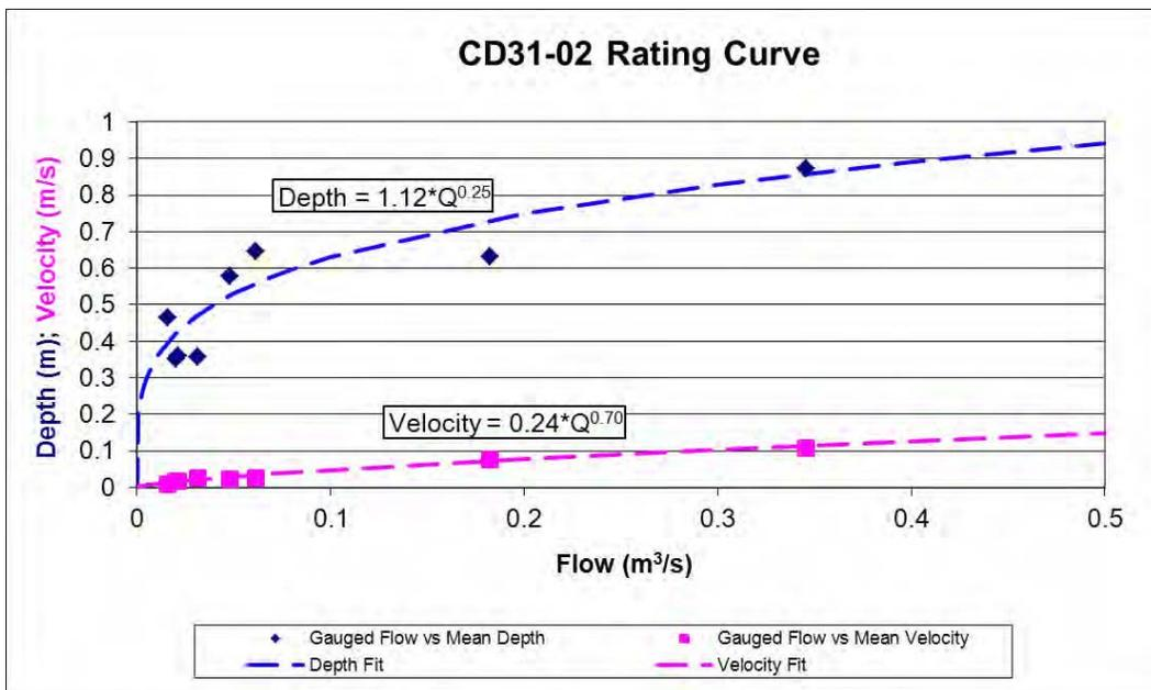
**Figure 3.2** Hydraulic rating curve plot for gauging station CD31-02.
