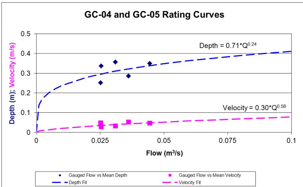
Figure 3.3 Hydraulic rating curve plot for gauging stations GC-04 and GC-05.
