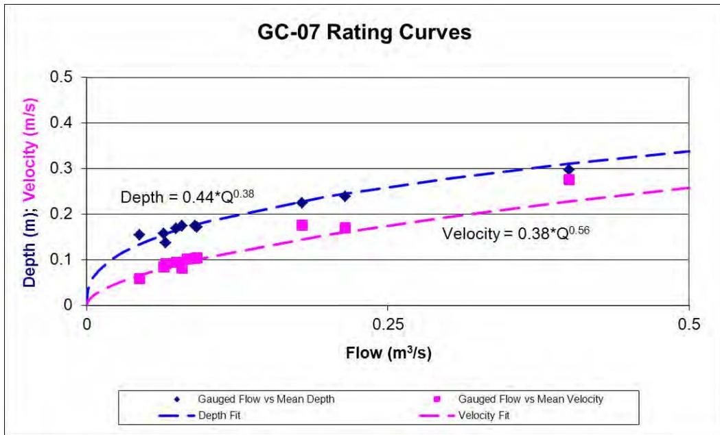
Figure 3.4 Hydraulic rating curve plot for gauging station GC-07.
