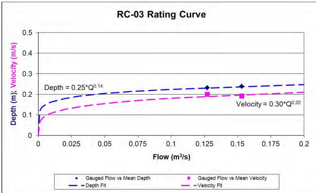
Figure 3.3 Hydraulic rating curve plot for gauging station RC-03.
