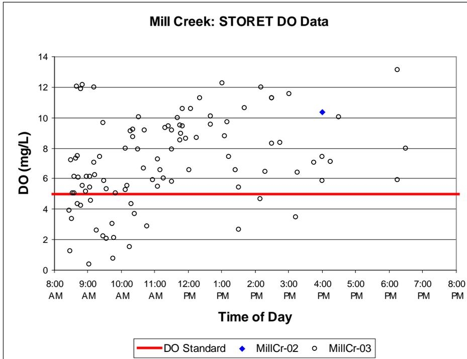
**Figure 2.3** Dissolved oxygen data from STORET for all Mill Creek stations by hour, regardless of year and month. No data was collected between 8:00 pm and 8:00 am.
