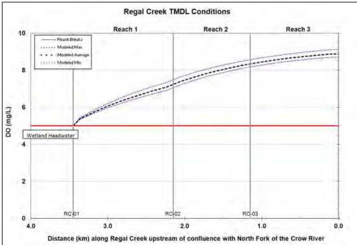
Figure 4.16. Regal Creek TMDL scenario QUAL2K model run.
