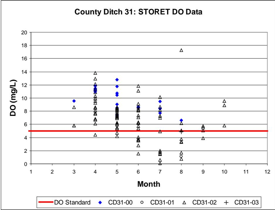
Figure 2.2 Dissolved oxygen data from STORET for all CD31 stations by month, regardless of year.
