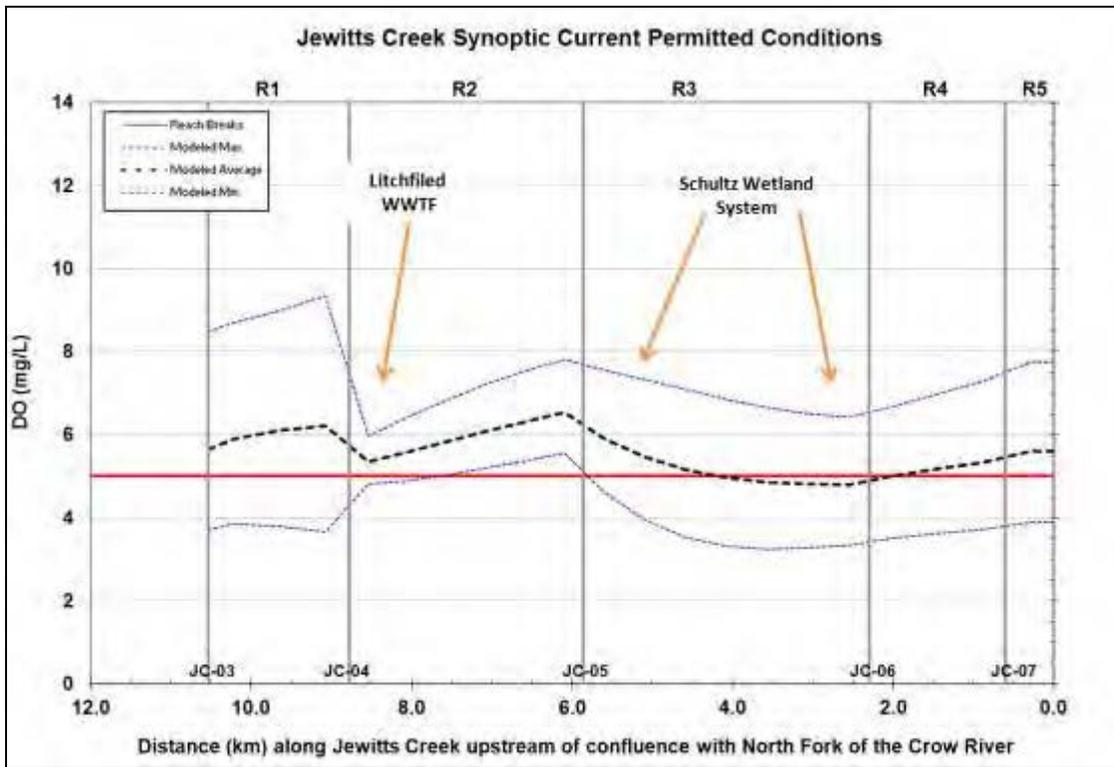
Figure 4.11. Jewitts Creek current permitted conditions QUAL2K model run.
