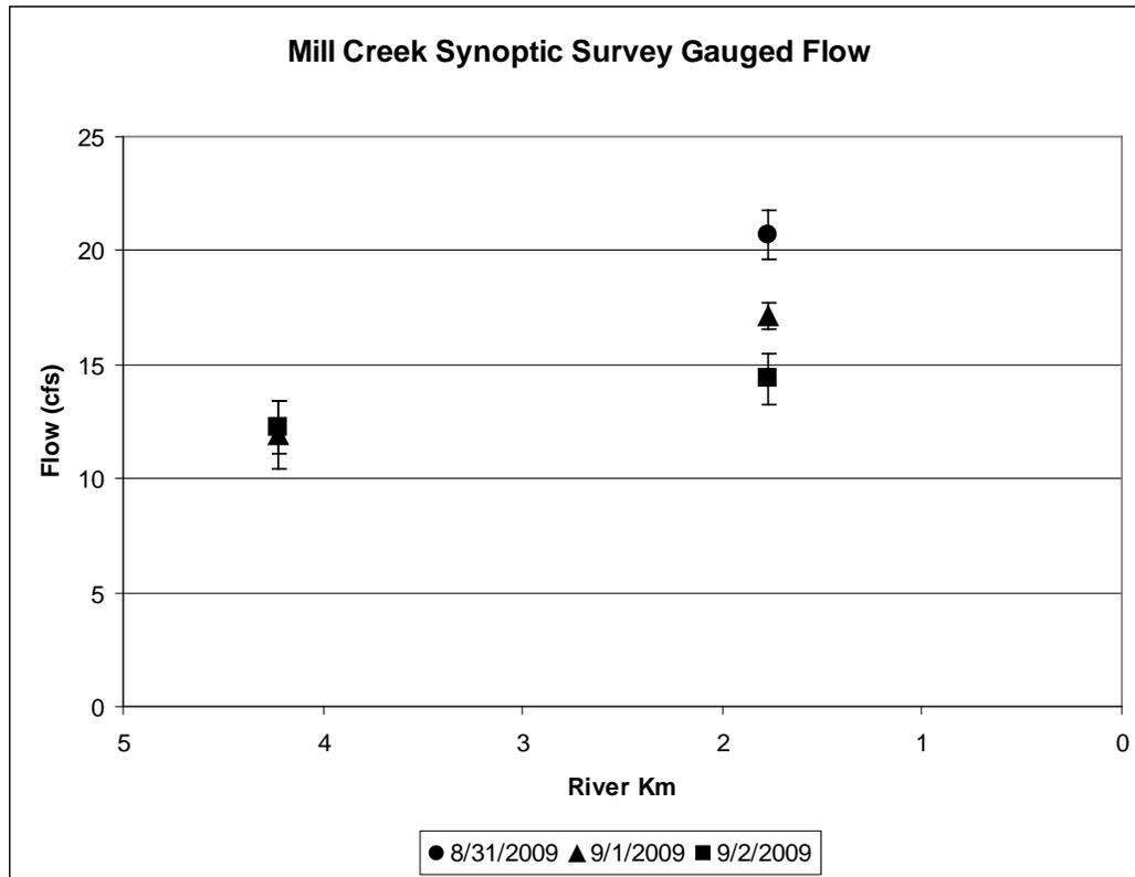
**Figures 4.2** Gauged flows by river kilometer for the Mill Creek synoptic survey. Error bars represent estimated uncertainty of the Flow-Tracker field measurement.
