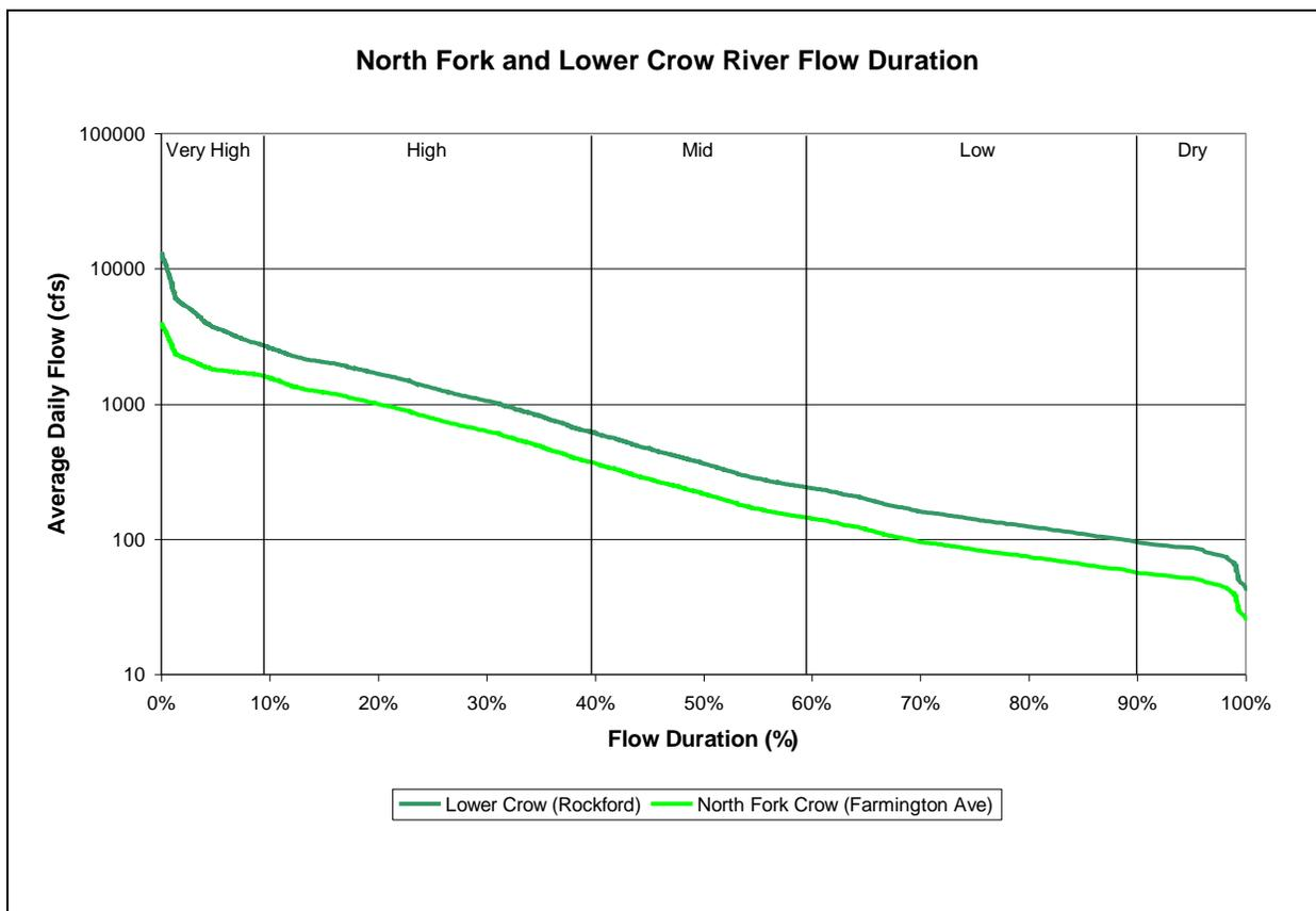
Figure 3.3. Flow duration for North Fork and Lower Crow River monitoring stations.
