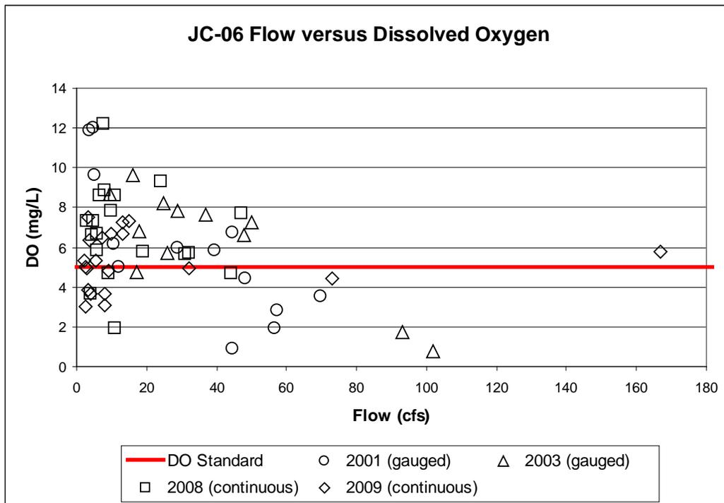
Figure 2.5 Dissolved oxygen compared to gauged and continuous flow measurements.
