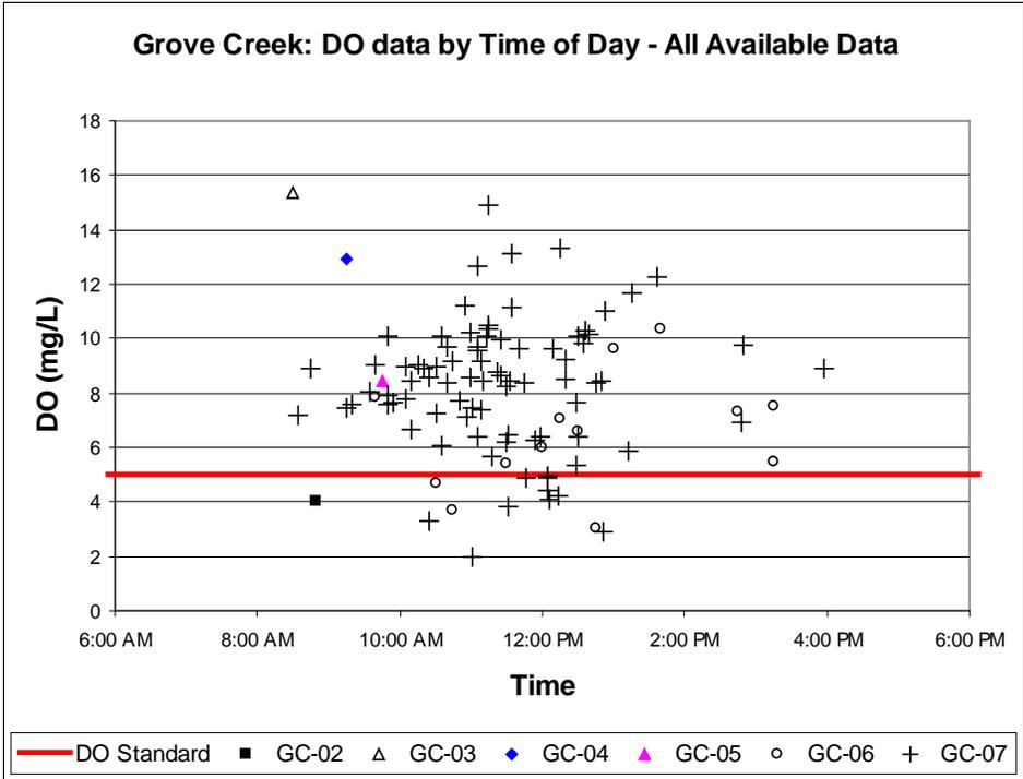
**Figure 2.3:** Dissolved oxygen data from STORET for all Grove Creek Stations by hour, regardless of year and month. No data was collected prior to 8:00 am or after 4:30 pm.
