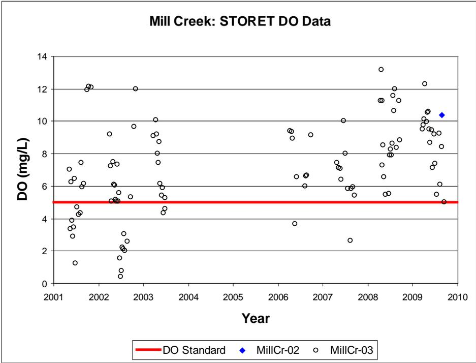
**Figure 2.1** Dissolved oxygen data from STORET for all Mill Creek Stations
