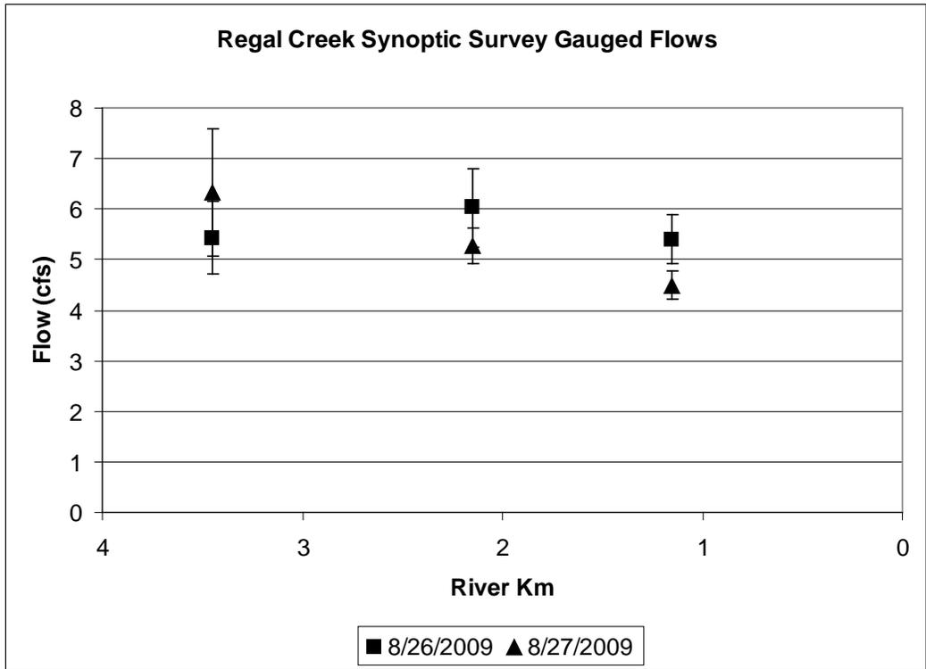
**Figures 4.2** Gauged flows by river kilometer for the Regal Creek synoptic survey. Error bars represent estimated uncertainty of the Flow-Tracker field measurement.
