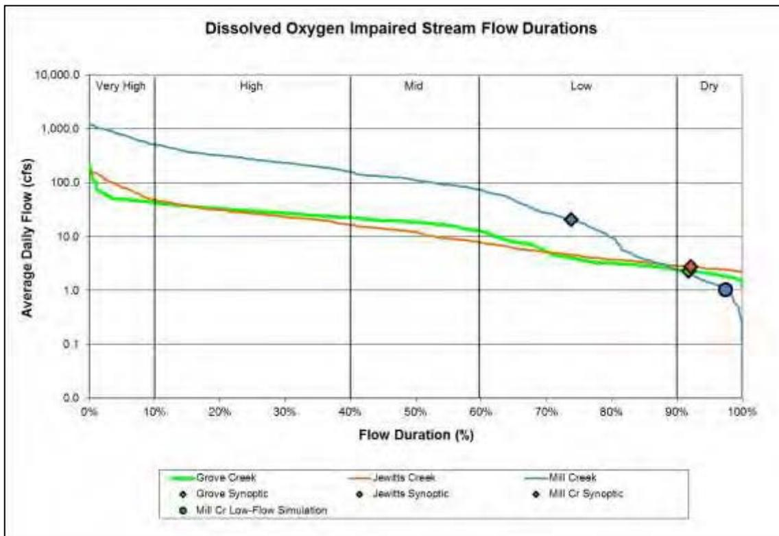
**Figure 4.8. Dissolved oxygen impaired reach 3-year flow duration curves (2008-2010).**
