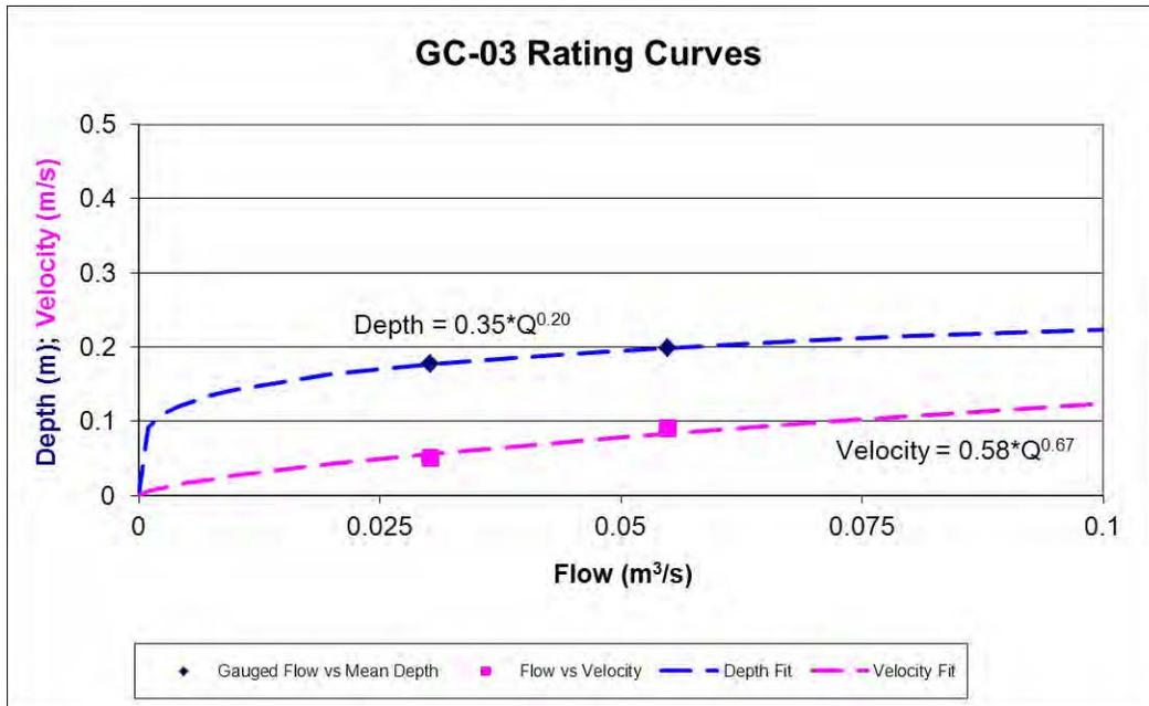
Figure 3.2 Hydraulic rating curve plot for gauging stations GC-03.
