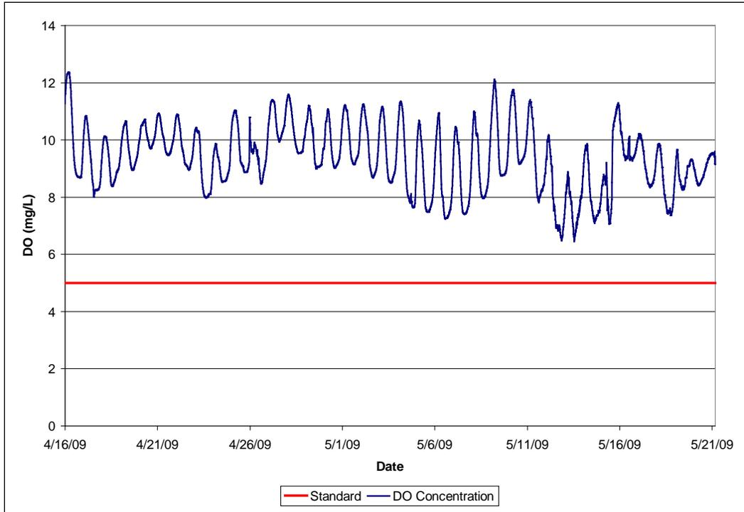
**Figure 2.4** Continuous DO measurements at Station S002-030 from 4/16/09 to 5/21/2009 (preliminary data supplied by the MPCA).
