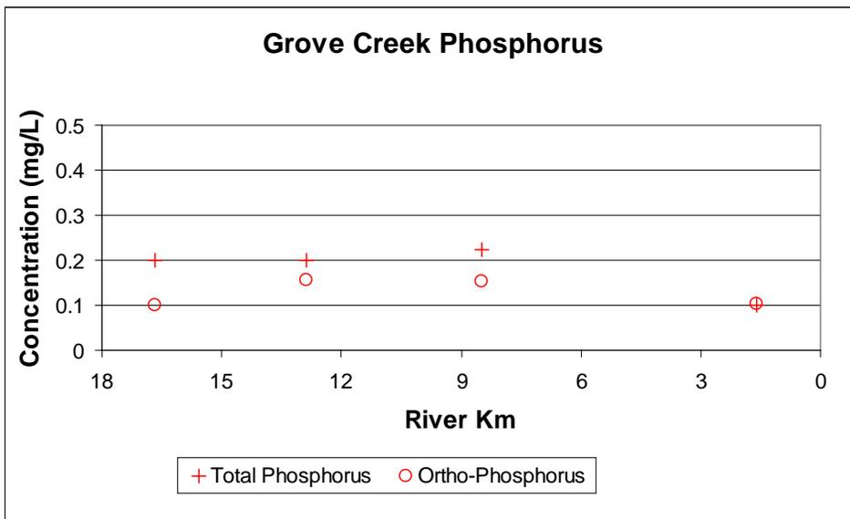
Figures 4.5 September 3, 2008 synoptic survey water quality lab results for Grove Creek.
