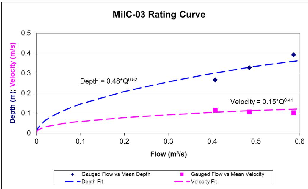
Figure 3.2 Hydraulic rating curve plot for gauging station MilC-03.
