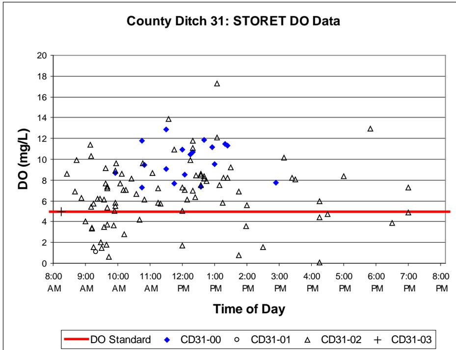
**Figure 2.3** Dissolved oxygen data from STORET for all CD31 stations by hour, regardless of year and month. No measurements were reported between 8:00pm and 8:00 am.
