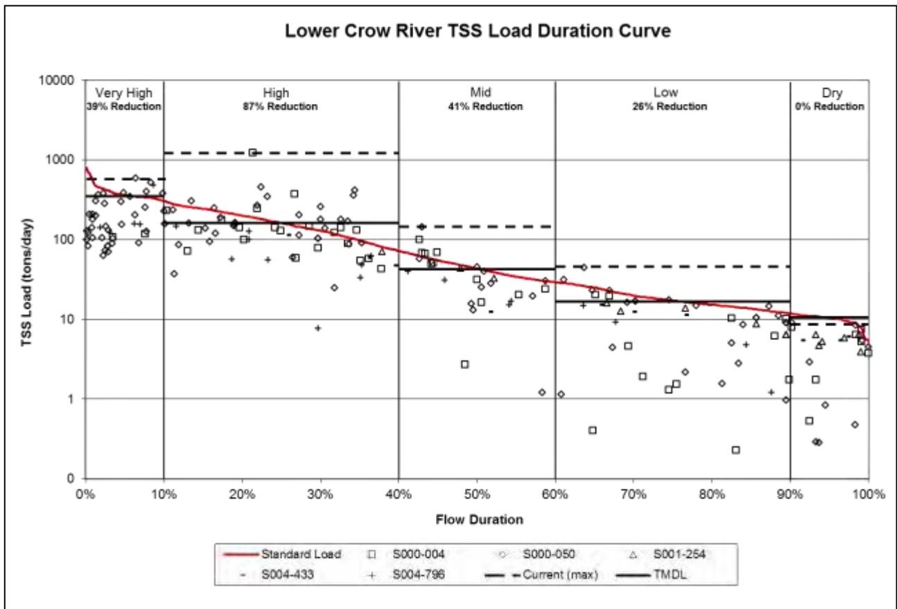
Figure 3.5. Lower Crow River Impaired Reach (07010204-502) TSS Load Duration Curve and necessary TSS reductions to meet TMDL.
