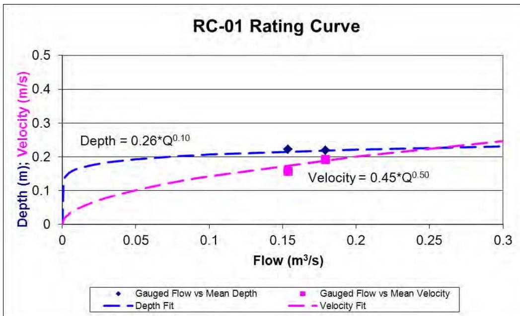
Figure 3.1 Hydraulic rating curve plot for gauging station RC-01.
