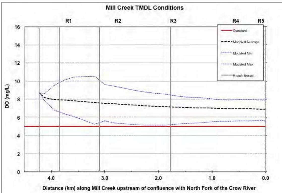
Figure 4.14. Mill Creek TMDL scenario QUAL2K model run.
