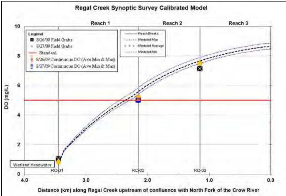
Figure 4.15. Regal Creek current conditions QUAL2k model run.
