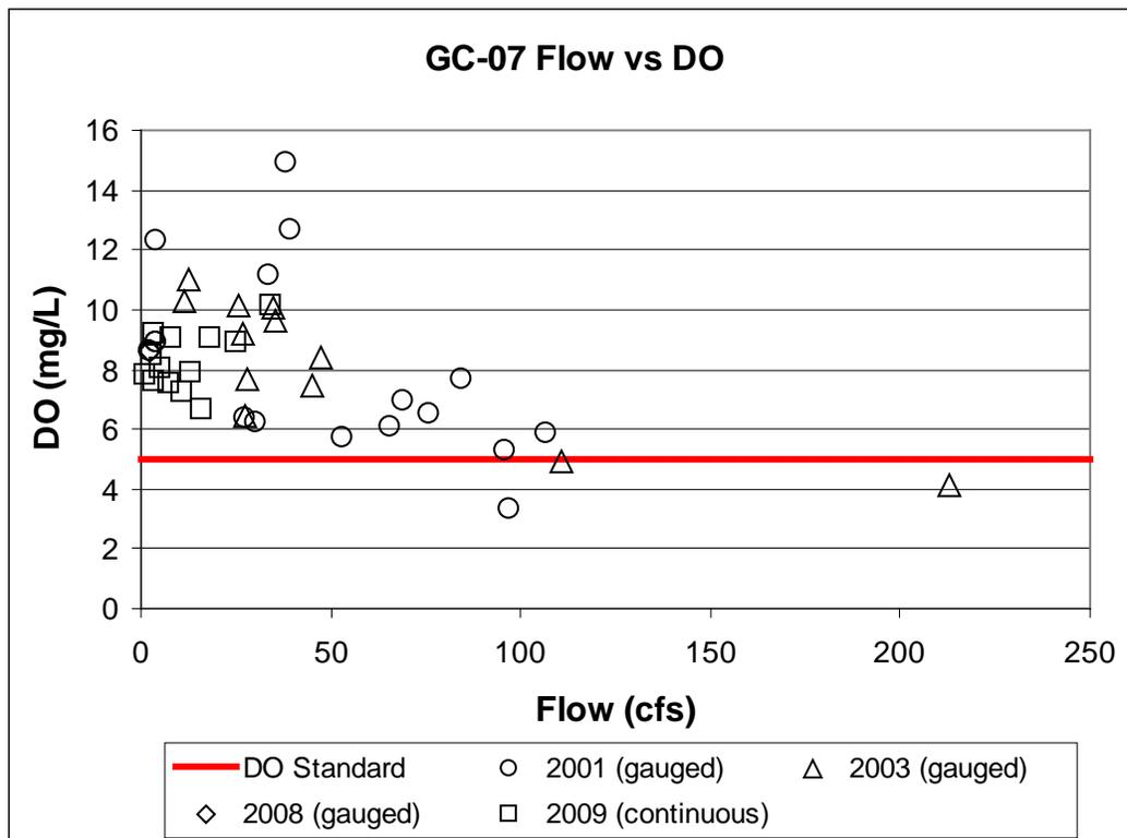
**Figure 2.5** Dissolved oxygen compared to gauged and continuous flow measurement.
