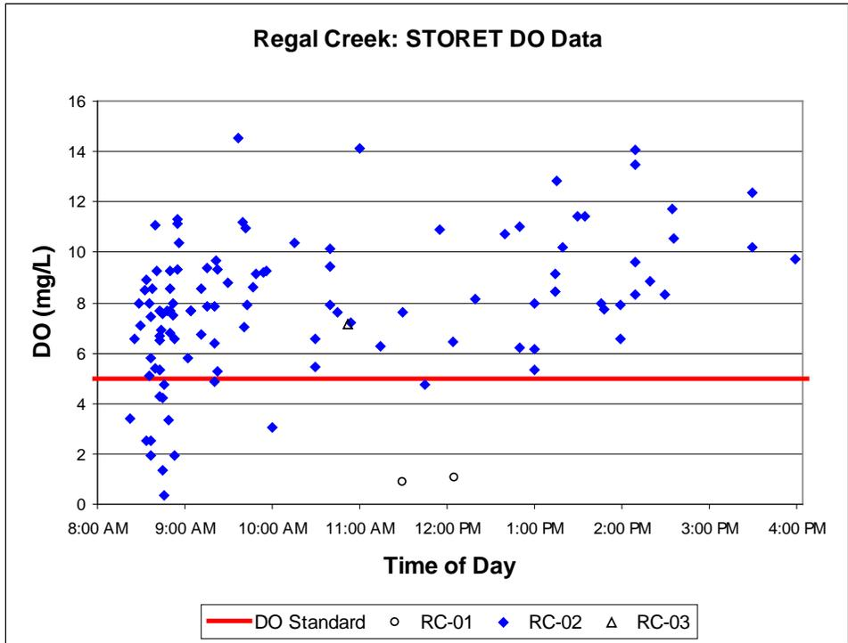
Figure 2.3 Dissolved oxygen data from STORET for all Regal Creek Stations by hour, regardless of year and month.
