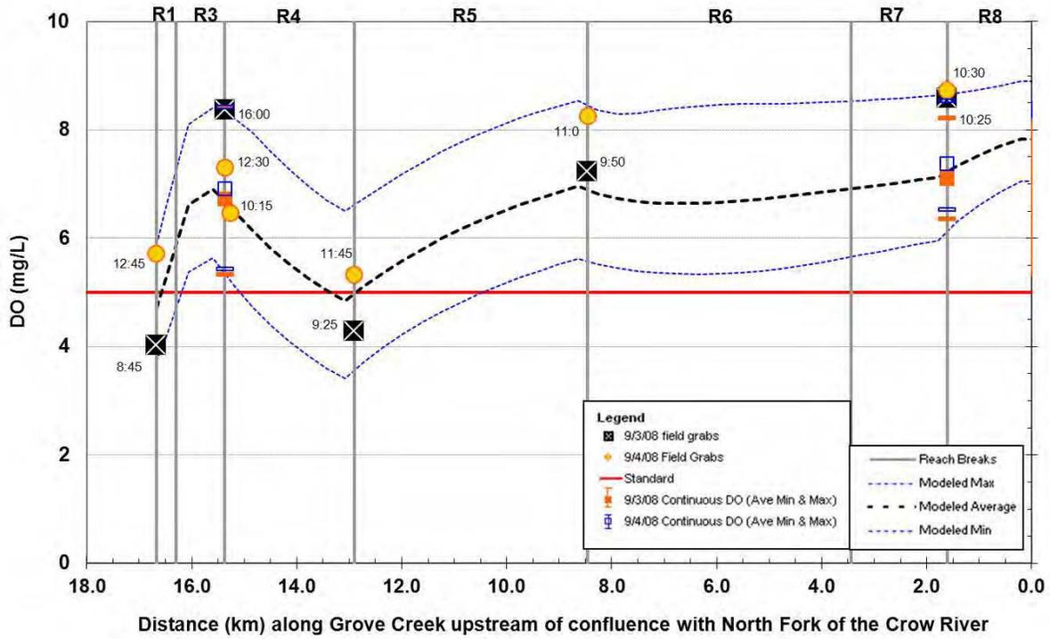
Figure 5.1 Grove Creek calibrated dissolved oxygen longitudinal profile.
