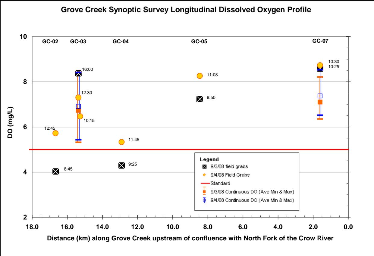
Figure 4.10 Dissolved oxygen observations during the September 2008 synoptic survey.
