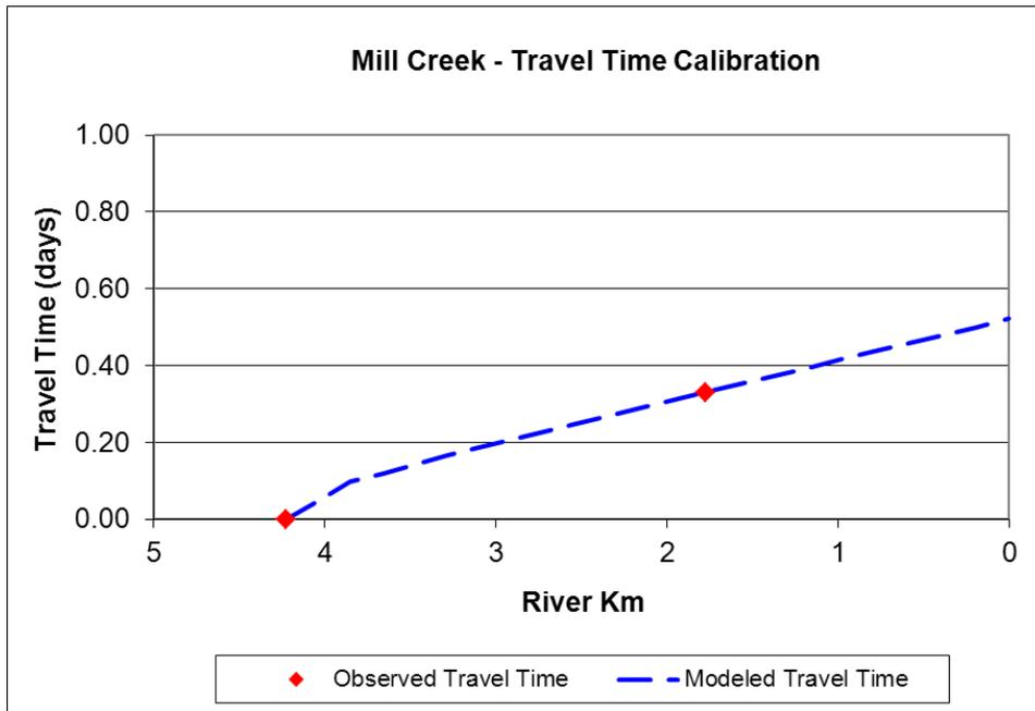
Figure 3.4 Mill Creek travel time calibration.
