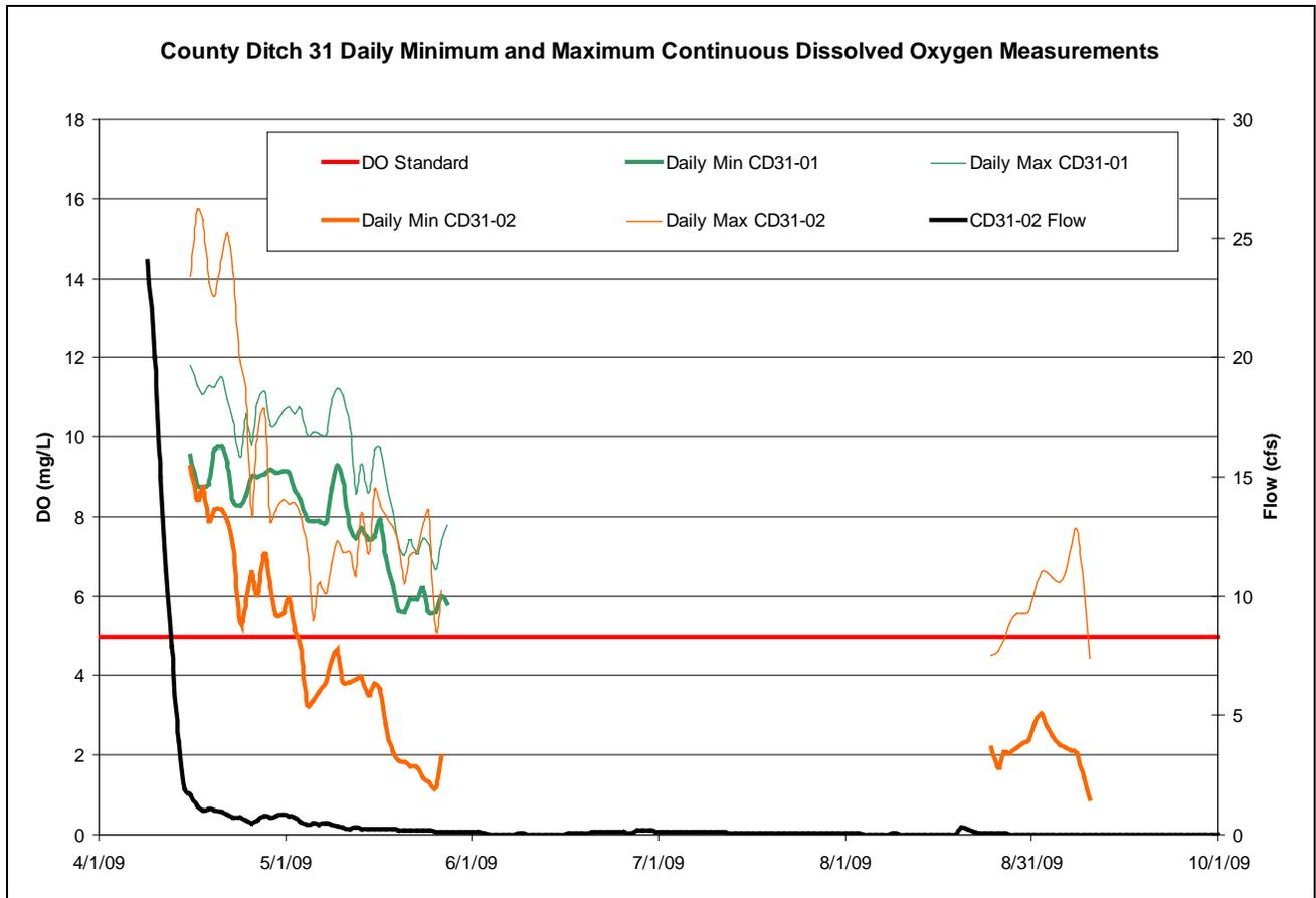
Figure 2.4 Statistics of continuous dissolved oxygen data collected in 2008.
