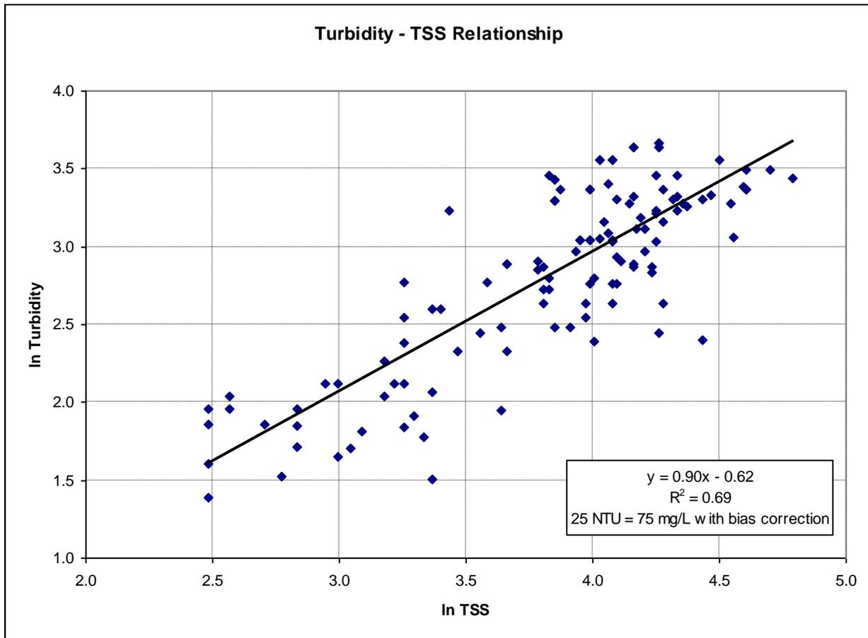
**Figure 3.2. Turbidity/Total Suspended Solids Relationship for three sites within the North Fork Crow and Lower Crow River Watershed.**
