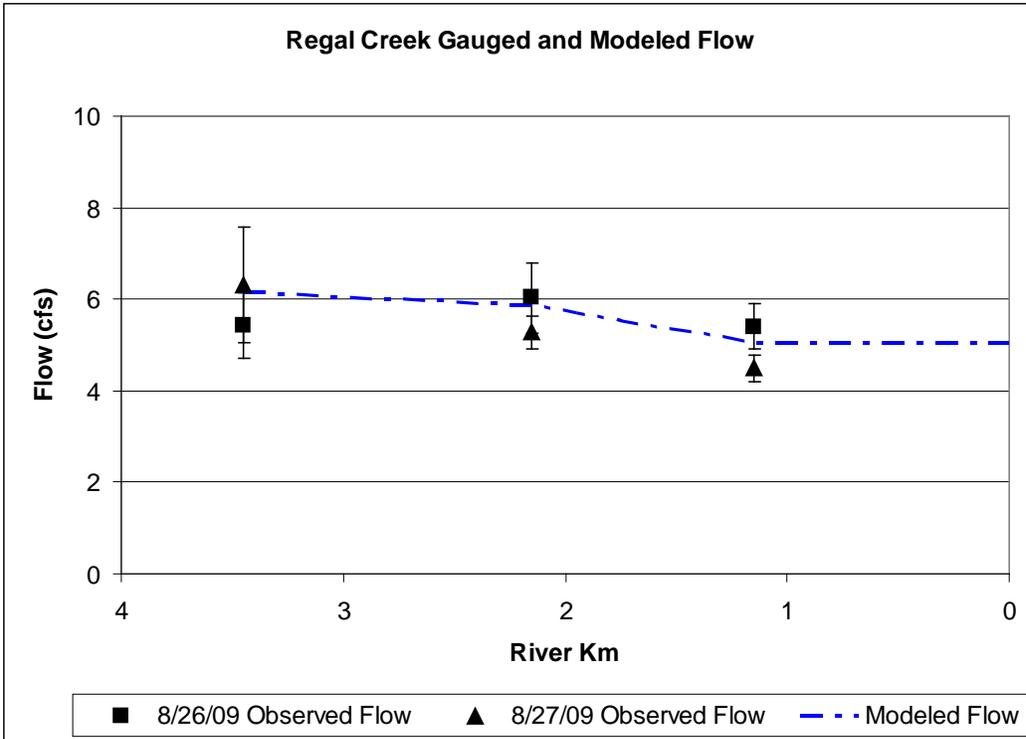
**Figure 3.4** Final Regal Creek Flow calibration with diffuse inflows/abstractions. Error bars on observed measurements represent estimated uncertainty of the Flow-Tracker field measurement.
