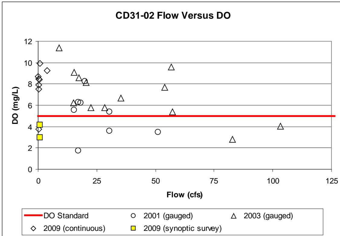
**Figure 2.5** CD31-02 dissolved oxygen compared to gauged and continuous flow measurement.
