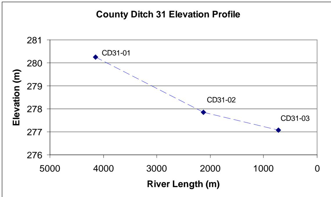
Figure 2.2 Survey elevations used to estimate reach slopes for County Ditch 31.
