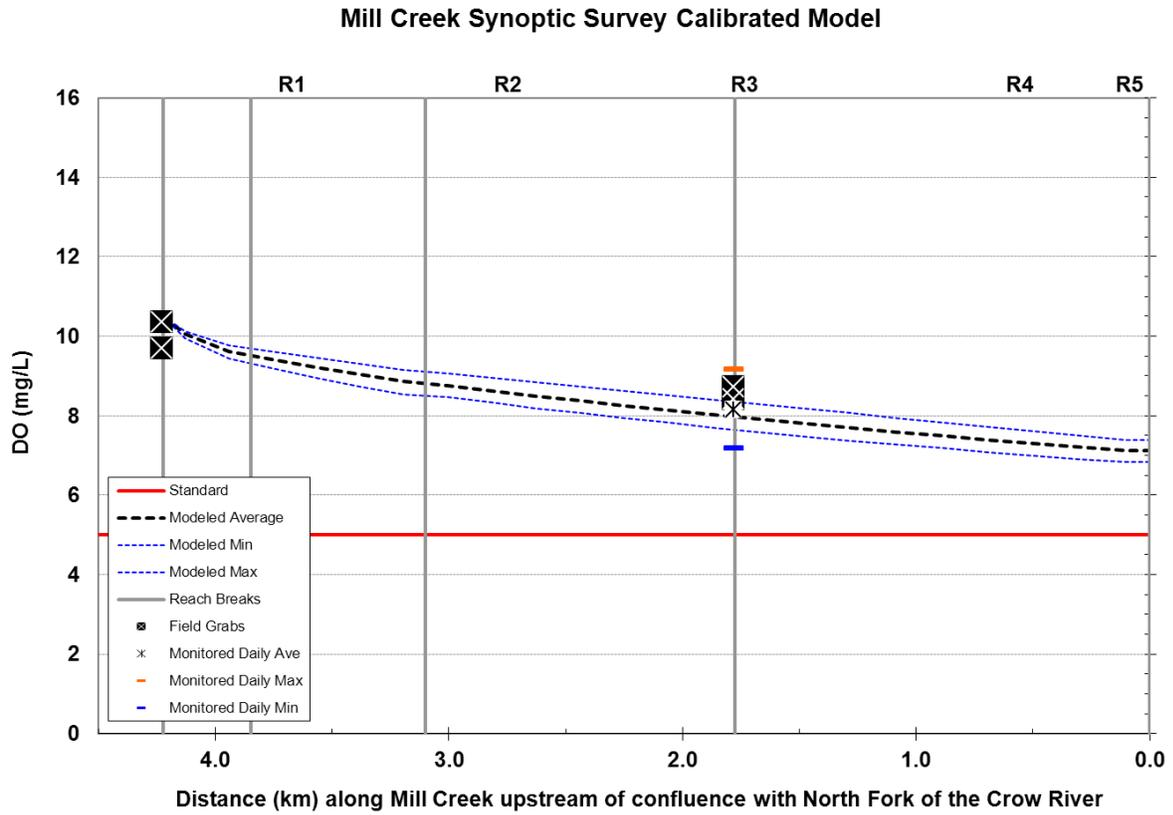
Figure 5.1 Mill Creek calibrated dissolved oxygen longitudinal profile.
