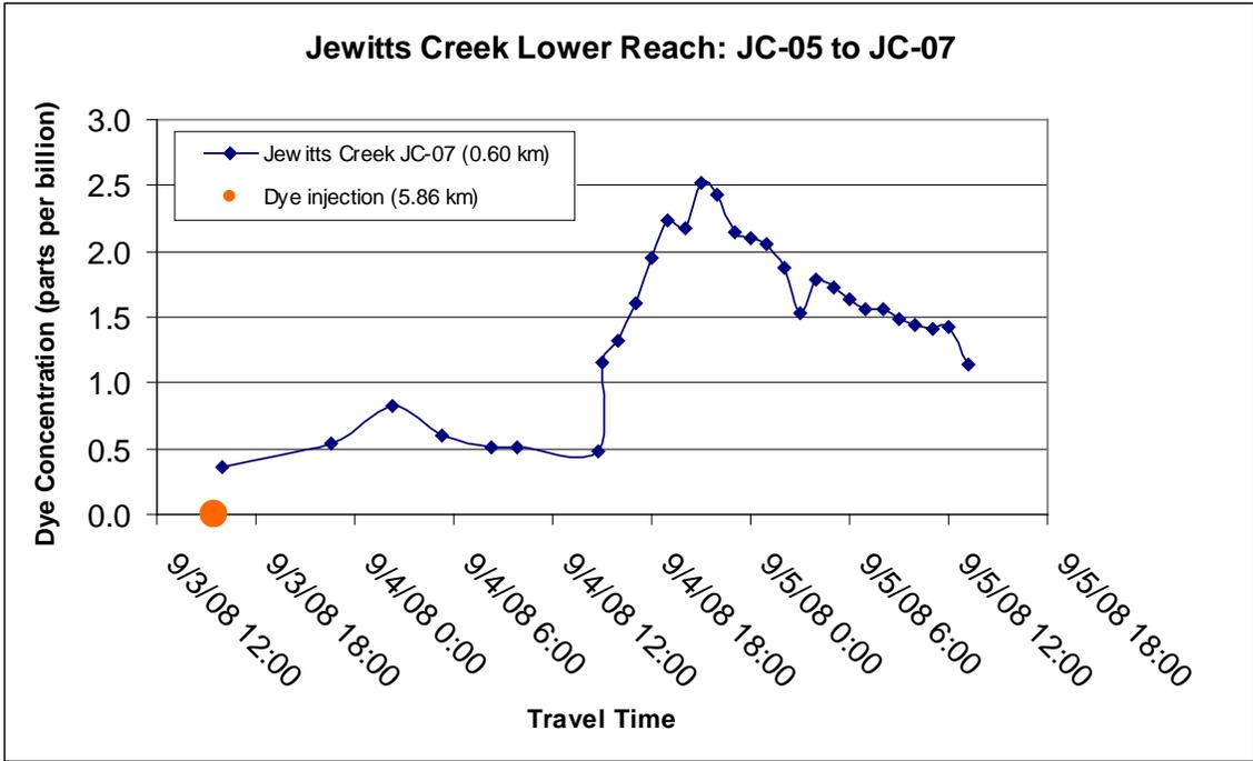
Figure 4.2 Dye concentration measurements for station JC-07
