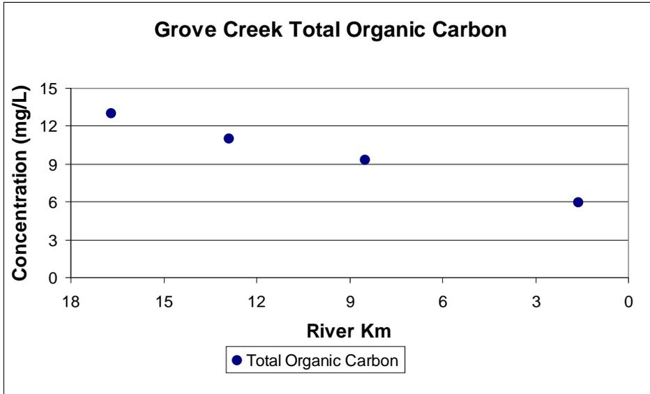
Figures 4.6 September 3, 2008 synoptic survey water quality lab results for Grove Creek.
