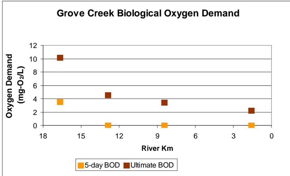
Figures 4.8 September 3, 2008 synoptic survey water quality lab results for Grove Creek.
