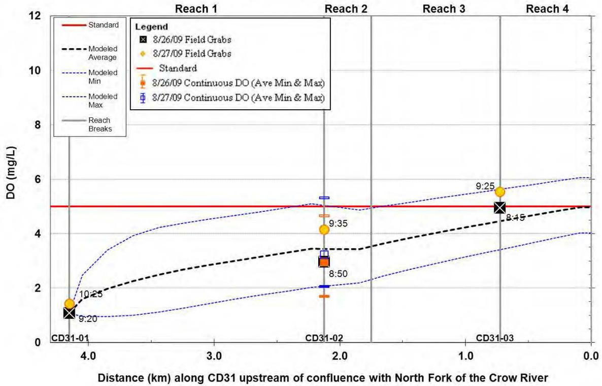
Figure 5.1 CD31 calibrated dissolved oxygen longitudinal profile.
