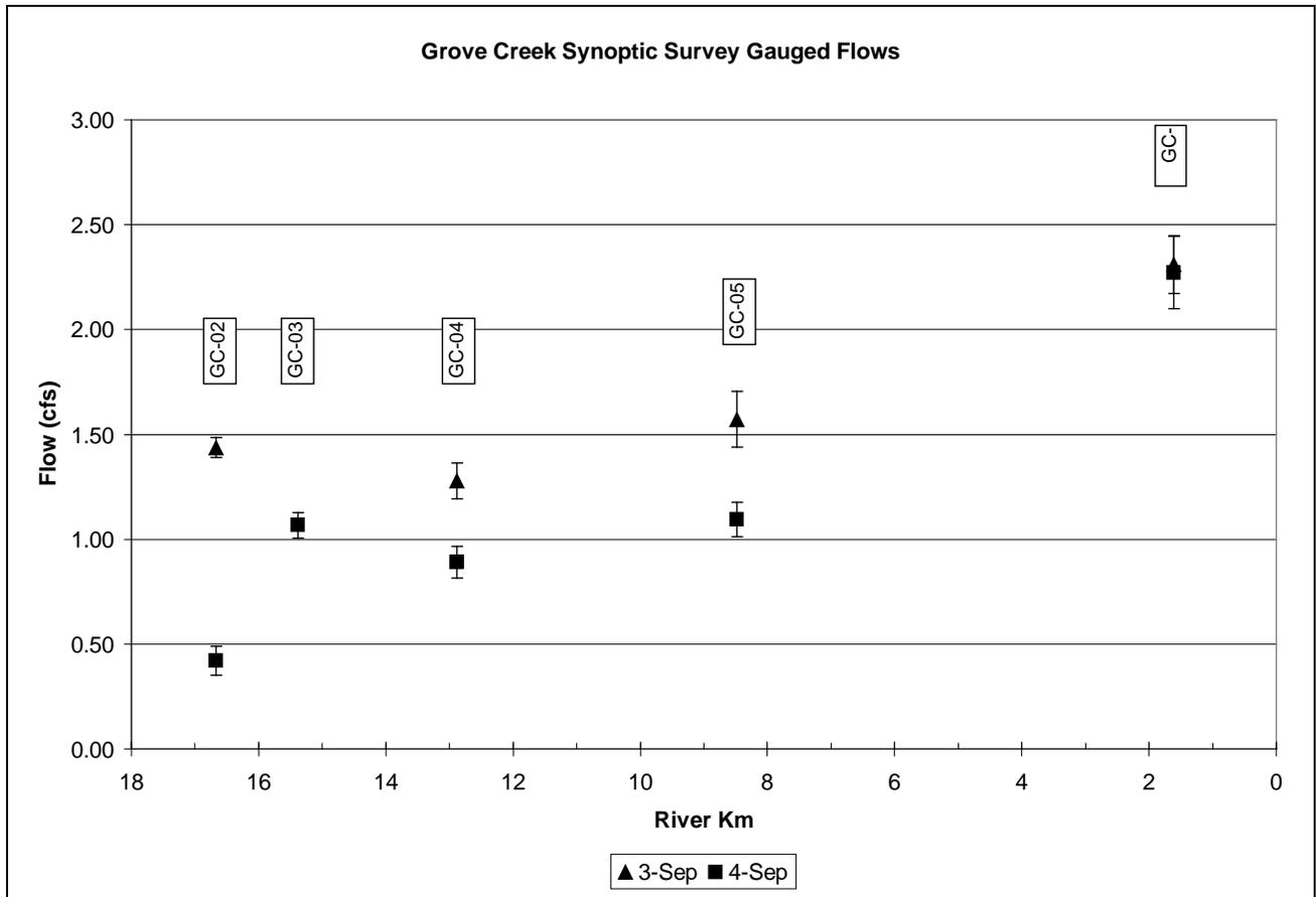
**Figures 4.3** Gauged flows by river kilometer for the Grove Creek survey. Error bars represent estimated uncertainty of the Flow-Tracker field measurement.
