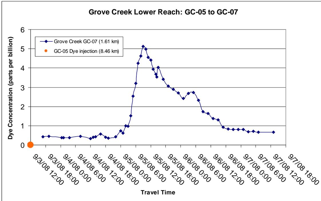
Figure 4.2 Dye concentration measurements from station GC-07.
