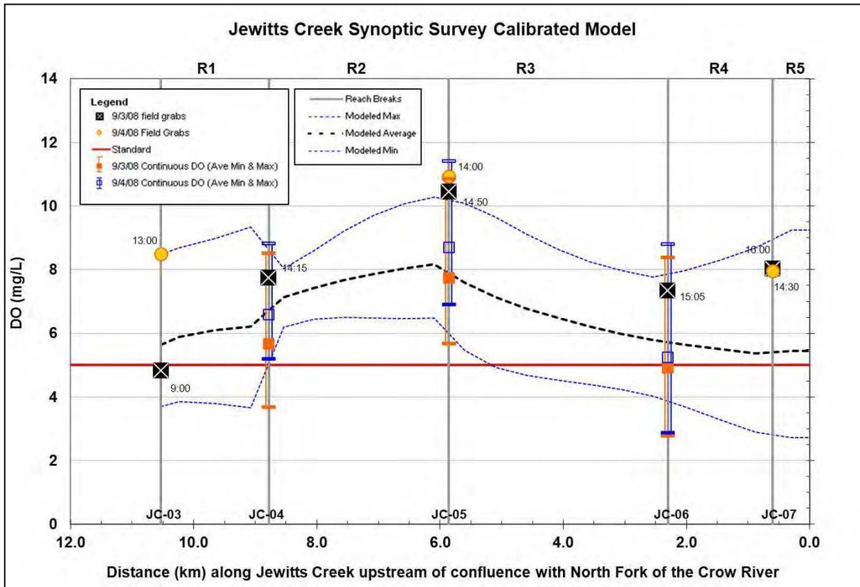
Figure 5.1 Jewitts Creek calibrated dissolved oxygen longitudinal profile.
