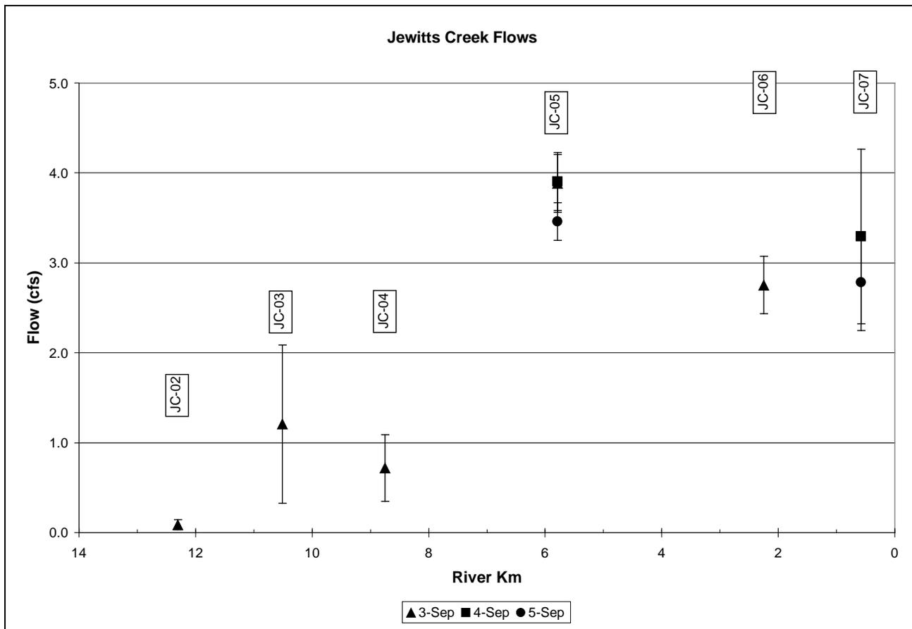
**Figures 4.3** Gauged flows by river kilometer recorded during the Jewitts Creek synoptic survey. Error bars represent estimated uncertainty of the Flow-Tracker field measurement.
