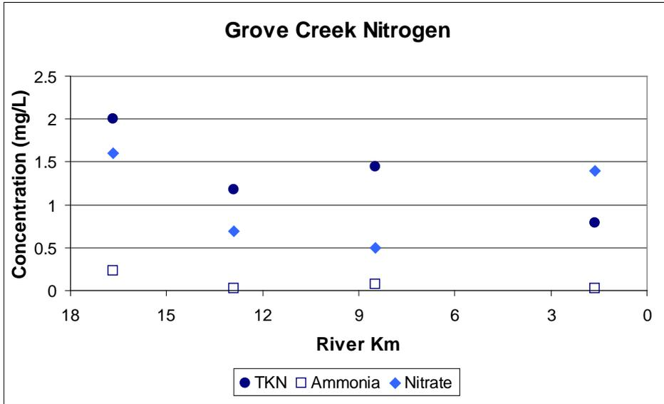
Figures 4.4 September 3, 2008 synoptic survey water quality lab results for Grove Creek.
