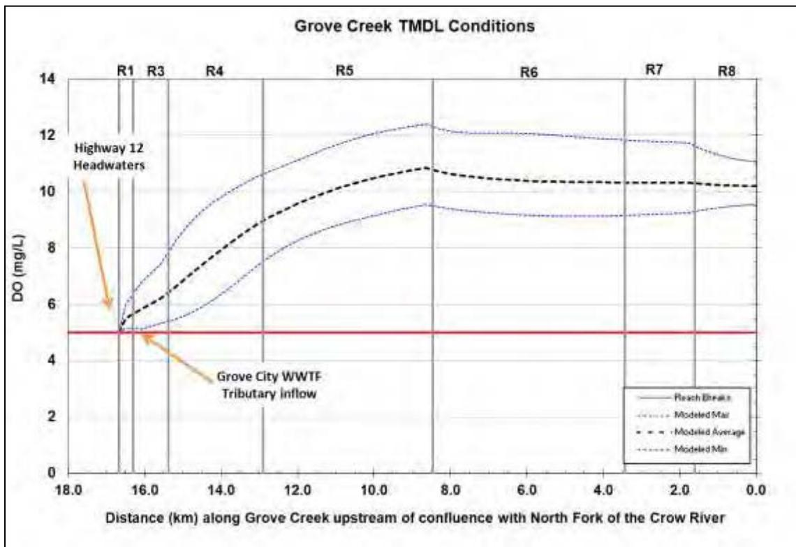
Figure 4.10. Grove Creek TMDL scenario QUAL2K model run.
