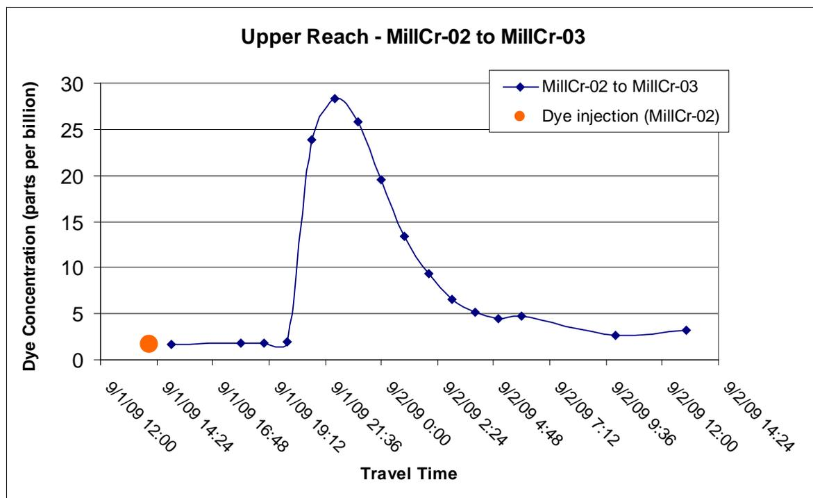
**Figure 4.1** Dye concentration measurements from station MillCr-03
