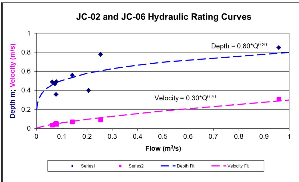
Figure 3.2 Hydraulic rating curve plot for gauging stations JC-02 and JC-06.
