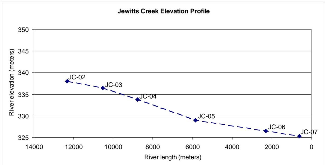
**Figure 2.2** Longitudinal elevation survey and modeled reach slopes for Jewitts Creek.
