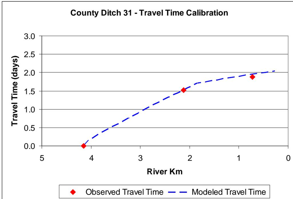
Figure 3.5 CD31 time of travel calibration.
