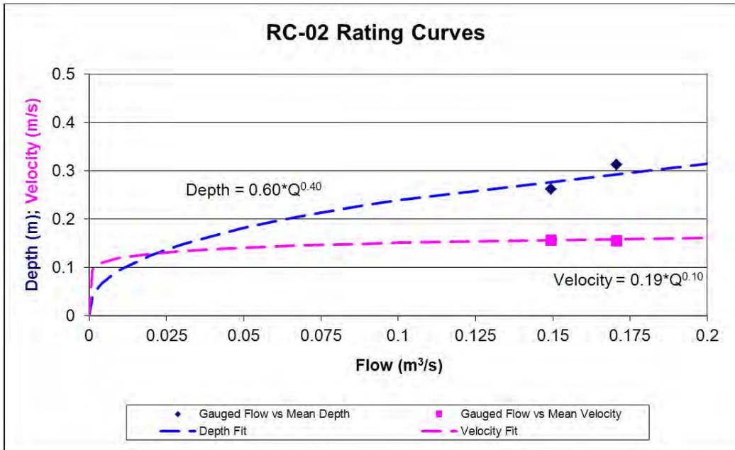
Figure 3.2 Hydraulic rating curve plot for gauging station RC-02.
