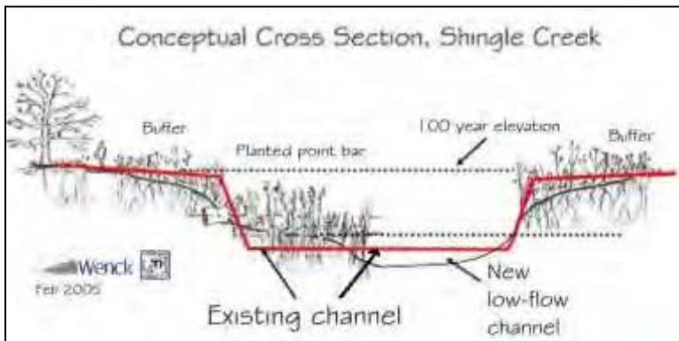
**Figure 5.1. Desirable stream cross section with enhanced habitat and a low-flow channel.**
