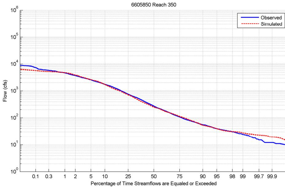
**Figure 8.** Flow-Duration Curve Example.
