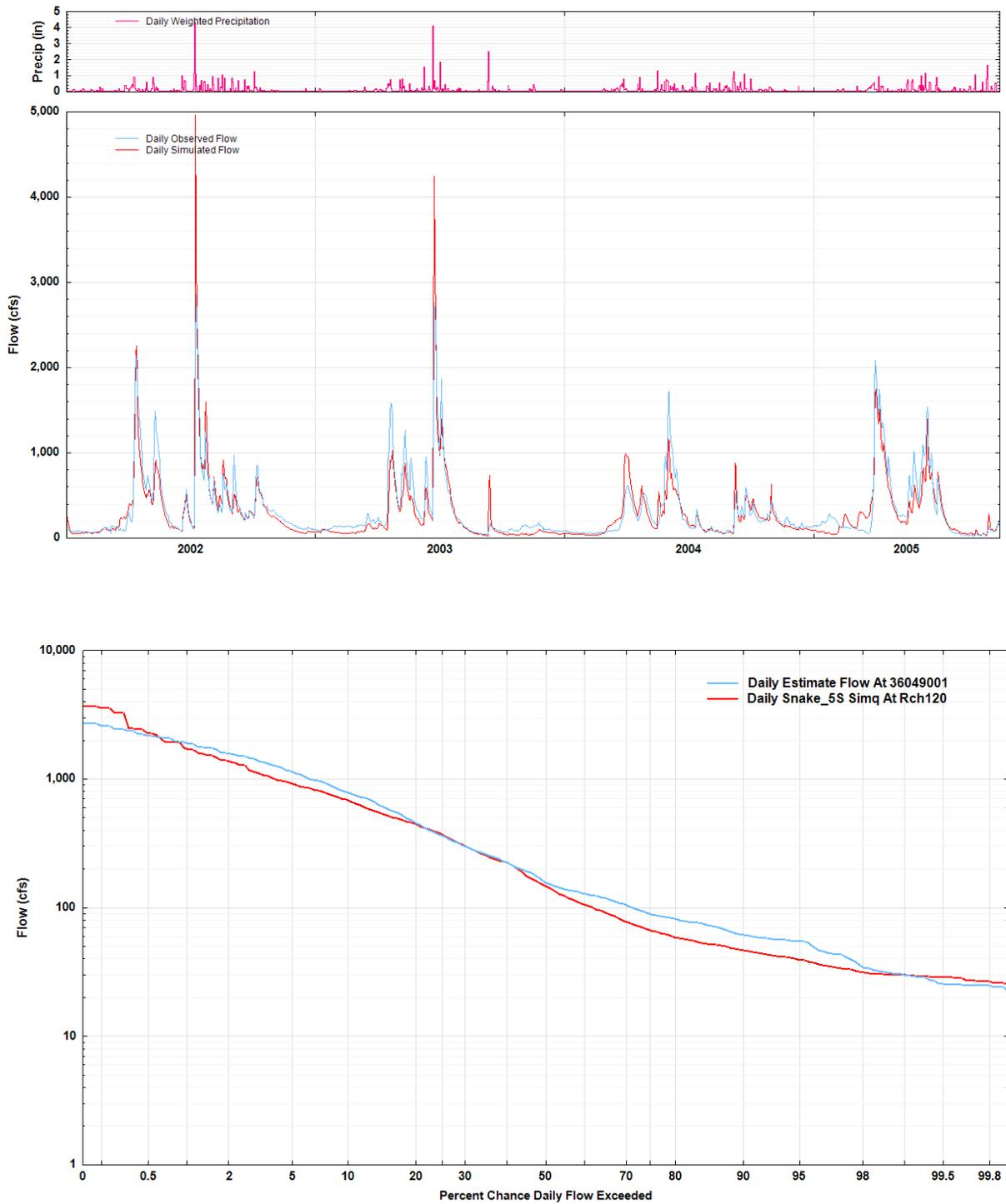
**Figure 2-9.** Observed and Simulated Flow Hydrograph and Frequency-Duration Curve at the Minnesota Pollution Control Agency Gage H36049001.
