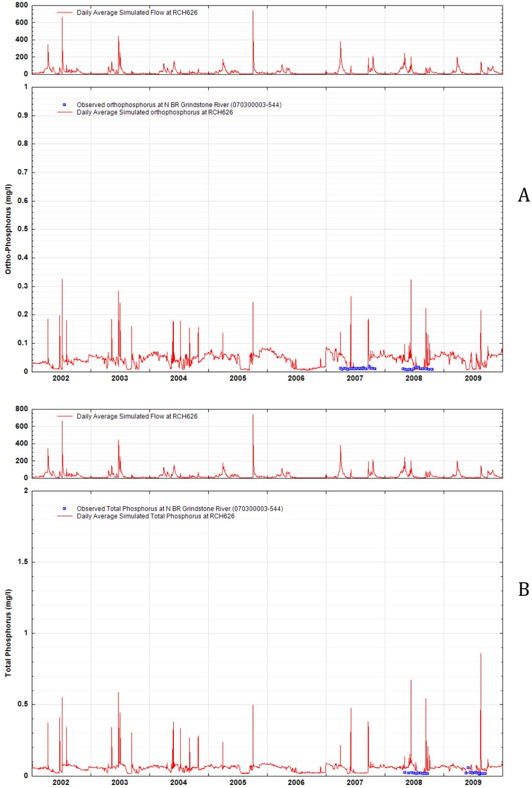
**Figure 4-15.** Observed and Daily Average Simulated (a) Ortho-Phosphorus as Phosphorus and (b) Total Phosphorus at N BR Grindstone River (RCH62) in the Kettle River Watershed.
