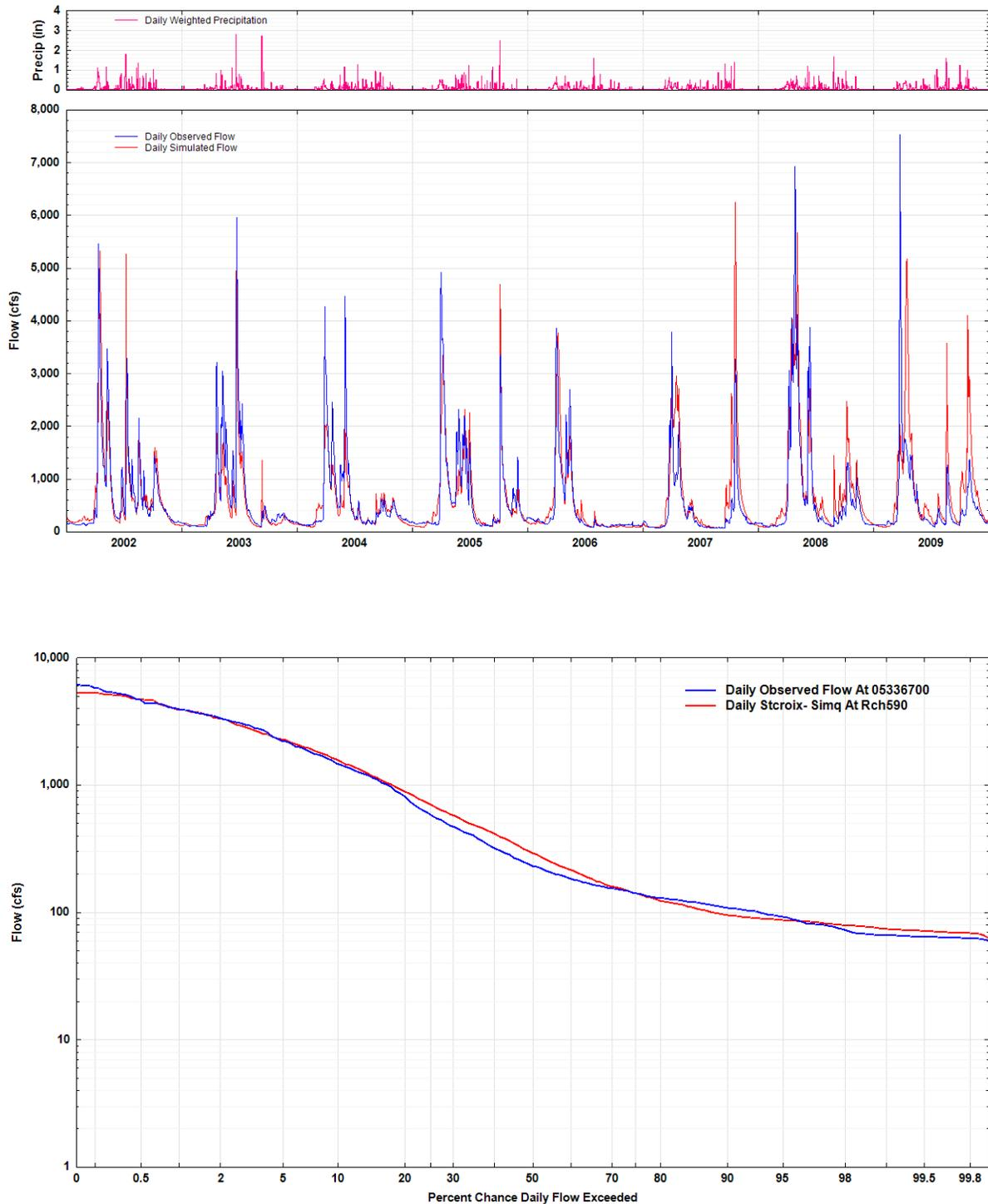
**Figure 2-14.** Observed and Simulated Flow and Flow Frequency Duration Curve at U.S. Geological Survey Gage 05336700 in the Kettle River Watershed for the Calibration Period.
