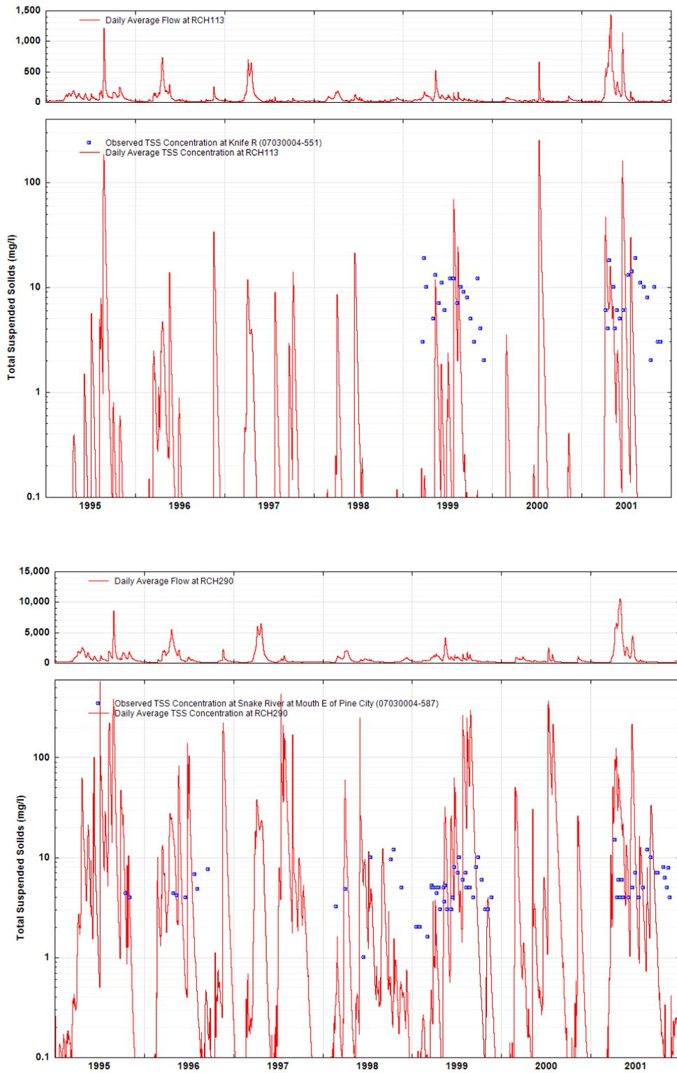
**Figure 3-5.** Observed and Simulated Total Suspended Solids Concentrations in Snake River Watershed at (a) the Knife River and (b) the Snake River Near the Outlet for the Validation Period.
