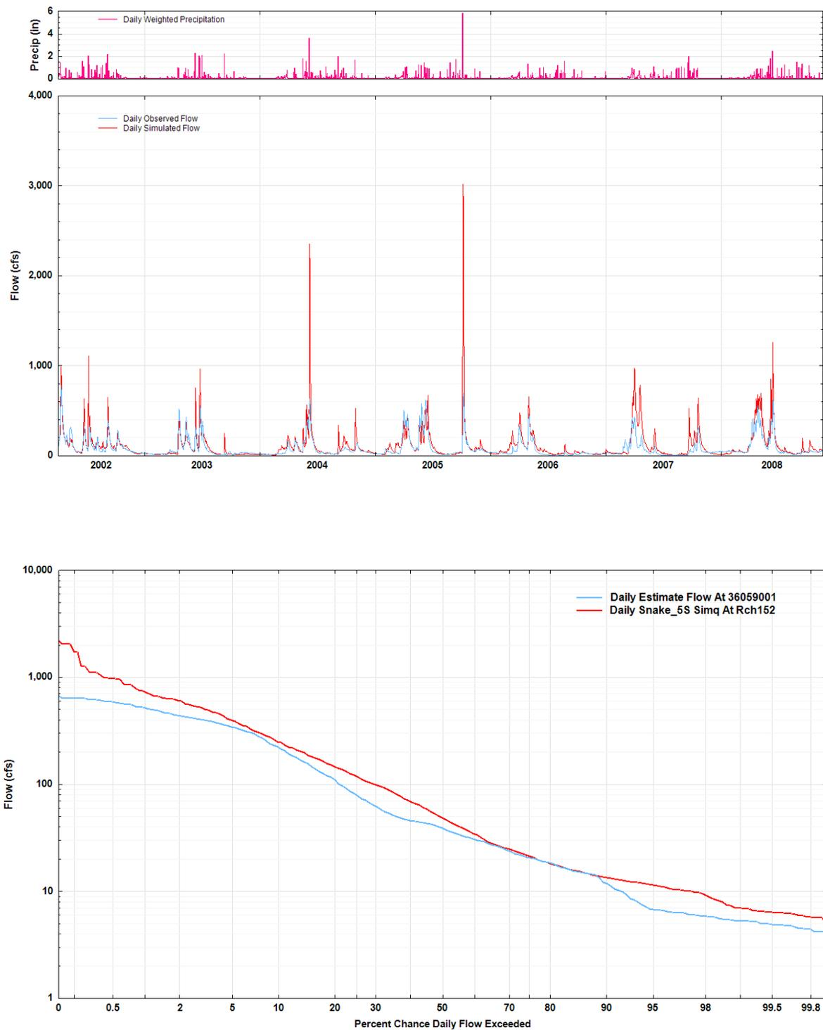
**Figure 2-10.** Observed and Simulated Flow Hydrograph and Frequency-Duration Curve at the Minnesota Pollution Control Agency Gage H36059001.
