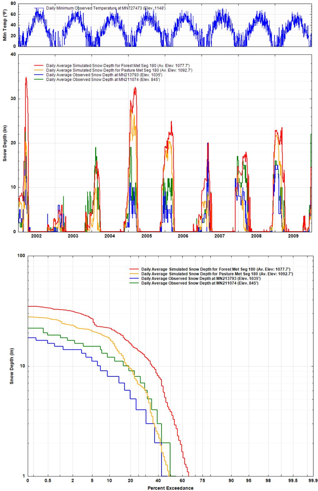
**Figure 2-13.** Simulated Snow Depth and Snow Frequency Compared With Observed Data for Met Segment 180 in the Kettle River Watershed.
