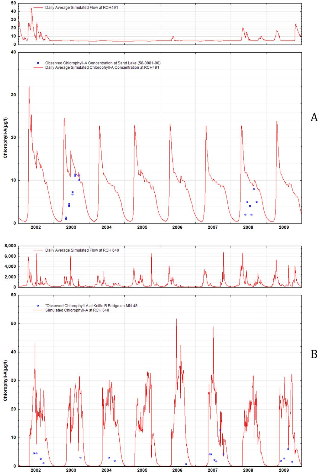
**Figure 4-17.** Observed and Daily Average Simulated Phytoplankton as Chlorophyll *a* at (a) Sand Lake Outlet (RCH491) and (b) Kettle River Bridge on MN-48 Outlet (RCH640).
