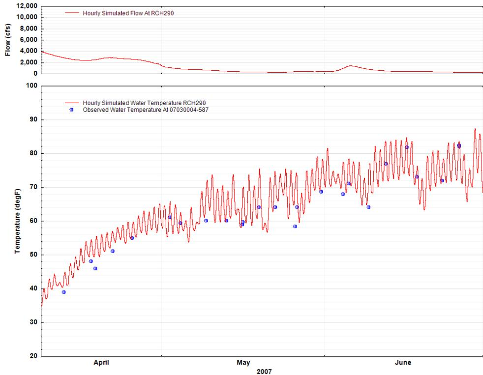
**Figure 4-3.** Observed and Hourly Simulated Water Temperature at Snake River Near Snake River Watershed Outlet (RCH290) for a Small Period.
