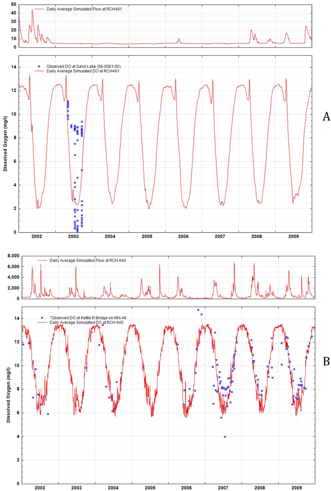
**Figure 4-6.** Observed and Daily Average Simulated Dissolved Oxygen at (a) Sand Lake (RCH491) and (b) Kettle River Bridge on MN-48 (RCH640).
