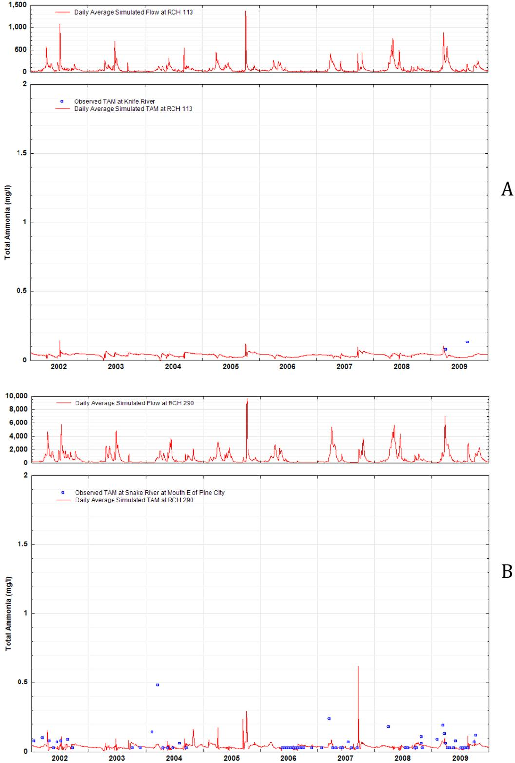
**Figure 4-9.** Observed and Daily Average Simulated Ammonia as Nitrogen at (a) Knife River (RCH113) and (b) Snake River Near the Watershed Outlet (RCH290).
