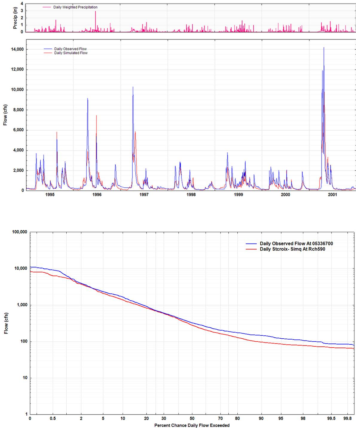
**Figure 2-15.** Observed and Simulated Flow and Flow Frequency Duration Curve at U.S. Geological Survey Gage 05336700 in the Kettle River Watershed for the Validation Period.
