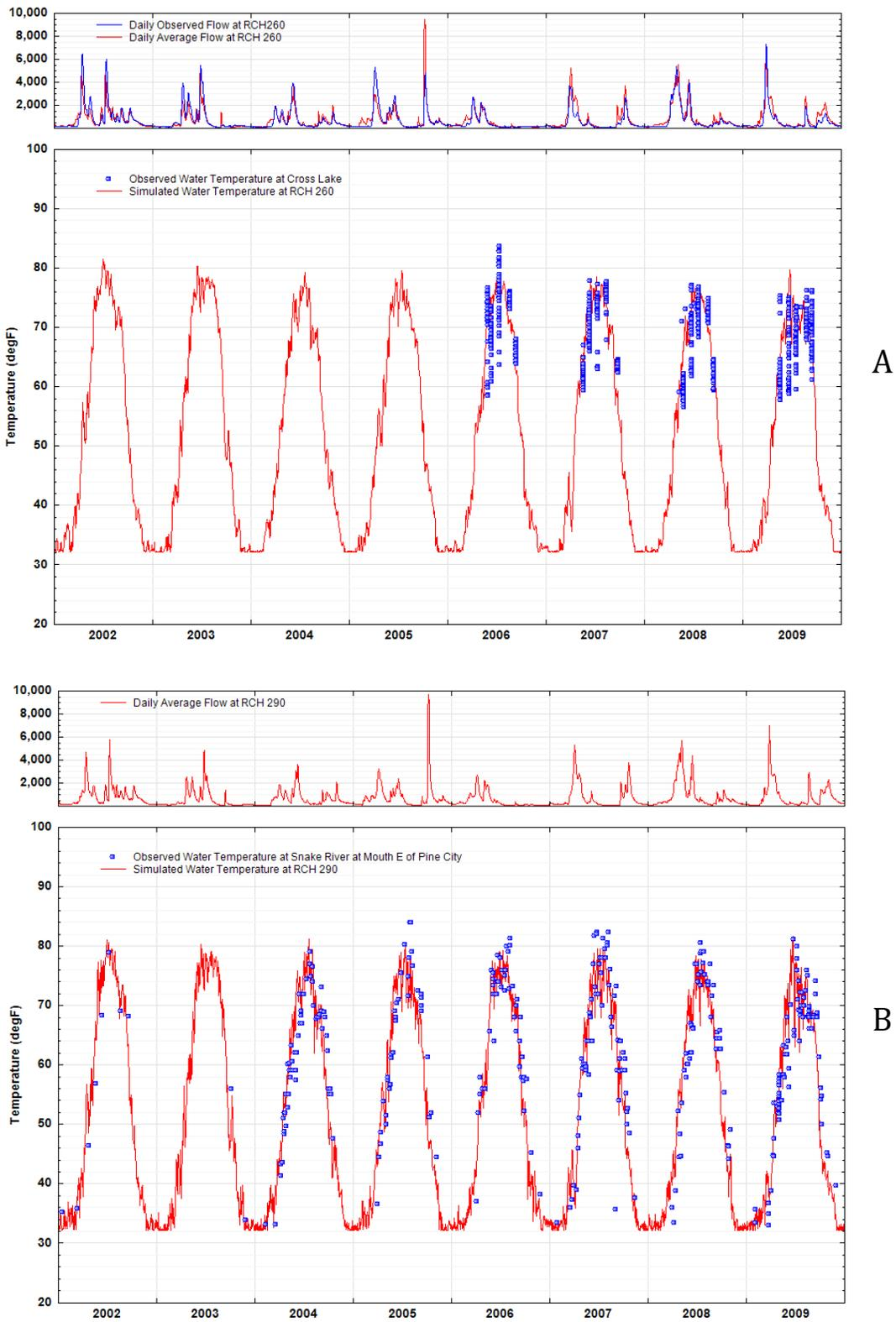
**Figure 4-1.** Observed and Daily Average Simulated Water Temperature at (a) Cross Lake on Snake River (RCH260) and (b) Snake River Watershed Outlet (RCH290).
