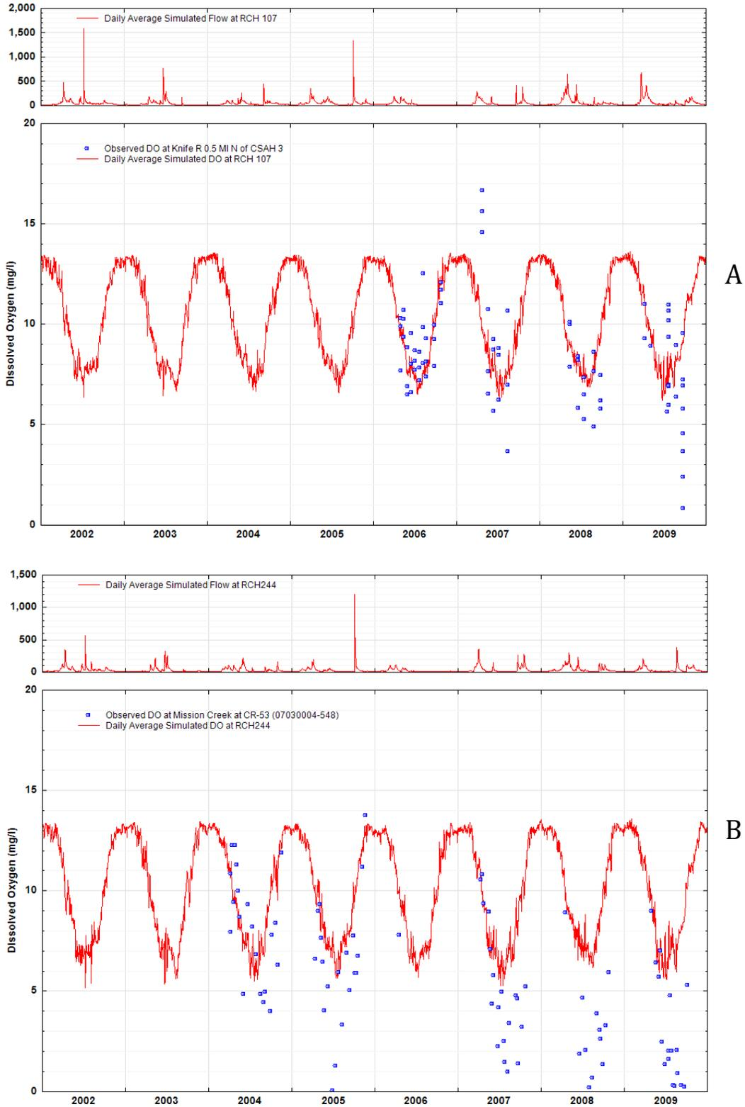
**Figure 4-7.** Observed and Daily Average Simulated Dissolved Oxygen at (a) Knife River (RCH107) and (b) Mission Creek at CR-53 (RCH244).
