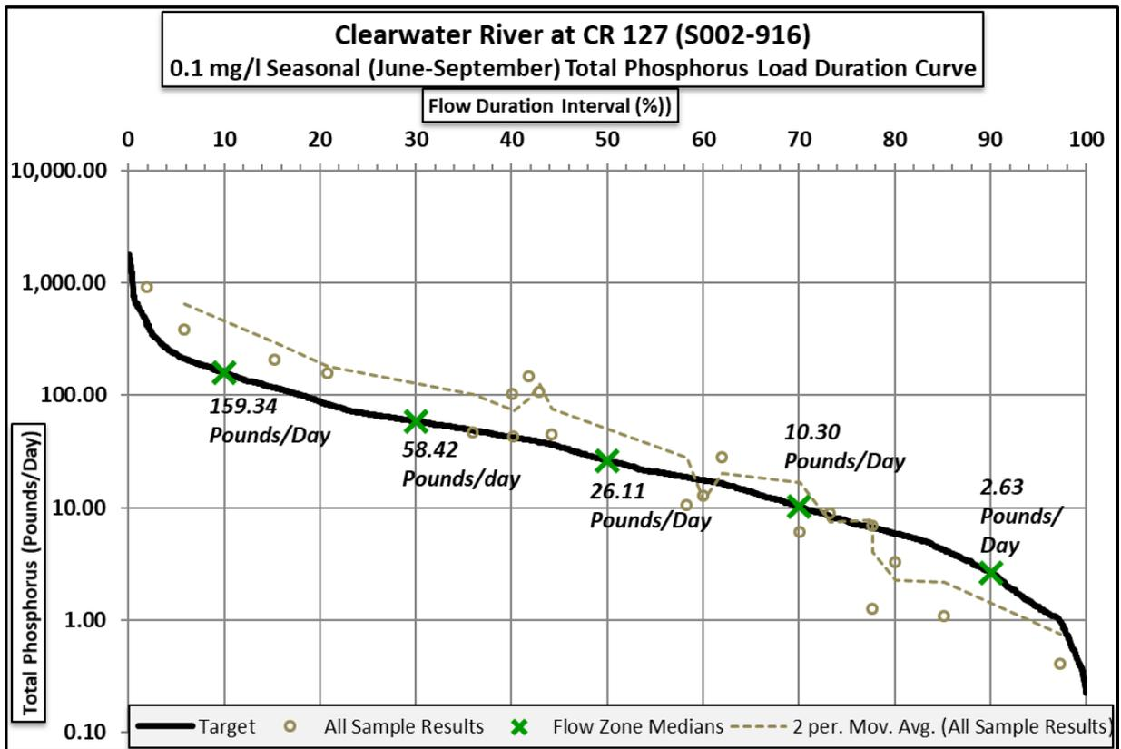
Figure 5-25. Seasonal TP load duration curve and median daily loads for the Clearwater River (AUID 647) at CR 127 (station S002-916)
