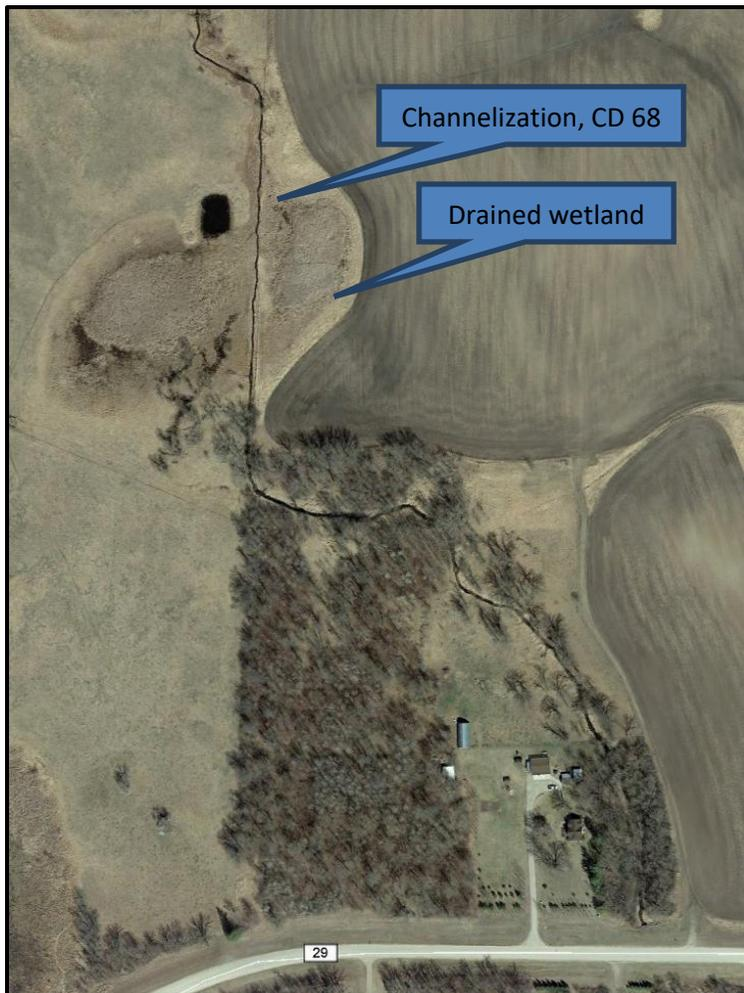
Figure 4-72. Portion of CD 68 (AUID 655), between CSAH 29 and CSAH 3, which was dug through the middle of a wetland
