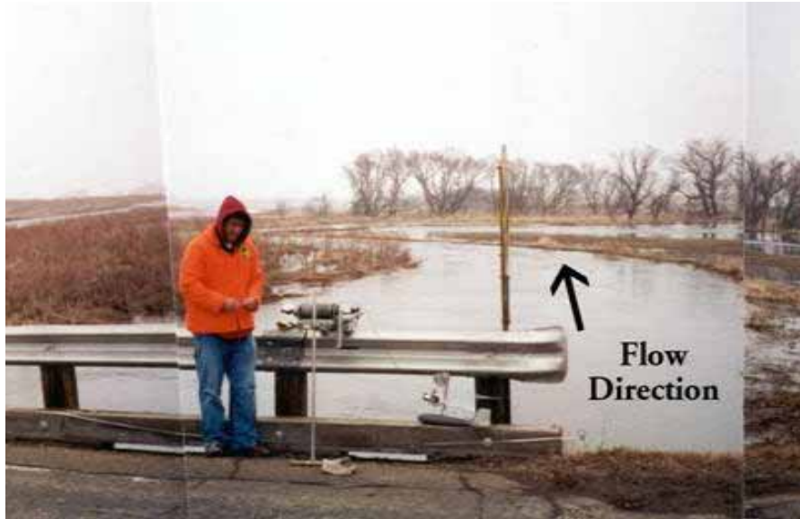
Figure 3: Bridgeboard and Weight being used to determine flow
