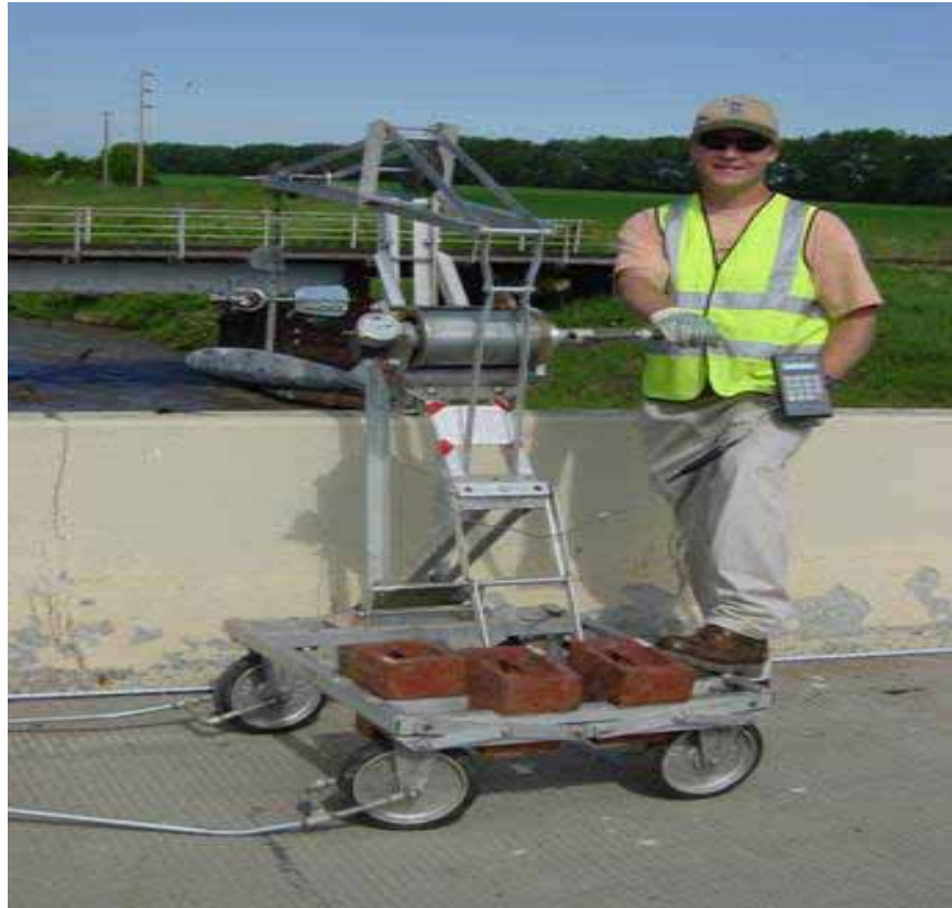
Figure 4: Bridge Crane and Weight used to determine flow
