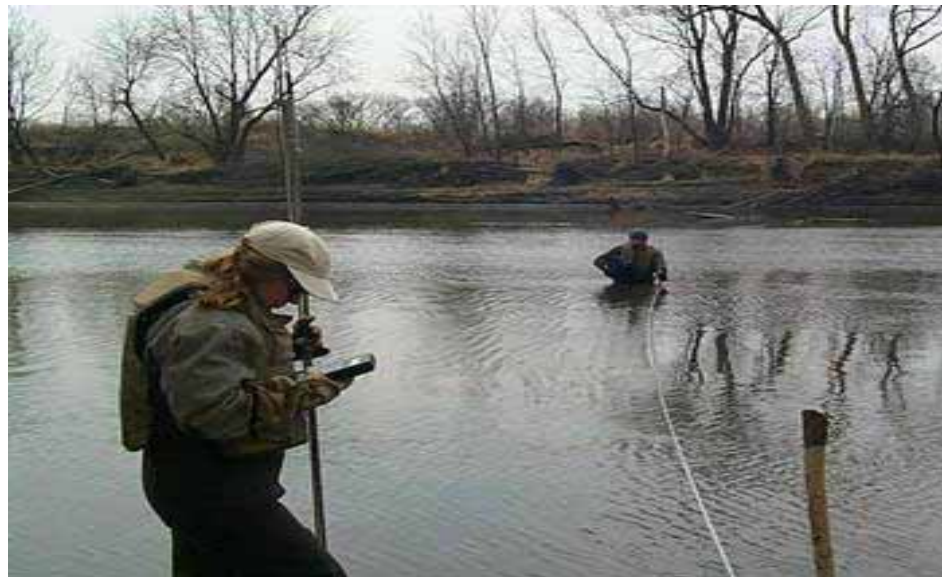
Figure 2: Wading Rod being used to determine flow.
