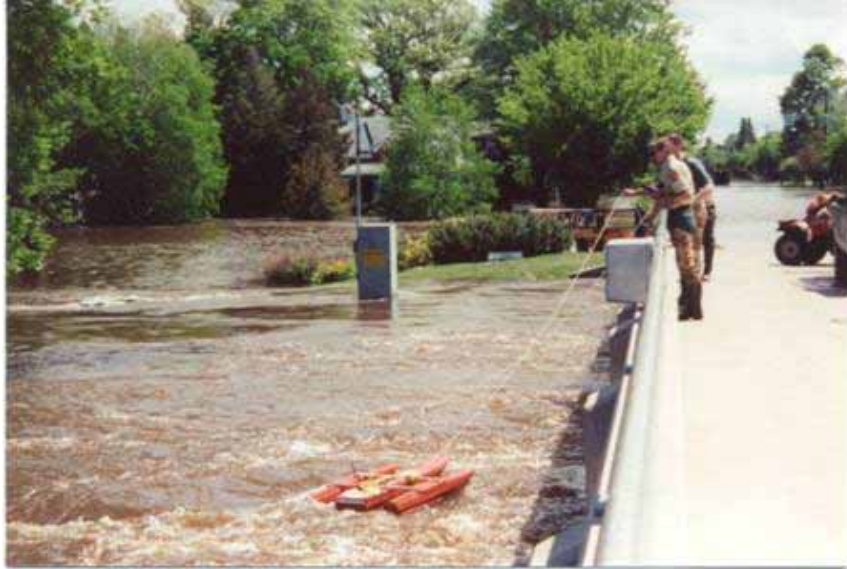
Figure 5: Acoustic Doppler Current Profiler being used to determine flow
