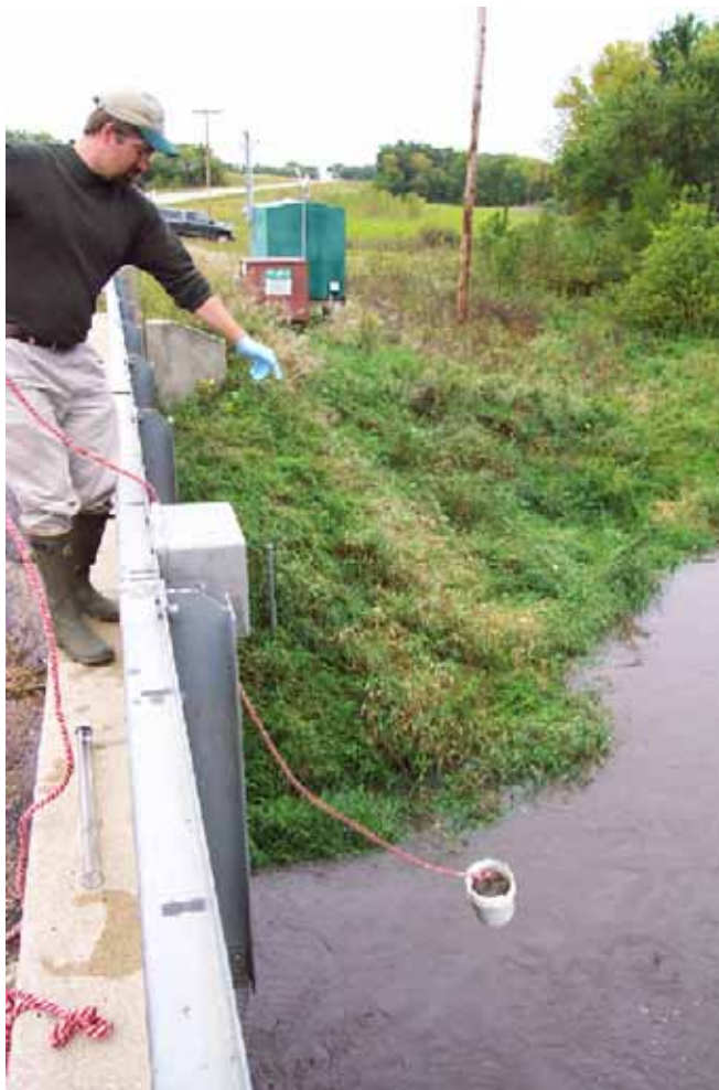
Figure 9: Staff taking a grab sample using a bucket and rope
