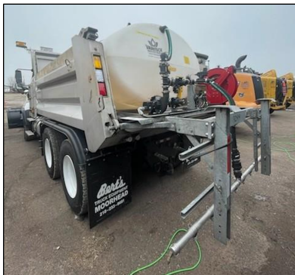
Figure 54. Plow truck with liquid application equipment.
