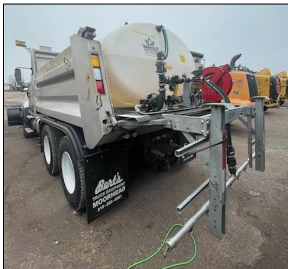
Figure 54. Plow truck with liquid application equipment.
