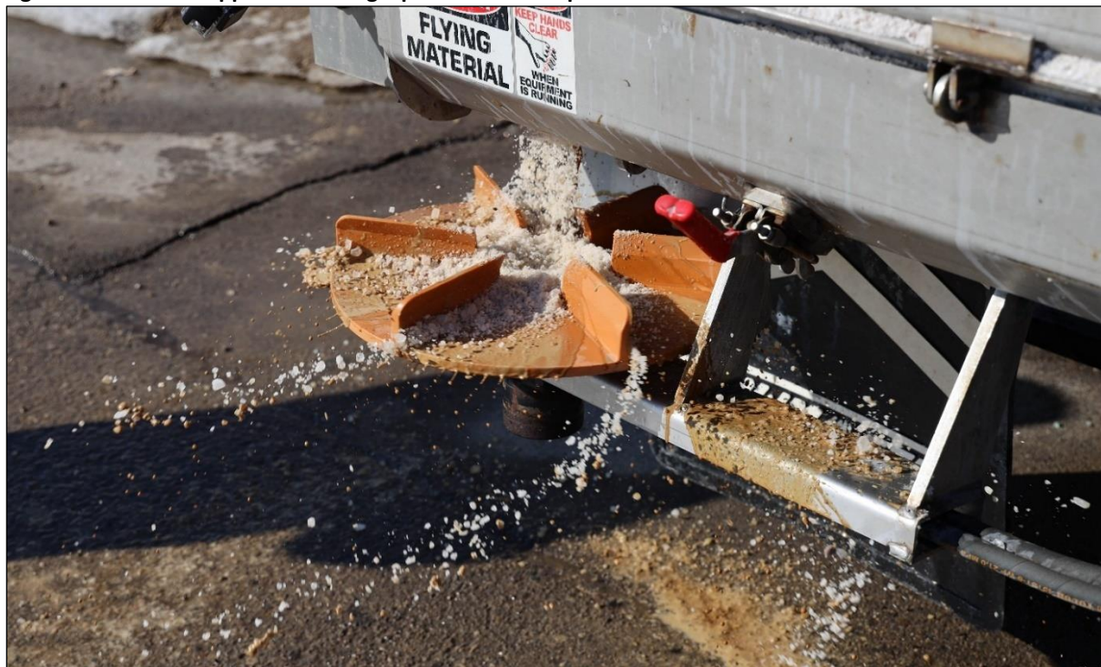
Figure 33. Road salt application using a plow truck and spinner.
