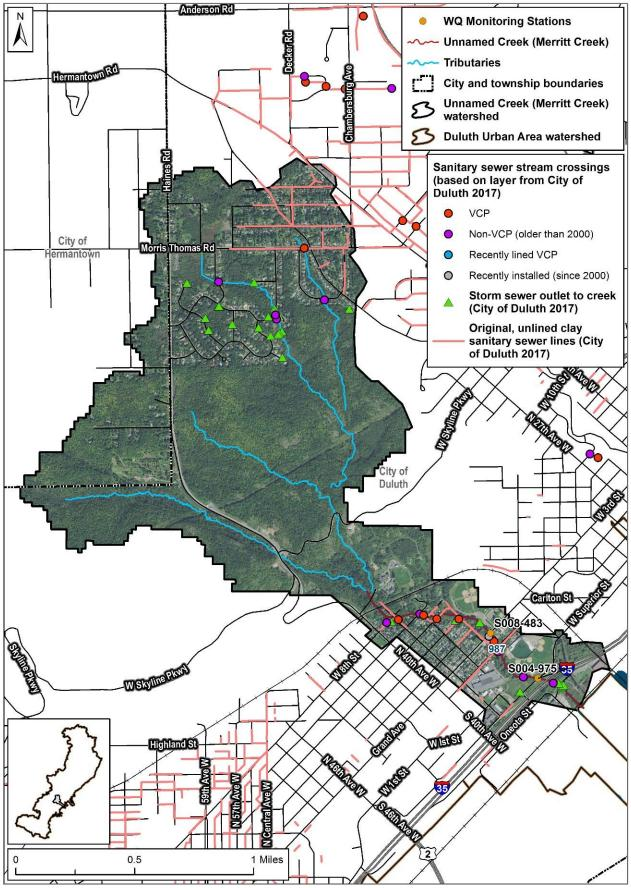
Figure 42. Potential wastewater infrastructure sources of E. coli in Merritt Creek.
