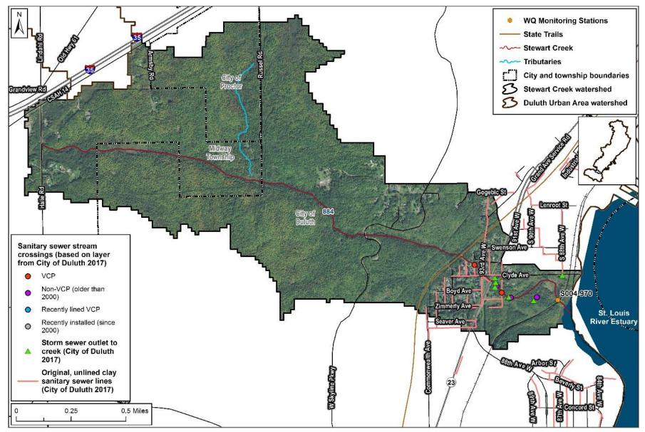
Figure 41. Potential wastewater infrastructure sources of *E. coli* in Stewart Creek.
