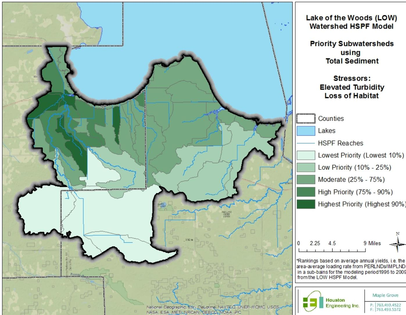
Figure 17: Tributary scale subwatershed priority for implementation for the stressors elevated turbidity and loss of habitat for LOWW using average (1996-2009) annual total sediment yields.
