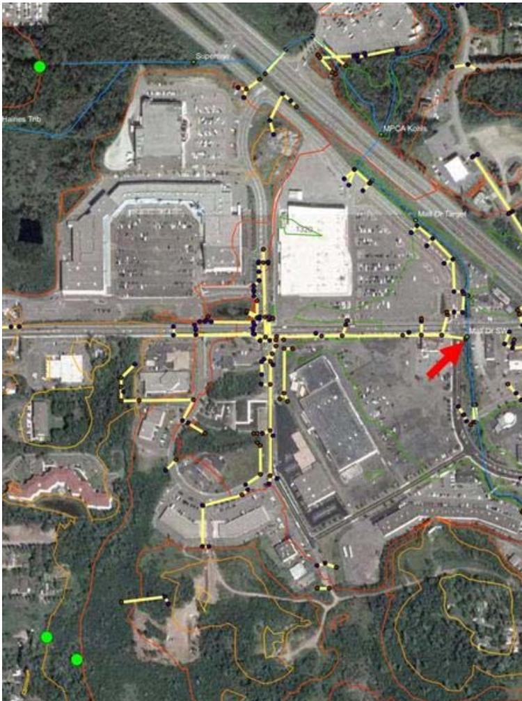
Figure 2.1. Commercial sub-watershed at Maple Grove Rd. The red arrow shows the drainage inlet to Miller Creek and the light-colored lines between black dots show the drainage system.
