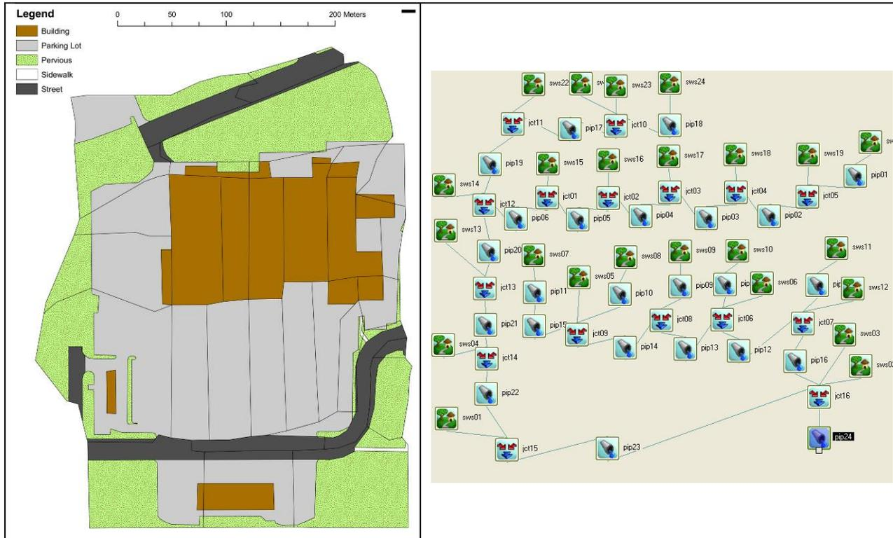
Figure A1.1. Diagram of the 24 sub-watersheds used to represent the 31.4 acre Wal-mart facility (left) and parking lot, and the corresponding MINUHET schematic (right).
