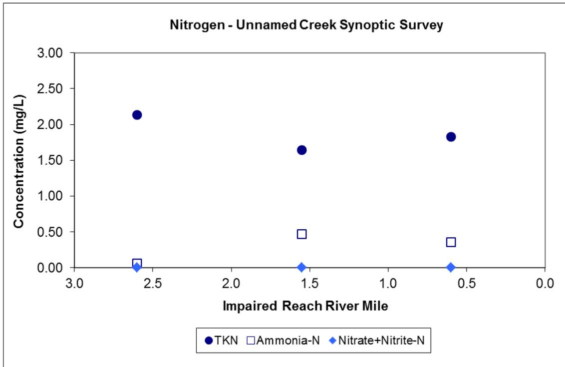
Figure 1-6. Main-stem synoptic survey nitrogen sampling results.
