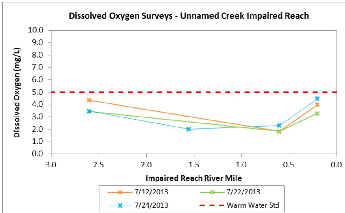
Figure 1-10. Unnamed Creek DO longitudinal profiles measured before and during the July 2013 synoptic survey.
