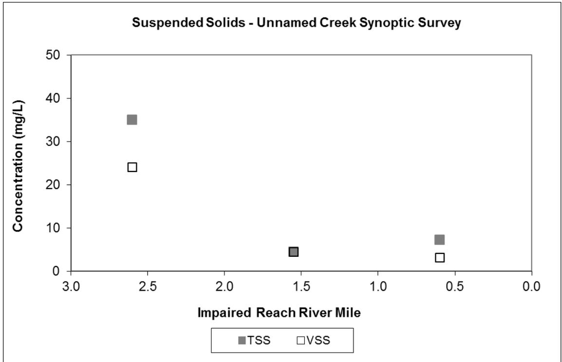
Figure 1-9. Main-stem synoptic survey suspended solids sampling results.
