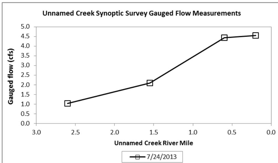
Figure 1-4. Gauged flow measurements during the July 24 synoptic survey.
