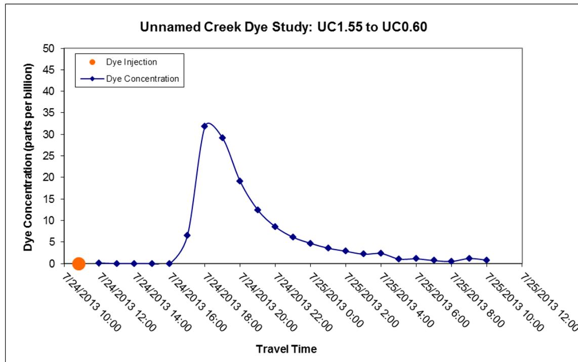
**Figure 1-2. UC1.55 to UC0.60 dye study measurements.**
