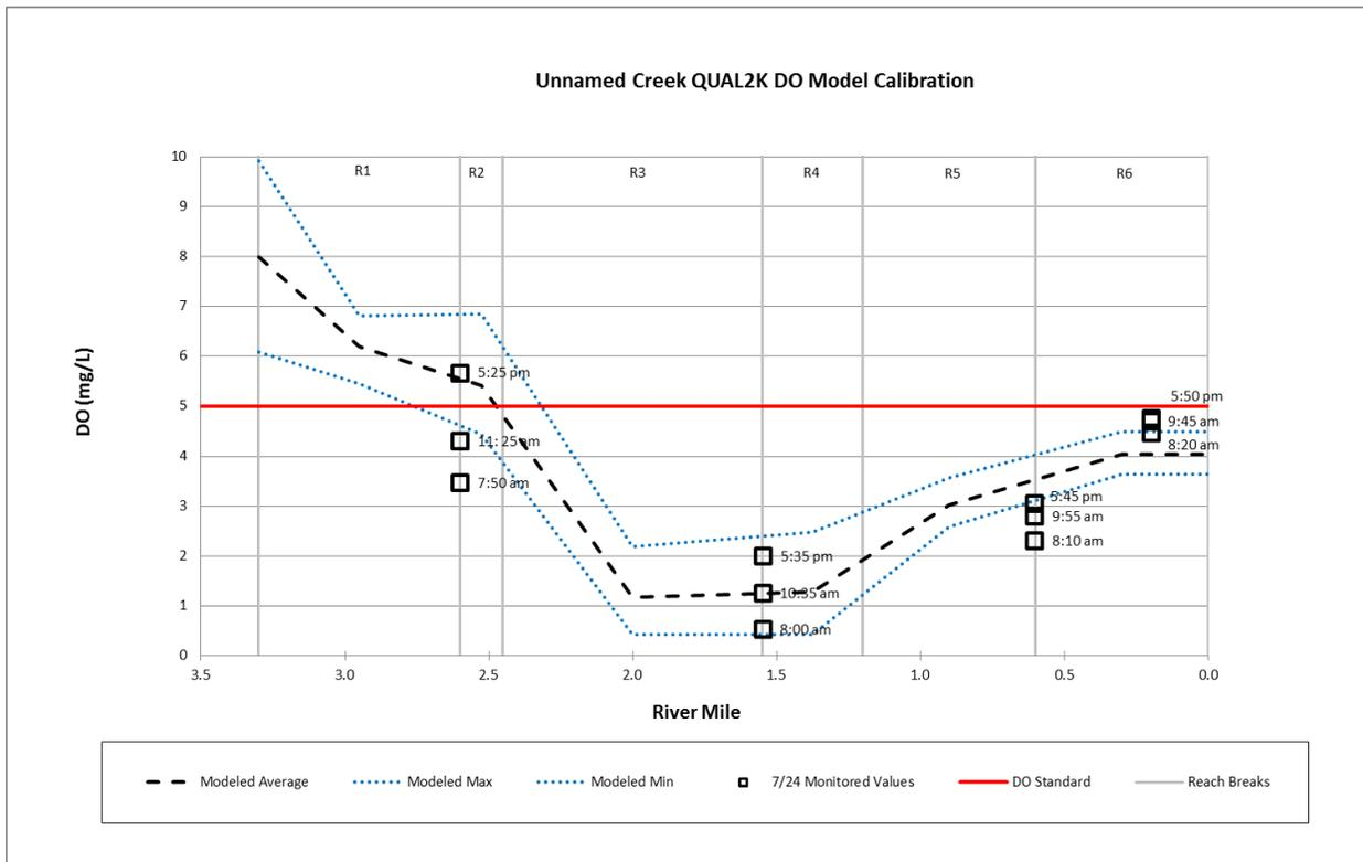
Figure 1.4. DO longitudinal profile for the Unnamed Creek QUAL2K calibrated model run.
