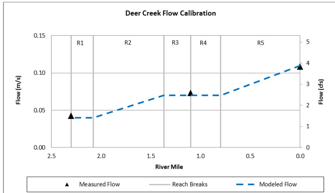
**Figure 1.2. Deer Creek QUAL2K flow calibration with headwater, tributary and groundwater diffuse inflows.**
