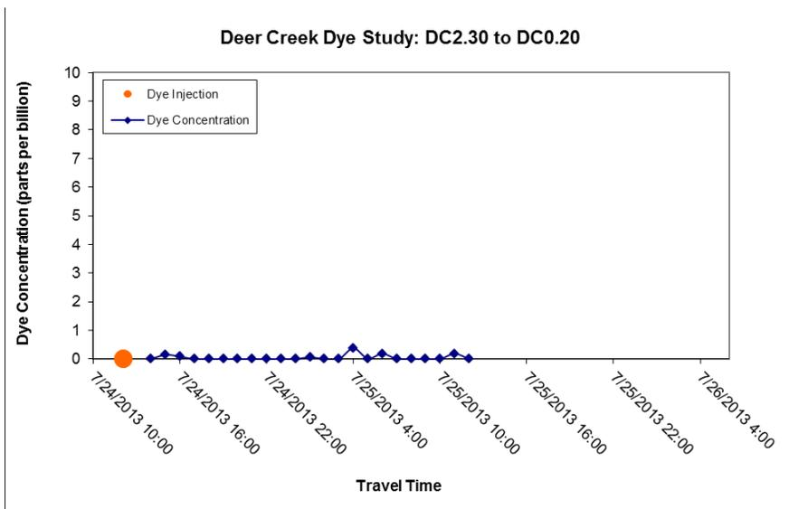
Figure 1-4. Sub-reach 2 dye study measurements.
