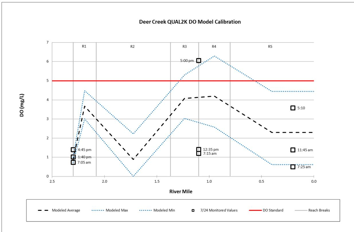
**Figure 1.4. DO longitudinal profile for the Deer Creek QUAL2K calibrated model run.**
