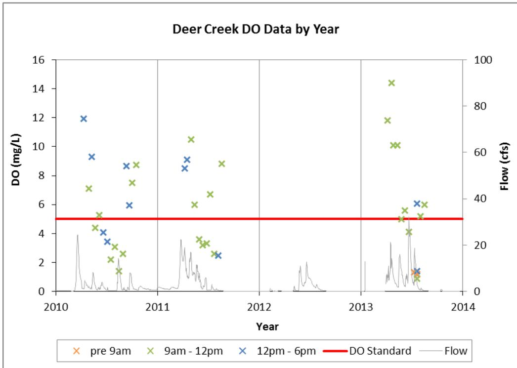
**Figure 2-1. DO and flow data for the Deer Creek impaired reach by year, color coded by time of day.**
