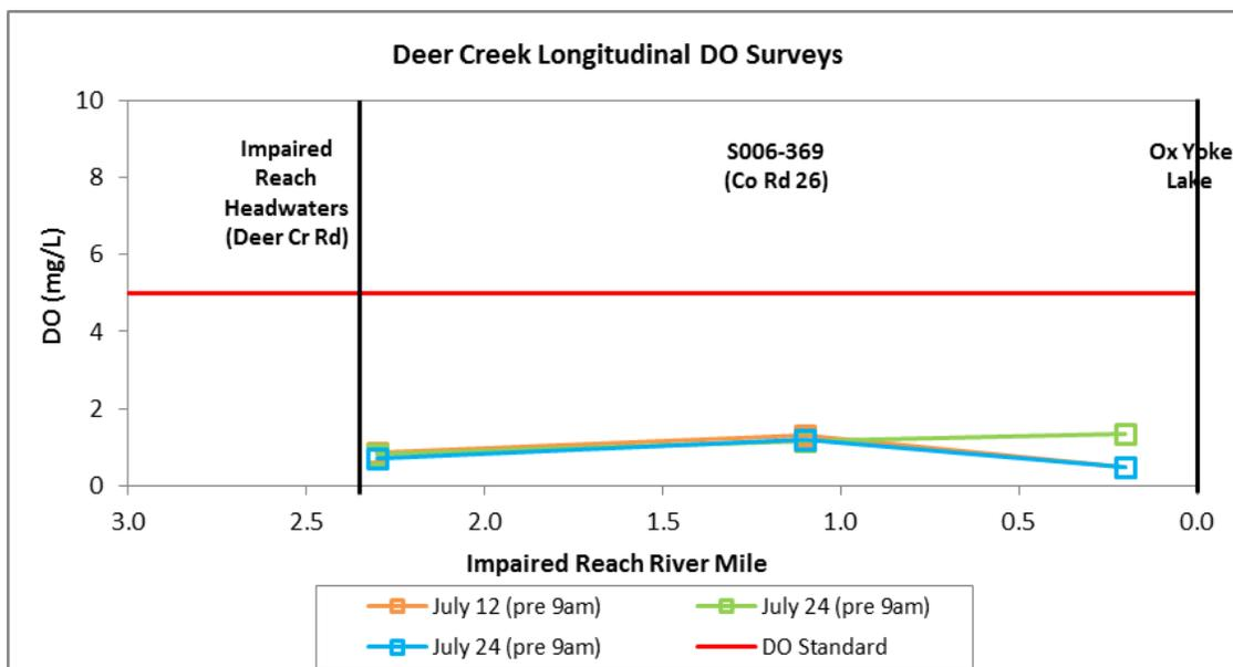
Figure 1-12. Deer Creek early morning DO longitudinal profiles measured before and during the July 2013 synoptic survey.
