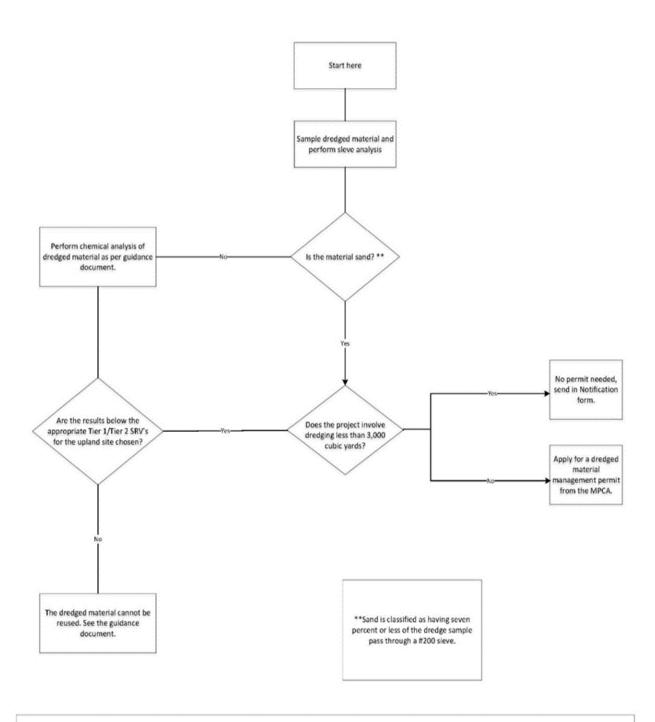
Note: If dredge material is proposed to go to a permitted landfill, disregard the process listed below. A permit for the management of dredged material is not required.
