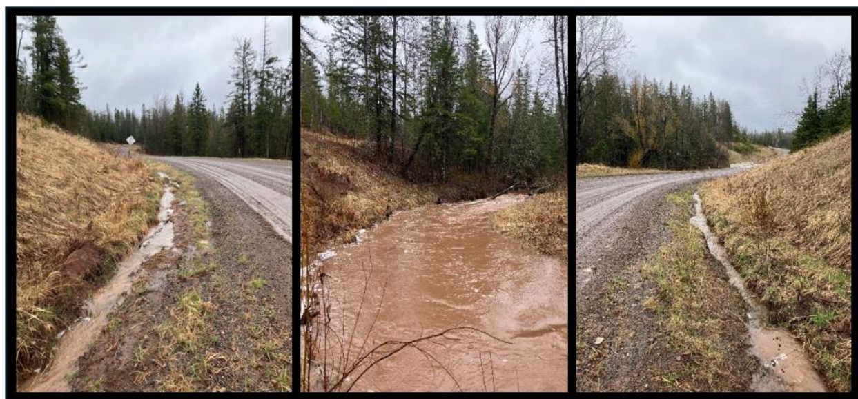
Figure 19. Observed clarity at Right: north ditch to Skunk Creek at CR103 crossing, Middle: Skunk Creek upstream of the CR103 crossing, and Left: south ditch to Skunk Creek at CR103 crossing.
