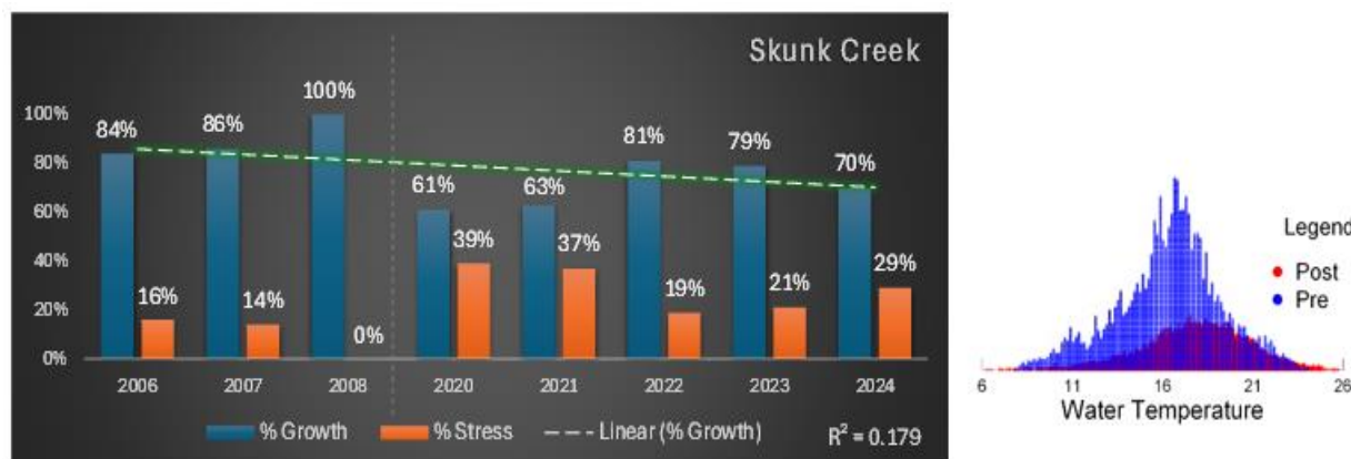
Figure 12. Skunk Creek thermal stats (% Growth and % Stress) for data years between 2006 and 2024 (Left) and density plot (Right) for the same period in the stream reach that extends from Skunk at CR103 site H05013005 downstream to Skunk ds restoration site H05013003.
