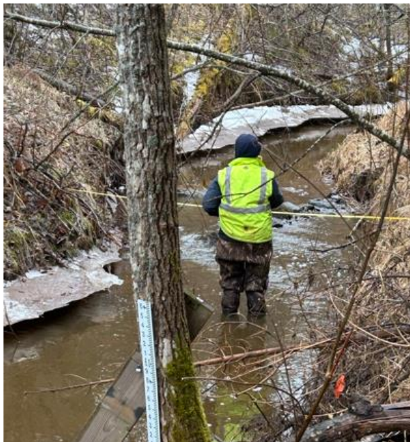
Figure 6. The MPCA measuring streamflow at Elim at outlet gage (H05013004).
