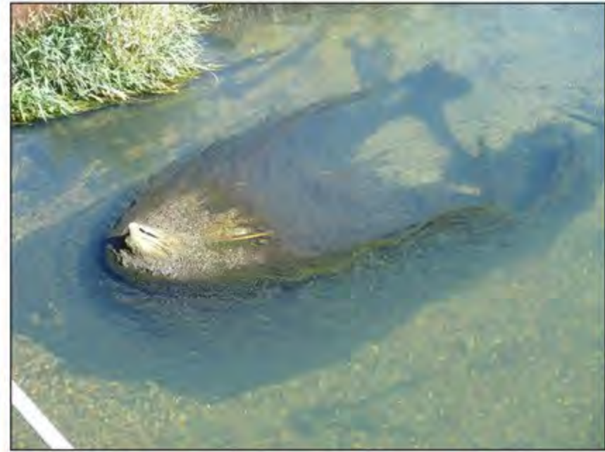
Figure 14. Filamentous algal growth on a vertical pipe, part of stream gaging equipment at 2016.
