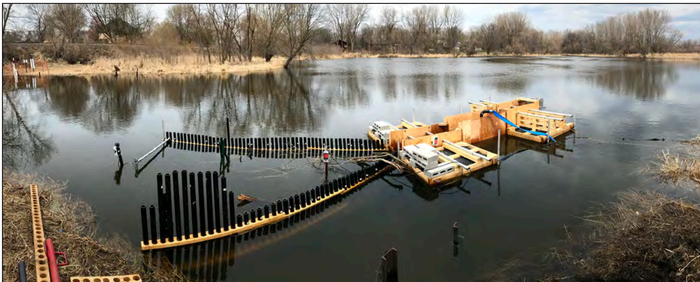
The Rice Creek Watershed District is testing a low-voltage electrical guidance system that directs migrating carp into a gate that leads to a fish ladder. Paired with a Whooshh System (AKA carp cannon), not yet attached, it is designed to remove about 75 percent of migrating carp. Carp removal is one part of RCWD's $7.3 million plan to improve water quality in Long Lake.
