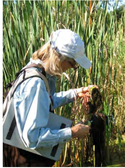
Figure 4. Handheld garden cultivator used for shoreline sampling (left) tied to a 20' length of rope with a loop tied on the end to prevent losing the cultivator. The tines are bent backwards to increase grip on aquatic vegetation. The cultivator is tossed and retrieved (above left) three times at each sampling station and aquatic rapid species are identified (above right).
