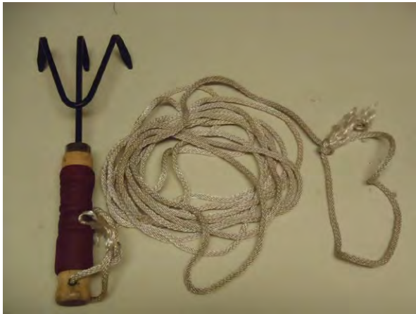
Figure 4. Handheld garden cultivator used for shoreline sampling (left) tied to a 20' length of rope with a loop tied on the end to prevent losing the cultivator. The tines are bent backwards to increase grip on aquatic vegetation. The cultivator is tossed and retrieved (above left) three times at each sampling station and aquatic rapid species are identified (above right).
