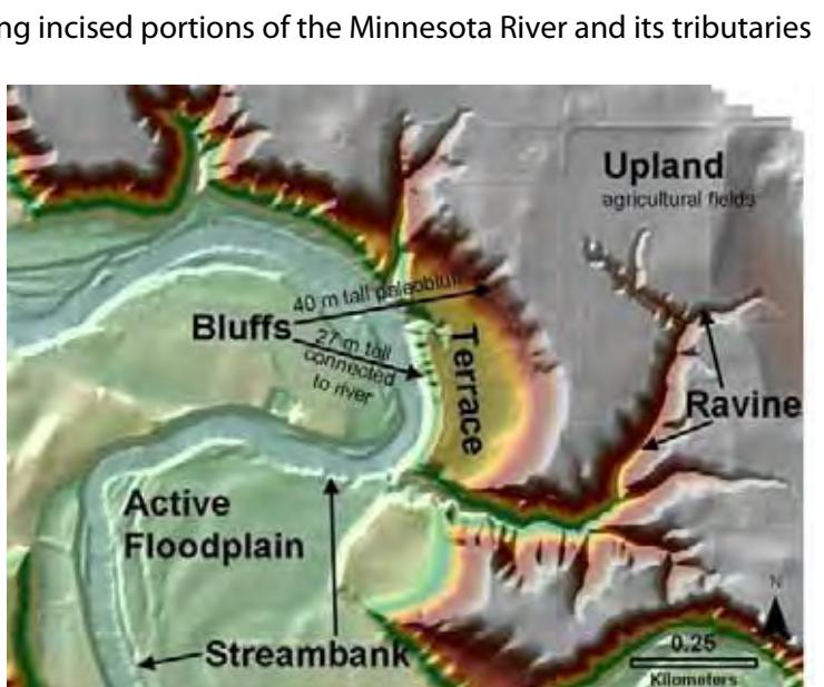
**Figure 5. Digital elevation model of a portion of the Le Sueur River watershed, showing the primary sources of sediment.**
