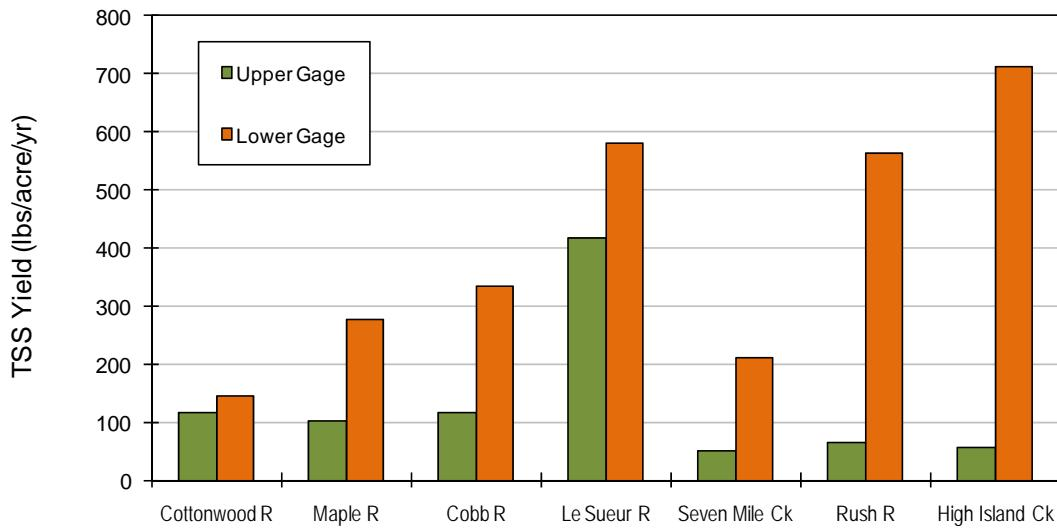
**Figure 8. Annual TSS yield at upper and lower gauges in seven watersheds tributary to the Minnesota River. The gauges are located above and below the incised lower portions of the river valleys. Increases in TSS yield are generally much larger than the corresponding increase in drainage area, indicating that disproportionately large amounts of sediment are supplied in the incised reaches between each pair of gauges.**
