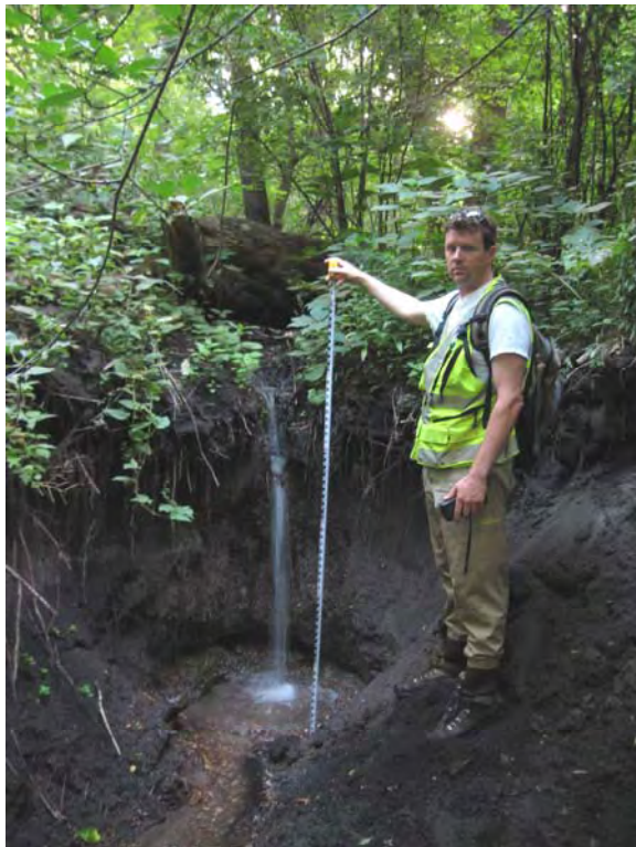
Figure 2: A headcut and incised channel on Tributary 1 of the Credit River.
